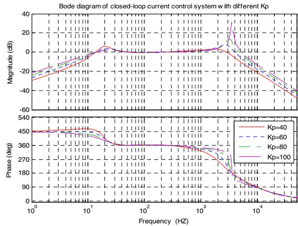
Fig. 6 Bode diagram of closed-loop current control system--  $G_{ref_c}(s)$  Parameters:  $K_r=5000$ ,  $\omega_c=5$ ;
