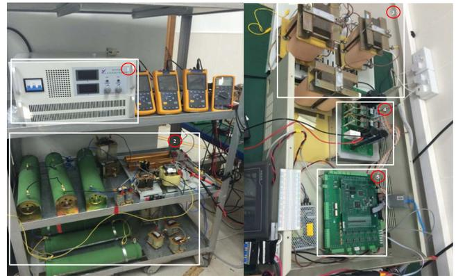
Fig. 12 Experimental Prototype (Note: ①-DC power supply; ②-Loads; ③-Coupling impedance; ④-IGBT and drivers; ⑤-Control board and signal conditional circuit.)
