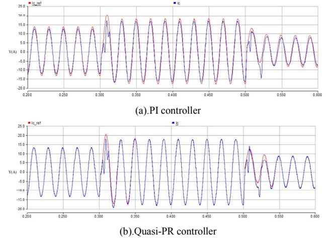
Fig. 9 Current waveforms when load (linear load) changes
