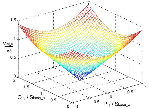
Fig. 2 Variation in inverter voltage with power
