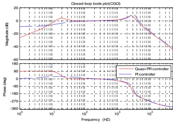
Fig. 7 Bode diagram of closed-loop transfer function  $G_{ref_c}(s)$  (solid line: use
