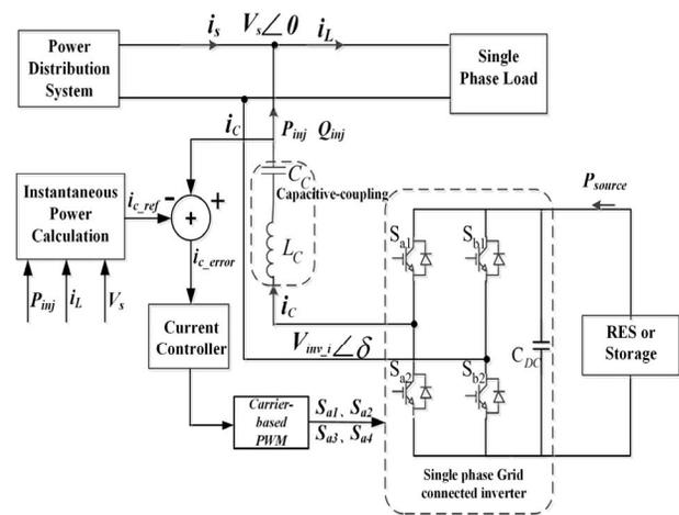
Fig. 1 System configuration of a single-phase CGCI
