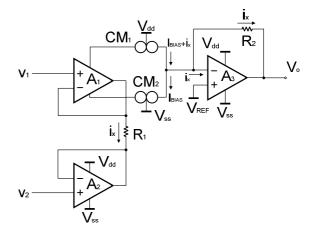
Fig. 1. Current mode instrumentation amplifier topology using op amp power supply current sensing technique.
