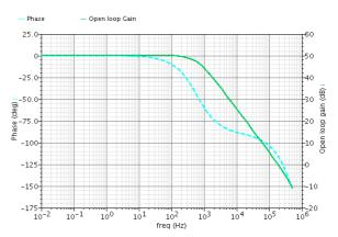
Fig. 2. Frequency response of input op amp.
