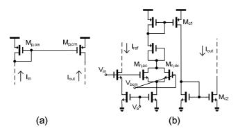
Fig. 4. Current Mirrors. (a) Schematic of CM1. (b) Schematic of CM2.
