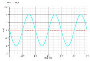
Fig. 6. Transient response to a 2m V<sub>pp</sub> input differential voltage.
