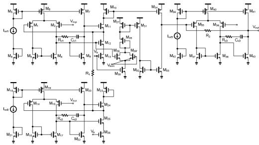
Fig. 3. Completed schematic of proposed CMIA
