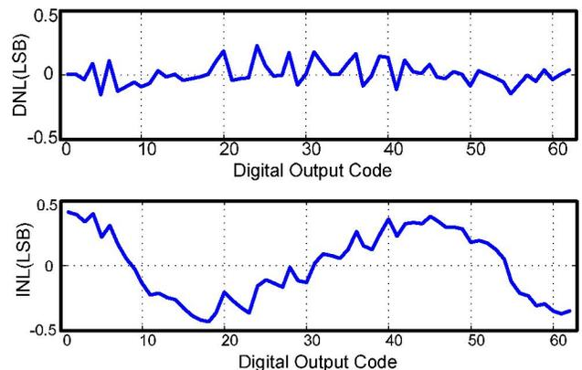
Fig. 6: Simulated DNL and INL of 6-bit ADC
