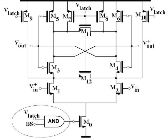
Fig. 5: High speed comparator and its switching circuit
