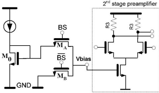
Fig. 3: Switchable biasing circuit for 2<sup>nd</sup> gain stage
