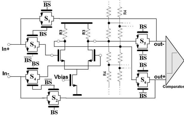
Fig. 4: Switching circuit between two resolution modes
