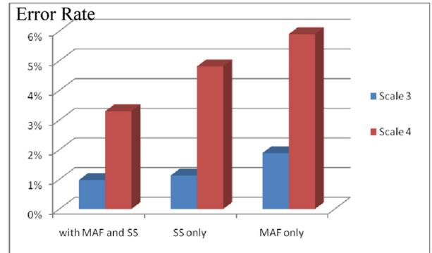
Fig. 4. Error rate of different system architecture evaluate by using MITBIH arrhythmia database; MAF stands for moving average filtering, SS stands for signed squaring.
