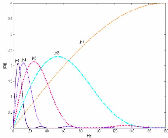
Fig. 2. The amplitude-frequency responses of equivalent filter  $Q_j(\omega)$  at different scales corresponding to 360 Hz sampling frequency;  $f=180\omega/\pi$ .
