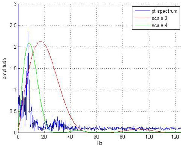
Fig. 3. The amplitude-frequency responses of equivalent filter  $Q_j(\omega)$  at scale 3 and 4 corresponding to 250 Hz sampling frequency; and spectrum of P and T wave of a typical ECG signal obtain from record "sel123" of MITBIH QT database.
