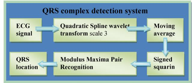
Fig. 1. System architecture of the proposed system.
