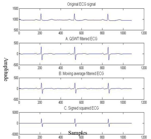
Fig. 3. Test with ECG signal from MIT/BIH Arrhythmia database record 102.
