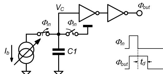
Figure 1: Traditional current-controlled delay generator.
