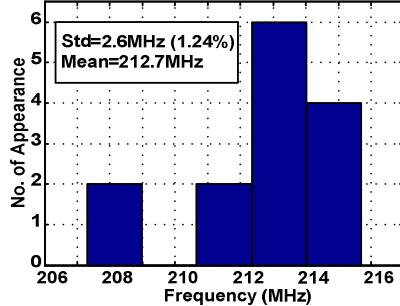
Figure 8: Statistics of measured oscillator frequency of 14 samples at  $I_b=40\mu\text{A}$ .
