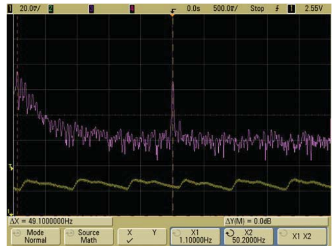
Fig. 5 Acquired Electric pulsation of the plethysmography from sensor (Yellow colour: Time domain & its FFT in purple colour)
