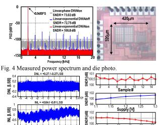
Fig. 5 Measured 17b DNL/INL, and SNDR vs. samples,  $V_{DD}$  & temp. Table I Performance summary and comparison with the state-of-
