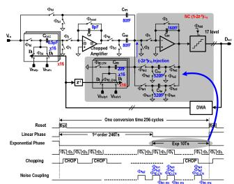
Fig. 3 Circuit diagram of the linear-exponential incremental
