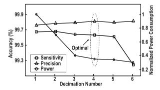
Fig. 4. Detection accuracy and normalized power consumption in different sampling rates.
