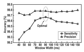
Fig. 6. Detection accuracy versus different window widths.
