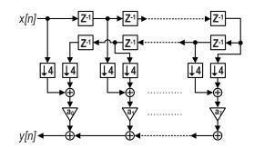
Fig. 5. Implementation architecture of the proposed DQSWT.
