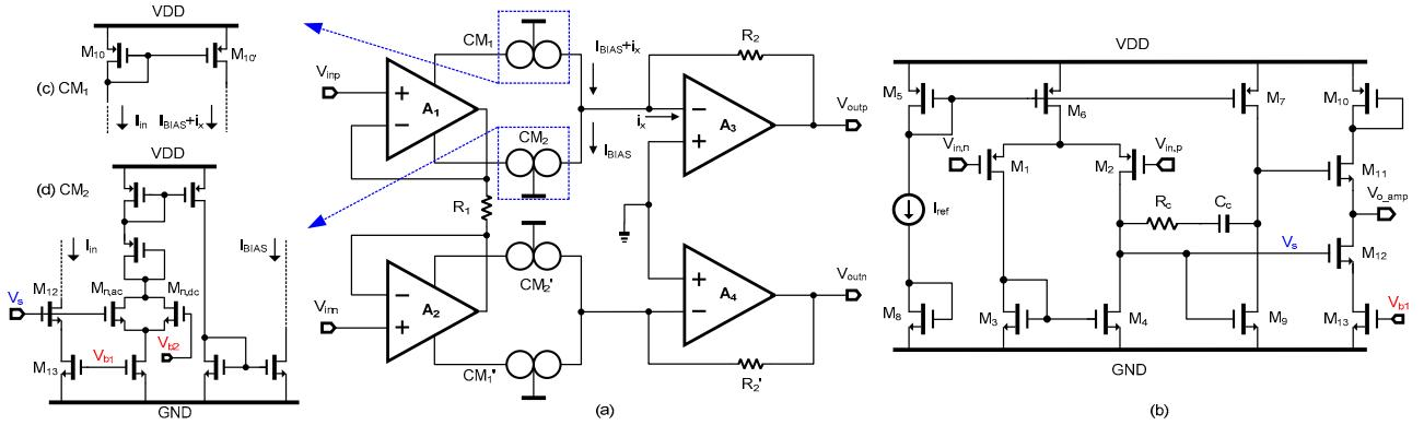
Fig. 2. (a) Current-conveyor-based CMIA. (b) Schematic of the OpAmp. (c) The Current mirror CM<sub>1</sub>. (d) The Current mirror CM<sub>2</sub>.
