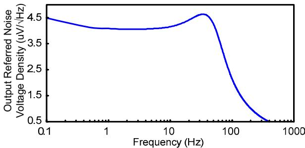
Fig. 10. LPF's output-referred noise voltage density.
