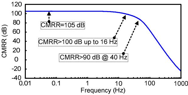
Fig. 8. CMRR of the entire readout front-end.
