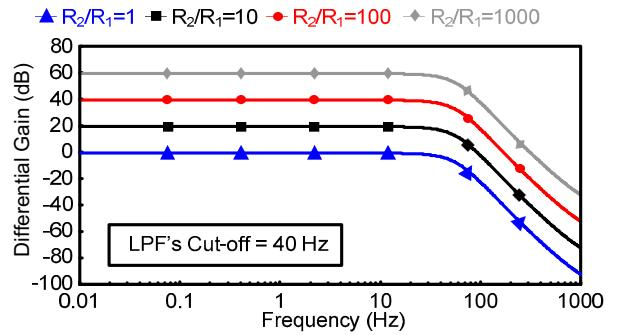
Fig. 7. Frequency response of the CMIA with 40-Hz LPF's cutoff.
