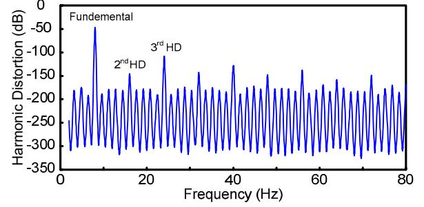
Fig. 6. Harmonic distortion with 5-mV<sub>pp</sub> input @ 8Hz. The gain is set to 10 V/V; corresponding to a 50-mV<sub>pp</sub> input at the LPF.
