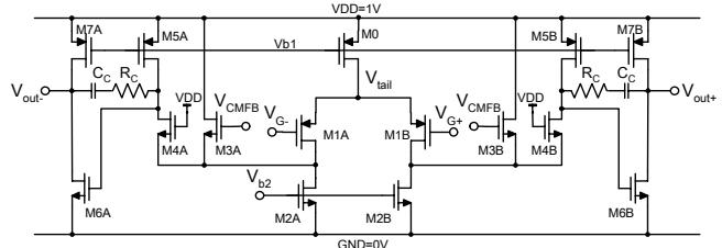
Fig. 4: The low-voltage two-stage fully-differential opamp.
