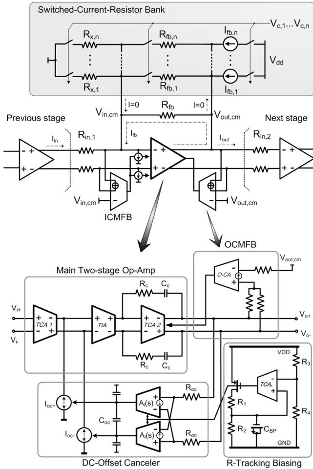
**Fig. 7 Gain-programmable amplifier with offset-canceler embedded op-amp.**
