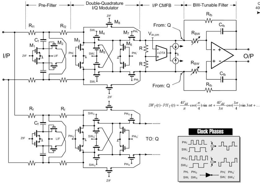
Fig. 5 Pre-filter, double-quadrature I/Q modulator and BW-tunable filter.
