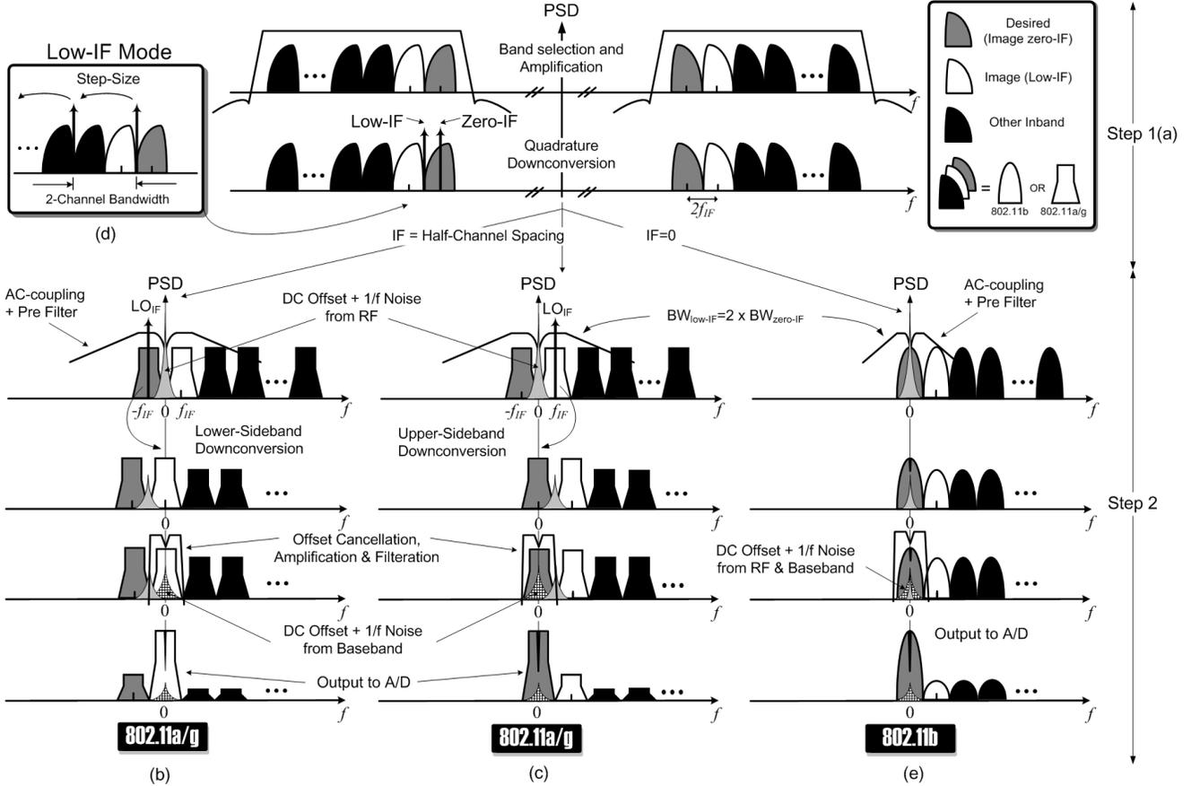
**Fig. 4 Spectra-flow illustrations. (a) Step-1: RF-to-IF downconversion for 802.11a/b/g. (b) Step-2: IF-to-baseband lower-sideband downconversion. (c) Step-2: IF-to-baseband upper-sideband downconversion. (d) Low-IF channel-selection scenario at RF. (e) Step-2: zero-IF mode.**
