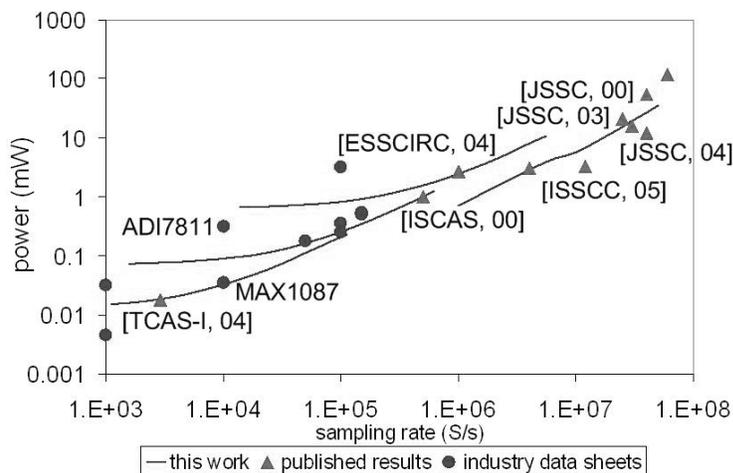
From "A 50MS/s (35mW) to 1KS/s (15É W) Power Scaleable 10b Pipelined ADC with Minimal Bias Current Variation," by Imran Ahmed and David Johns - Univ. of Toronto, Toronto, ON. Canada, providing a comparison of their results with industry data sheets.
