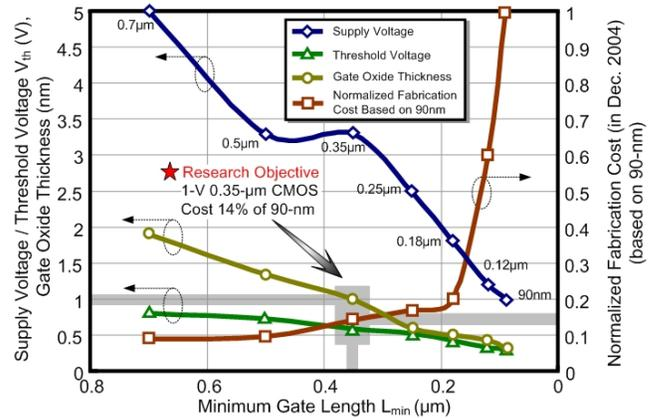
Fig. 1 Roadmap of CMOS scaling and the research objective.
