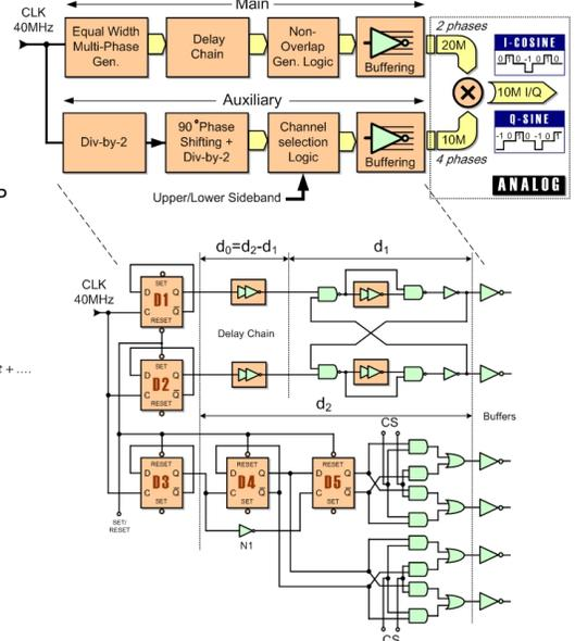
Fig. 6 Mixed-signal clock generator.
