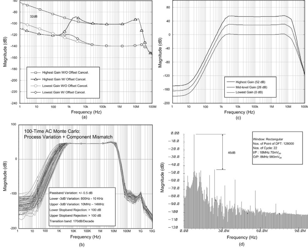
**Fig. 9 Post-layout simulation results. (a) Output noise (zero-IF). (b) AC response (zero-IF). (c) Monte-Carlo AC responses (zero-IF). (d) FFT response (low-IF).**
