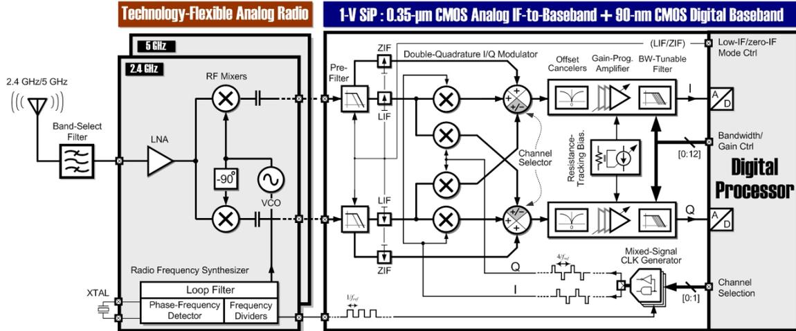
Fig. 2 Receiver architecture.
