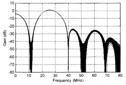
Fig.5 Monte-Carlo amplitude response simulations ( $\sigma_e = 0.7$  %)
