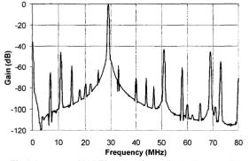
Fig.6 Spectrum of 29 MHz output signal with 1.5Vp-p 11 MHz sinusoidal input from the worst-case transistor-level simulation
