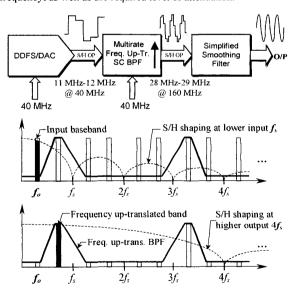
Fig.1 Frequency up-translated bandpass filtering for DDFS systems
