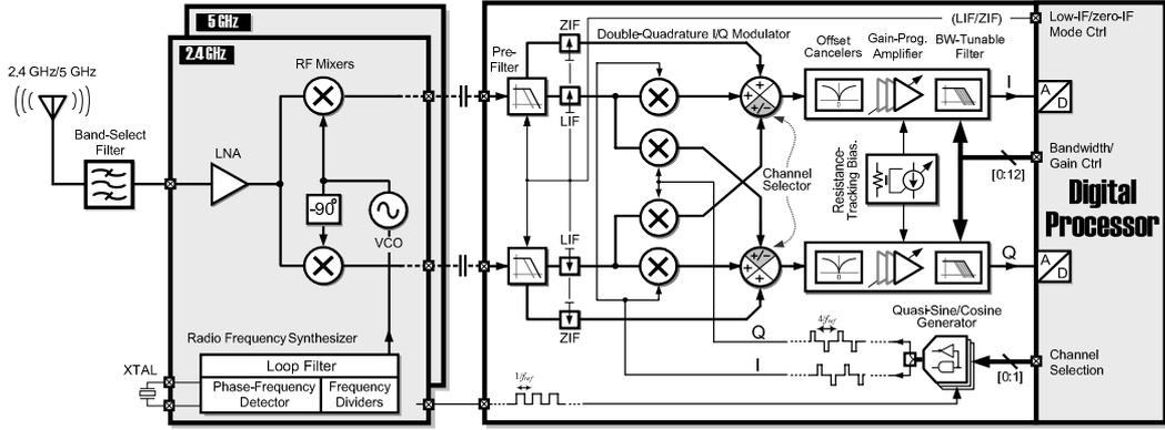
Fig. 2: Proposed low-IF/zero-IF reconfigurable receiver architecture.
