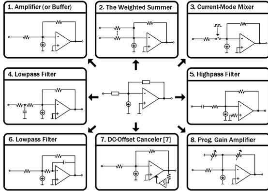
Fig. 4: Opamp-based functions in inverting configuration.
