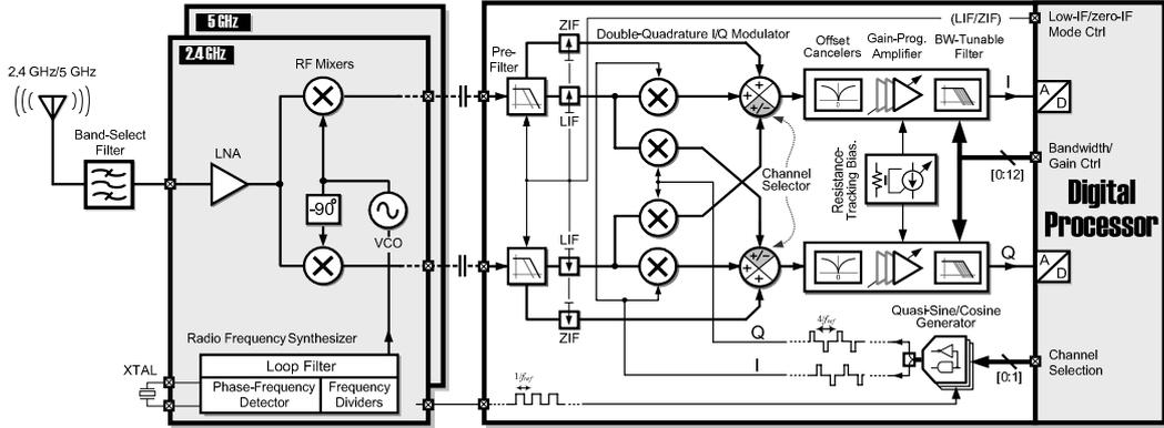
Fig. 2: Proposed low-IF/zero-IF reconfigurable receiver architecture.
