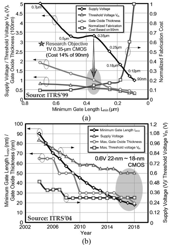
Fig. 1: Scaling of CMOS - (a) From microscale to 90 nm, (b) From 90 nm to 18 nm.
