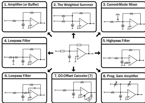
Fig. 4: Opamp-based functions in inverting configuration.
