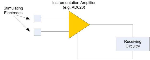
Fig. 3. Design of the IBC receiver
