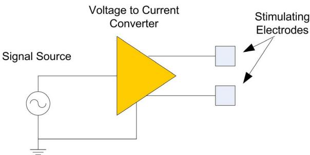
Fig. 2. Design of the IBC transmitter
