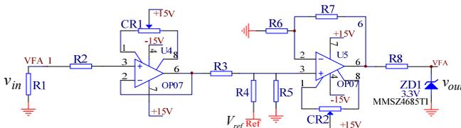
Fig. 2. Proposed signal conditioning circuit
