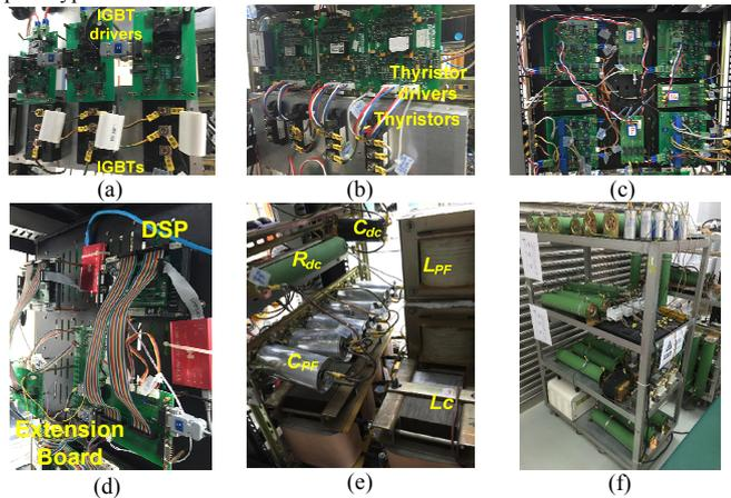
Fig. 5 The 110V-5kVA TCLC-HAPF and loading system: (a) IGBTs and their drivers, (b) thyristors and their drivers, (c) transducers with signal conditioning circuits, (d) DSPs and their extension boards, (e) TCLC part components, dc capacitor and discharge resistor and (f) loading system
