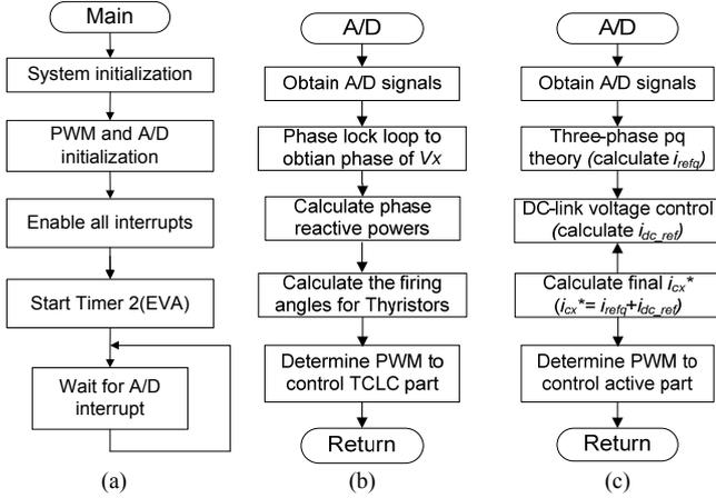
Fig. 3. DSP flowcharts of the TCLC-HAPF: (a) main program, (b) interrupt routine for the TCLC part and (c) interrupt routine for the active inverter part
