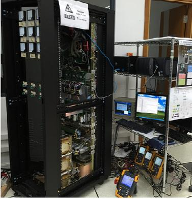
Fig. 4 Experimental setup of the 110V-5kVA TCLC-HAPF experimental prototype
