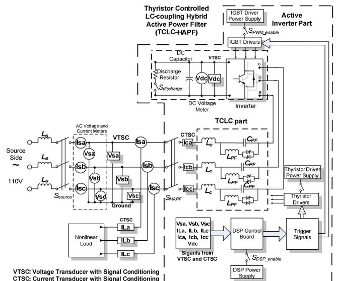
Fig. 1. System configuration of the 110V-5kVA TCLC-HAPF experimental prototype
