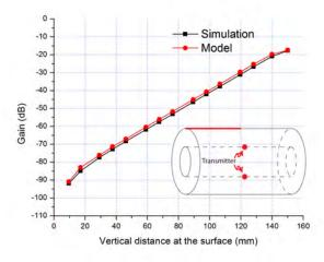
Fig. 4. Path loss along the limb surface from center to the end
