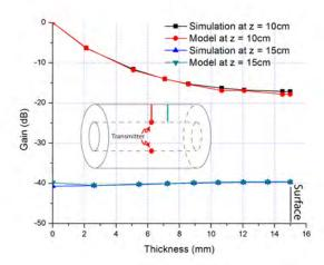
Fig. 3. Signal gain versus outward radial distance
