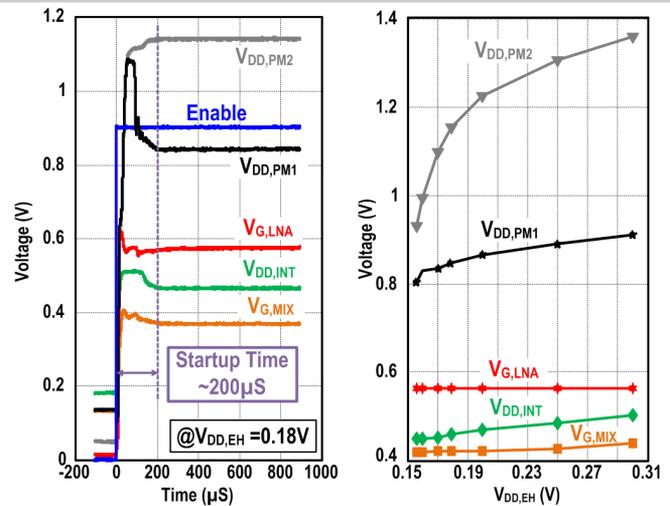
Figure 24.4.4: Measured startup time (left) and locking conditions (right) of the micropower manager. The very steady  $V_{G,LNA}$  stabilizes the RF performances against  $V_{DD,EH}$ .
