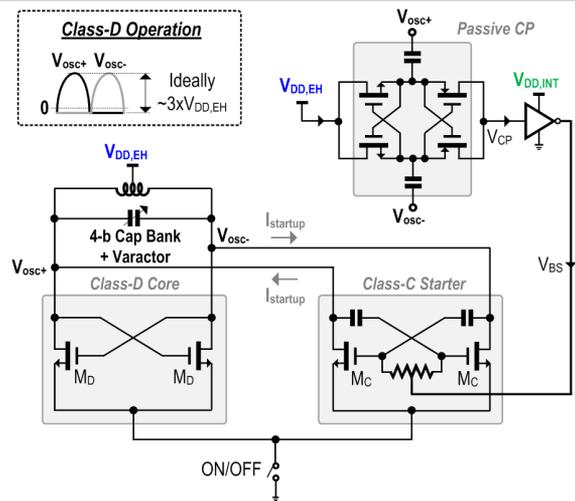
Figure 24.4.2: Proposed ULV Class-D VCO with a Class-C starter. The passive charge-pump (CP) senses  $V_{osc\pm}$  to activate/stop the Class-C starter during/after the startup process.
