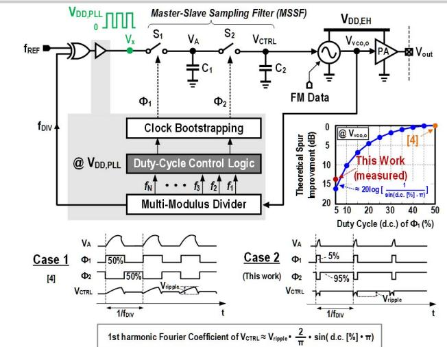
Figure 28.5.4: A 2.4GHz integer-N type-I PLL with passive XOR and MSSF. The MSSF uses a 5%-duty-cycle  $\Phi_1$  to aid suppressing the reference spurs.  $V_{DD,PLL}=0.55V$  and  $f_{ref}=1\text{MHz}$ .
