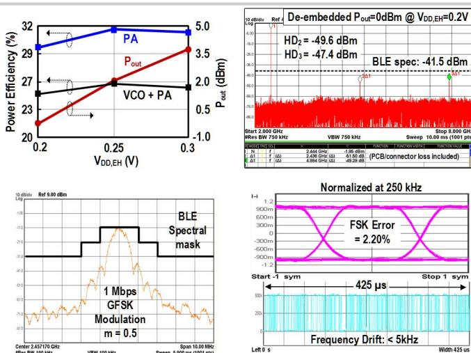
Figure 28.5.5: Upper: measured  $P_{out}$ , power efficiency and  $HD_{2,3}$ . Lower: measured modulated output spectrum, FSK error and frequency drift under open-loop operation.
