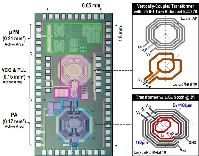
Figure 28.5.7: Die micrograph of the 28nm CMOS BLE TX and details of transformers. Extra pads are for individual characterization of the μPM, VCO and PA in active and sleep modes.
