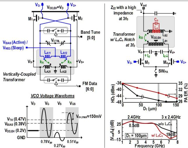
Figure 28.5.3: Left: ULV VCO with  $M_{1,2}$  always in saturation region even at  $V_{DD,EH}=0.2V$ . Right: ULV Class-E/F<sub>2</sub> PA, with its transformer-embedded  $L_nC_n$  notch to suppress  $HD_3$
