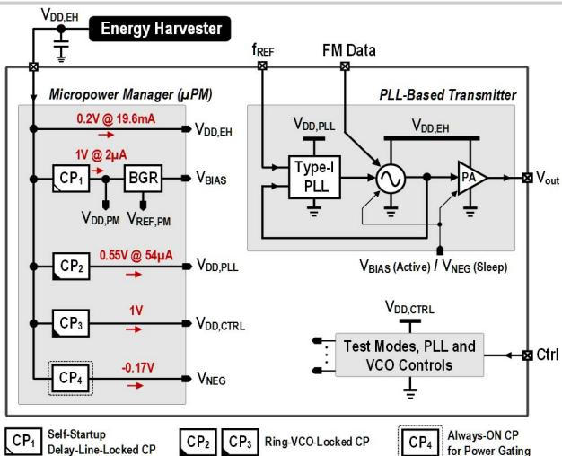
Figure 28.5.1: Proposed energy-harvesting BLE TX features a fully-integrated  $\mu\text{PM}$  to control the active/sleep power and tolerate variation of the energy source ( $V_{DD,EH}$ ) down to 0.2V.
