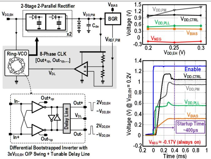
Figure 28.5.2: Left: CP<sub>1</sub> of the  $\mu\text{PM}$ . Its ring-VCO is locked via tunable delay lines to track  $V_{DD,EH}$  variation. Right: Measured internal voltages against  $V_{DD,EH}$  and their startup time.
