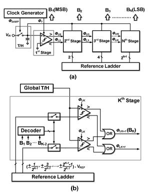
Fig. 2: (a) Block diagram of the second binary-search ADC [2] (b) Scheme of the K<sup>th</sup> stage.
