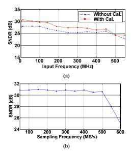
Figure 7. (a) SNDR versus input frequencies at  $f_S = 500MS/s$ (b) SNDR versus sampling frequencies
