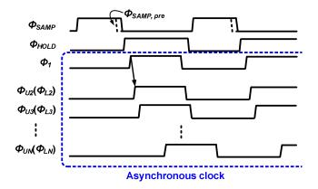
Fig. 4. Clock generation and asynchronous clock phase diagram
