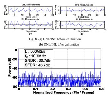
Fig. 9. FFT spectrum with 10.7MHz input (Output Decimated by 25)
