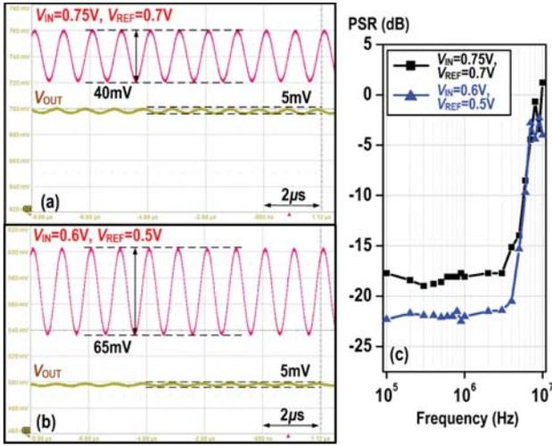
Fig. 8. The measured transient waveforms of  $V_{IN}$  and  $V_{OUT}$ , with  $I_{LOAD}=10mA$ ,  $f_{ripple}=1MHz$ ,  $f_{CLK}=5MHz$  when (a)  $V_{IN}=0.75V$  and  $V_{REF}=0.7V$ , (b)  $V_{IN}=0.6V$  and  $V_{REF}=0.5V$ ; and (c) the summary of the measured PSR from 100K to 10MHz under these two cases.
