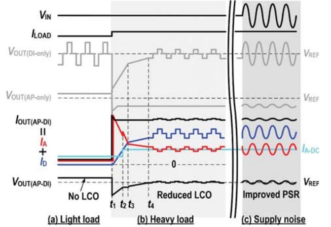
Fig. 3. The working principle of the proposed DLDO in the (a) light load, (b) heavy load, and (c) with supply noise conditions, and its comparison to the AP- and DI-only LDOs.
