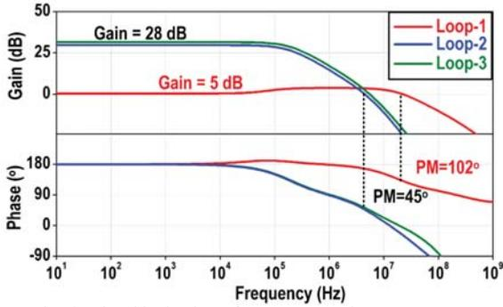
Fig. 2. The simulated bode plots of Loop-1, -2 and -3.
