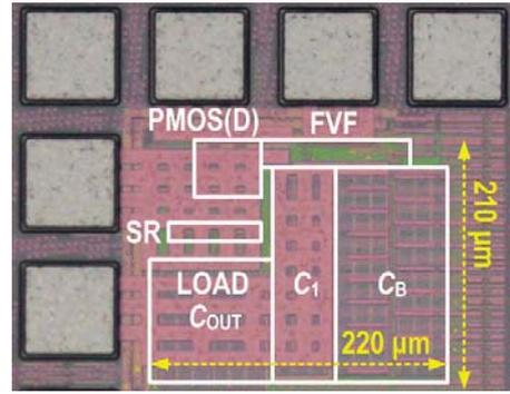
Fig. 6. Chip microphotograph of the proposed DLDO.
