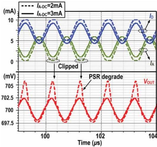
Fig. 5. The simulated transient waveforms of  $I_D$ ,  $I_A$  and  $V_{OUT}$  when  $I_{A-DC}$  is set to 2 (dashed line) and 3mA (bold line), respectively, with  $V_{IN}=0.75V$ ,  $V_{REF}=0.7V$ ,  $V_{ripple}=40mV_{pp}$ ,  $I_{LOAD}=10mA$ ,  $f_{ripple}=1MHz$ ,  $f_{CLK}=5MHz$ .
