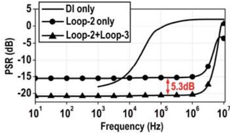
Fig. 4. The simulated PSR under  $V_{IN}=0.75V$ ,  $V_{REF}=0.7V$ ,  $V_{ripple}=40mV_{pp}$ ,  $I_{LOAD}=10mA$ ,  $f_{ripple}=1MHz$ ,  $f_{CLK}=5MHz$ , when DI only, Loop-2 only and both Loop-2 and 3 are applied.
