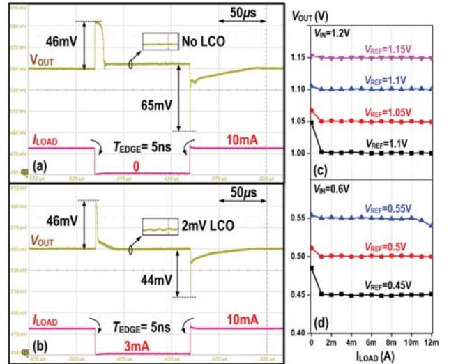
Fig. 7. The measured transient response with a (a) 0-10mA, and (b) 3-10mA  $I_{LOAD}$  step, when  $V_{IN}=0.6V$ ,  $V_{REF}=0.55V$ ,  $f_{CLK}=5MHz$ , with no or only 2mV LCO in the light load conditions; and the measured load regulation with (c) 0.6V and (d) 1.2V  $V_{IN}$ , respectively.
