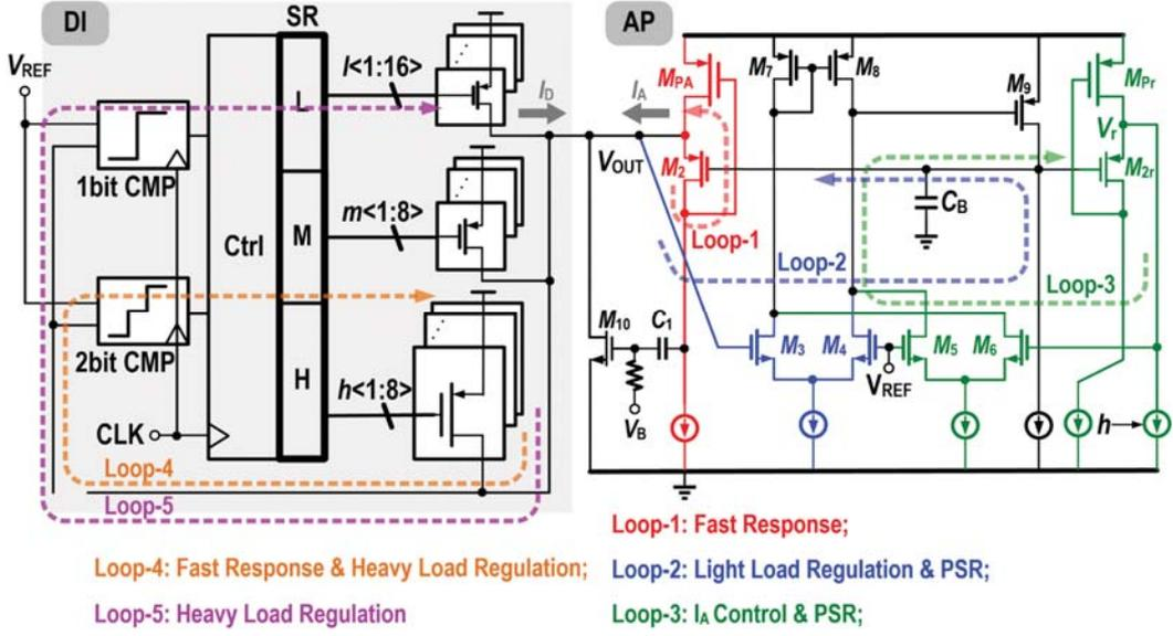
Fig. 1. The full schematic of the proposed DLDO with five control loops, and the function of each loop.
