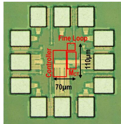
Fig.4. Chip micrograph of the proposed AF-DLDO.
