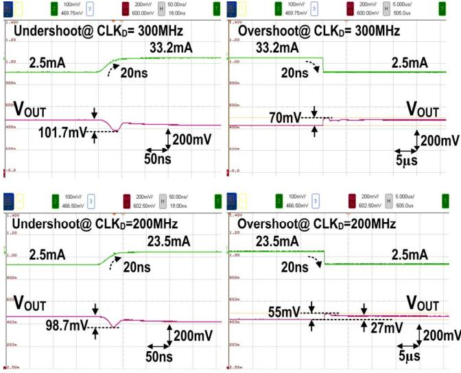
Fig. 5. Measured load transient response with  $V_{IN}=0.5V$ ,  $V_{OUT}=0.45V$ ,  $C_L=100pF$ , and load changes (a) from 2.5mA to 33.2mA within 20ns at  $CLK_D=300MHz$  and (b) from 2.5mA to 23.5mA at  $CLK_D=200MHz$ .
