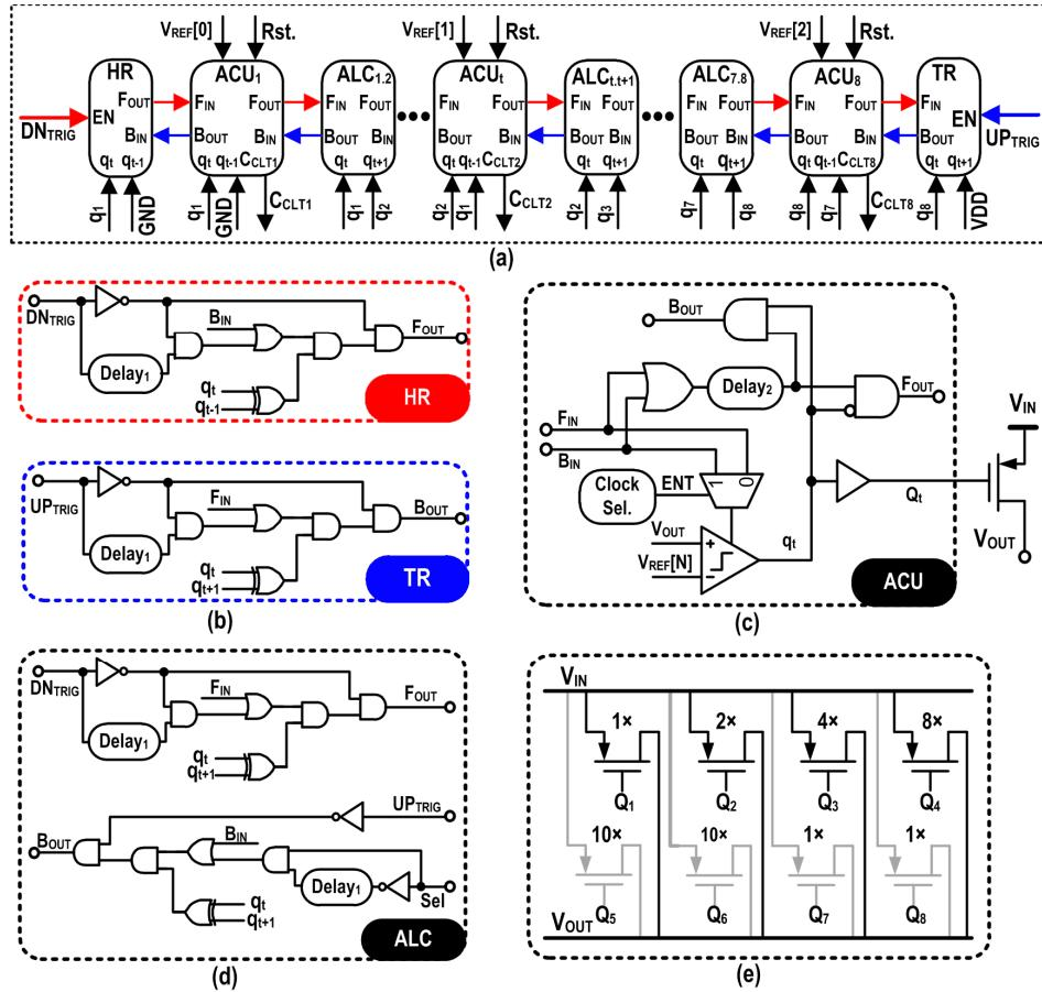
Fig.2. Implementation of the (a) asynchronous flash bidirectional SR; (b) heading reflector (HR); (c) asynchronous control unit (ACU); (d) architectural logic connector (ALC); and (e) power transistor in the AF directed coarse tuning loop.
