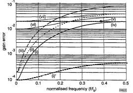
Fig. 2 Gain-error comparison of SC delay circuits ( $A = 100, C_i/C_j = 1$ ) (i) proposed Fig. 1
