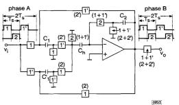
Fig. 3 Gain- and offset-compensated and mismatch-free SC  $z^{-1}$  (phase A) and  $z^{-3/2}$  (phase B) delay circuits
