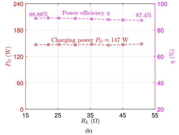
Fig. 15. (a) Measured output current and voltage versus battery resistance. (b) Measured power and efficiency versus battery resistance.
