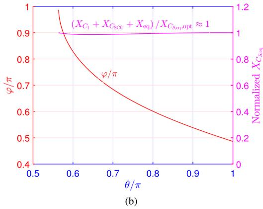
Fig. 7. (a) Conduction angle  $\theta$ , normalized  $R_{eq}$ , normalized  $X_{eq}$  versus load resistance  $R_L$ . (b) Phase delay angle  $\varphi$ , normalized  $X_{C_S,eq}$  versus conduction angle  $\theta$ .
