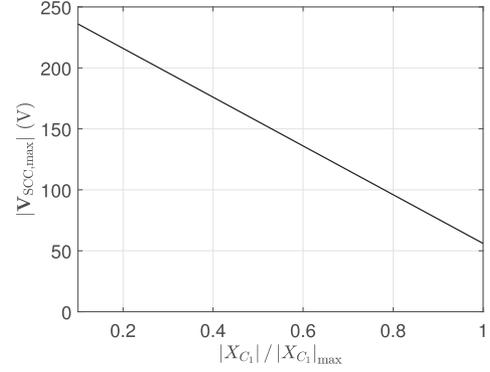
Fig. 11. Voltage stress  $|V_{SCC,max}|$  of the SCC versus design value of  $X_{C1}$ .
