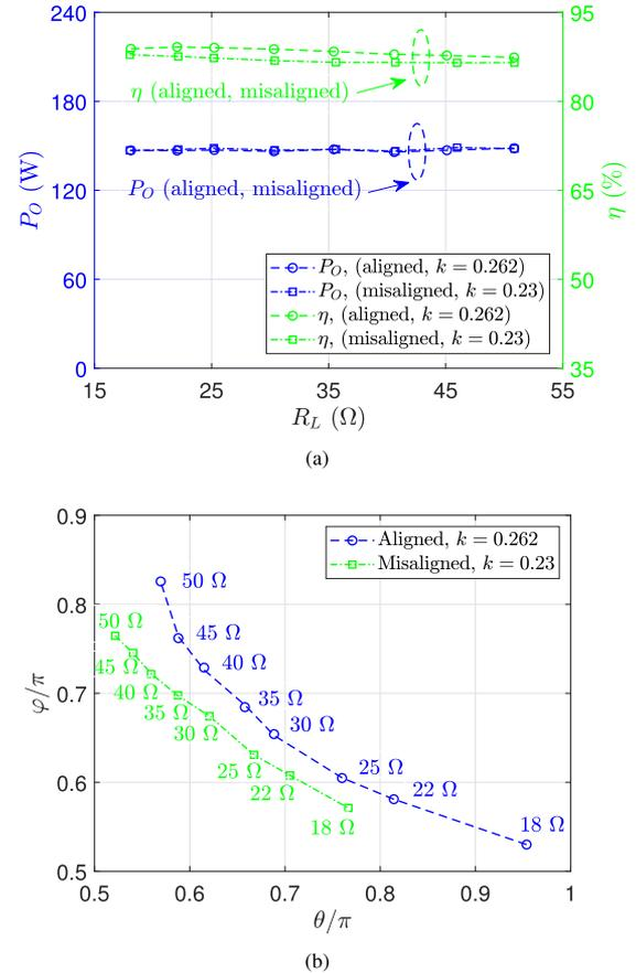
Fig. 18. Validation of the proposed method under aligned and misaligned conditions. (a) Measured output power and efficiency versus battery resistance. (b) Measured operating points.
