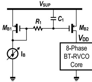
Fig. 9. Frequency tuning scheme for the proposed 8-phase BT RVCO.
