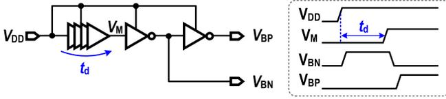
Fig. 6. Startup signal generation circuit.
