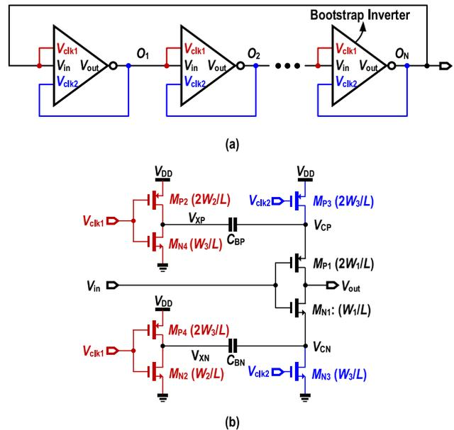
Fig. 1. (a) Single-ended BT RVCO and (b) schematic of the BT inverter.
