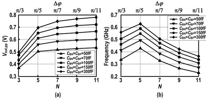
Fig. 3. Simulated (a) output swing and (b) oscillation frequency against the number of stage  $N$  and  $\Delta\varphi$  for a single-ended BT RVCO. ( $V_{\text{DD}} = 0.3\text{V}$ ,  $W_1 = 0.3\ \mu\text{m}$ ,  $W_2 = 1\ \mu\text{m}$ ,  $W_3 = 0.75\ \mu\text{m}$ ).
