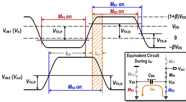
Fig. 2. Timing diagram of the  $V_{\text{clk}1,2}$  in the single-ended BT RVCO and the states of the transistors in the bottom charge pump during the time interval  $t_{\text{ov}}$ . This defines the conventional clocks under low-voltage supply.
