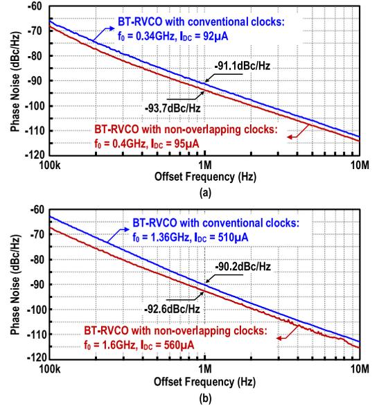
Fig. 11. Measured phase noise of the BT RVCOs using non-overlapping and conventional clocks at the (a) lowest and (b) highest frequencies.
