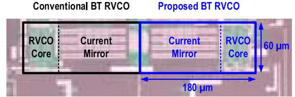
Fig. 10. Chip photo of the two fabricated BT RVCOs in 65-nm CMOS.
