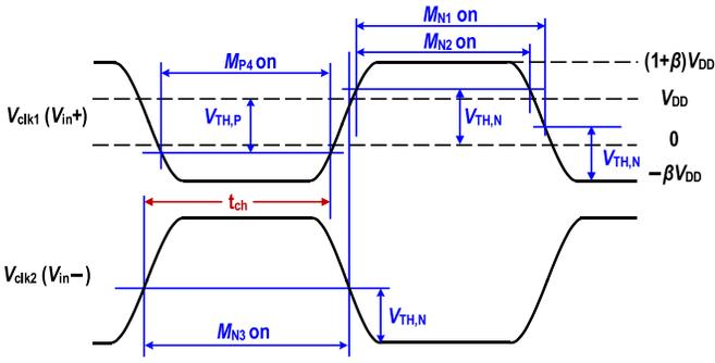
Fig. 5. Timing diagram of the clock signals in the 8-phase BT RVCO using non-overlapping clocks.
