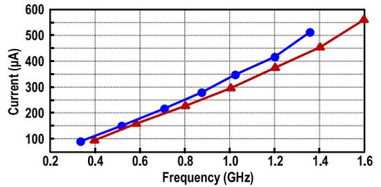
Fig. 12. Measured current consumptions of the two BT RVCOs with non-overlapping clocks (triangle symbols) and conventional clocks (circle symbols) versus the oscillation frequency.
