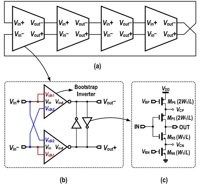
Fig. 4. (a) Block diagram of the proposed 8-phase BT RVCO core using non-overlapping clocks and (b) its pseudo-differential delay element. (c) Schematic of the cross-coupled inverter with auxiliary startup transistors.
