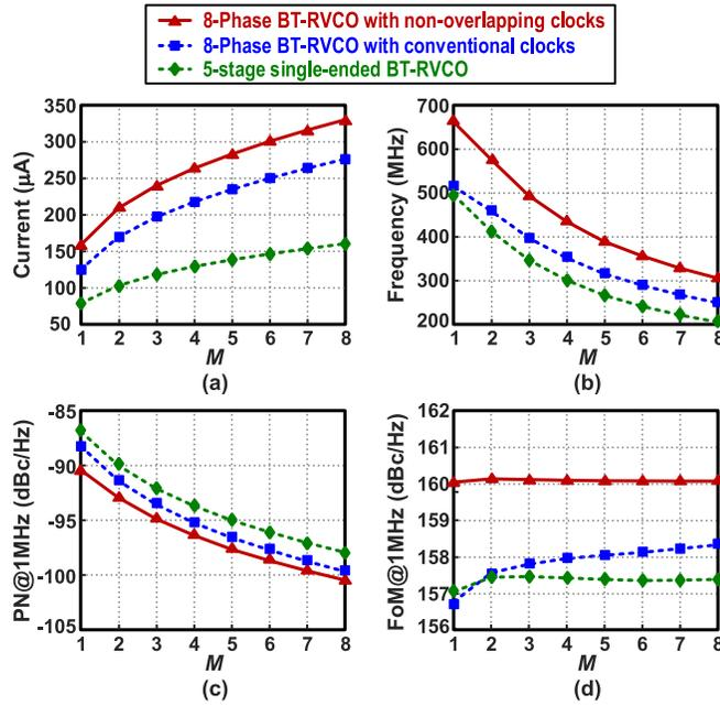
Fig. 8. Comparison of simulated (a) current, (b) oscillation frequency, (c) phase noise and (d) FoM for the 8-phase BT RVCOs using non-overlapping clocks and conventional clocks and 5-stage single-ended BT RVCO. ( $V_{DD} = 0.3$  V,  $W_2 = 1$   $\mu\text{m}$ ,  $W_3 = 0.75$   $\mu\text{m}$ ).
