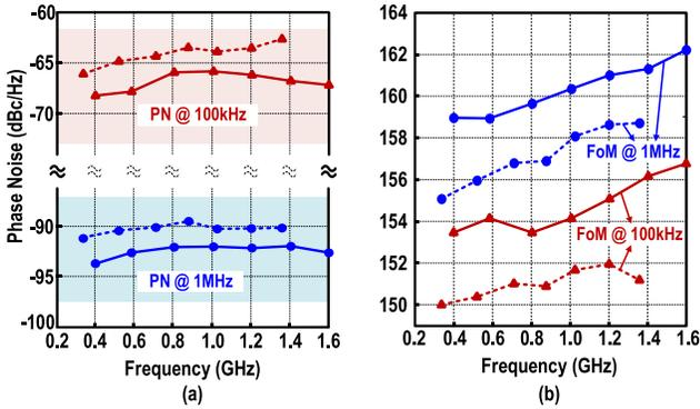
Fig. 13. Measured (a) phase noise and (b) FoM of the two BT RVCOs with non-overlapping clocks (solid lines) and conventional clocks (dashed lines) versus the oscillation frequency.
