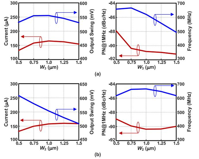
Fig. 7. Simulated current, output swing, oscillation frequency and phase noise of the 8-phase BT RVCO using non-overlapping clocks versus (a)  $W_3$  ( $W_2 = 1 \mu\text{m}$ ) and (b)  $W_2$  ( $W_3 = 0.75 \mu\text{m}$ ). ( $V_{DD} = 0.3\text{V}$ ,  $W_1 = 0.3 \mu\text{m}$ ,  $C_{BN} = C_{BP} = 70 \text{fF}$ ).
