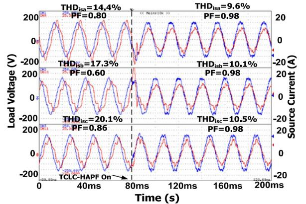
Fig. 10. Experimental waveforms of  $v_x$  and  $i_{sx}$  before and after the TCLC-HAPF compensation with the proposed selective compensation method ( $k_H = 1$ ,  $k_U = 1$ ,  $k_Q = 0.85$ ).
