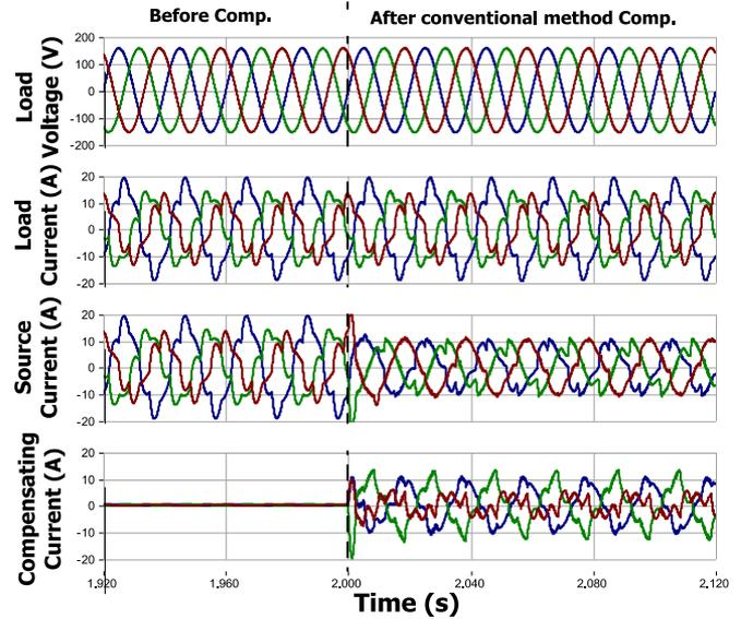
Fig. 6. Simulated distortion, unbalanced and reactive power compensation performances by using the conventional control strategy [14] of the TCLC-HAPF.
