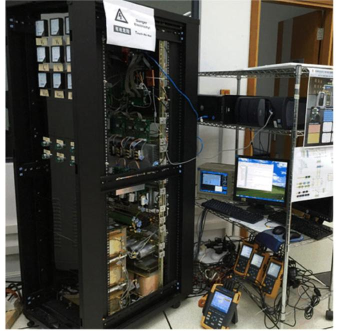
Fig. 9. Experimental setup of the TCLC-HAPF hardware prototype and its testing environment.
