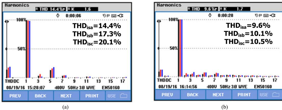
Fig. 13. Experimental current harmonic spectrums of  $i_{sx}$ : (a) before compensation (b) after the TCLC-HAPF compensation with the proposed selective compensation method ( $k_H = 1$ ,  $k_U = 1$ ,  $k_Q = 0.85$ ).
