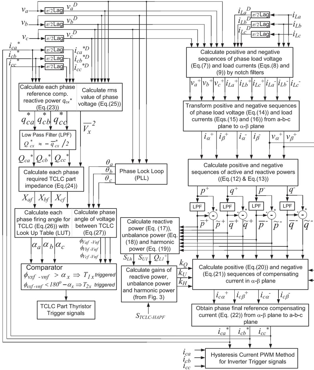
Fig. 4. Control block of the proposed selective compensation control strategy of TCLC-HAPF.
