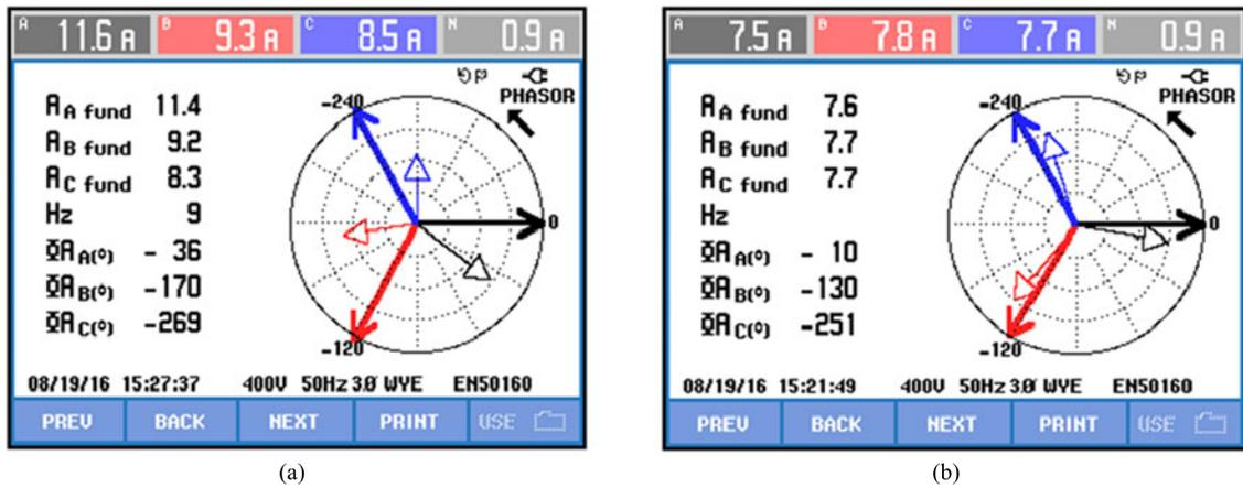
Fig. 12. Experimental phasor diagrams of  $v_x$  and  $i_{sx}$ : (a) before compensation (b) after the TCLC-HAPF compensation with the proposed selective compensation method ( $k_H = 1$ ,  $k_U = 1$ ,  $k_Q = 0.85$ ).
