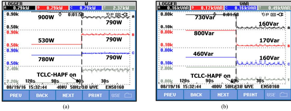
Fig. 11. Experimental results of dynamic performance before and after the TCLC-HAPF compensation with the proposed selective compensation method ( $k_H = 1$ ,  $k_U = 1$ ,  $k_Q = 0.85$ ): (a)  $P_{sx}$  and (b)  $Q_{sx}$ .
