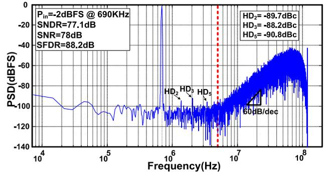
Fig. 14. Measured FFT output spectrum over a 5MHz bandwidth.
