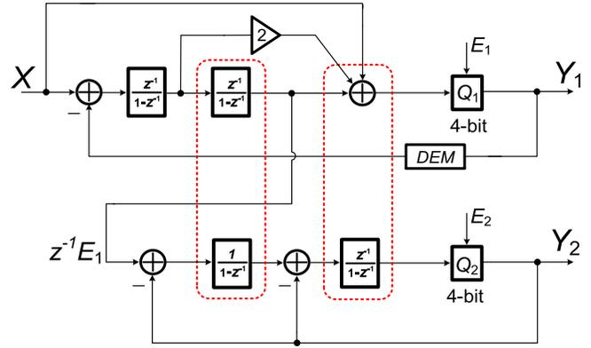
Fig. 1. Block diagram of the 2-2 MASH with vertical sharing proposed in [7].
