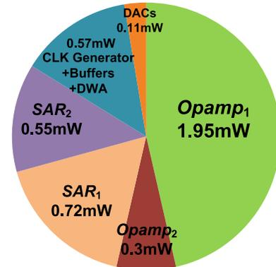
Fig. 17. Modulator power breakdown.
