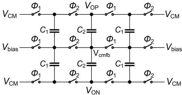
Fig. 9. The DT CMFB configuration for both horizontal and vertical sharing.
