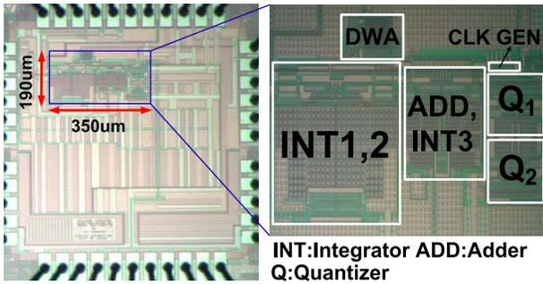
Fig. 12. Chip micrograph.
