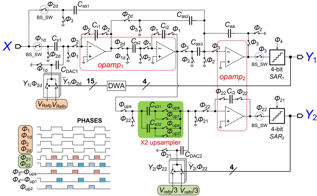
Fig. 10. The implementation of the proposed DT 2-1 MASH with multirate opamp sharing and the operating clock phases.
