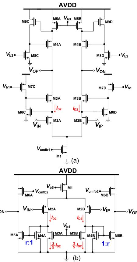
Fig. 8. (a) The topology of the  $opamp_1$  for horizontal sharing. (b) The topology of the  $opamp_2$  for vertical sharing.
