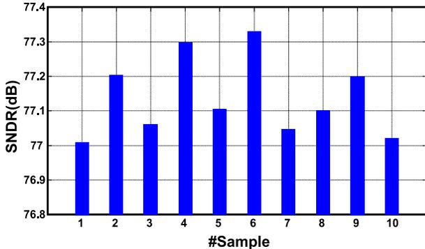
Fig. 13. Measured SNDR over 10 samples with a 690kHz input frequency.
