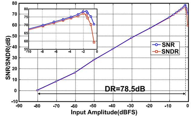
Fig. 16. Measured SNR/SNDR versus input amplitude with a 690kHz input.
