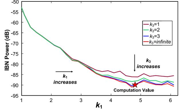
Fig. 7. The total IBN power versus  $k_1$  with different values of  $k_3$ .
