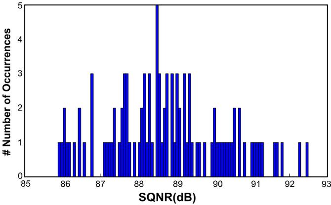
Fig. 5. Monte Carlo simulation with 0.1% capacitor mismatch.
