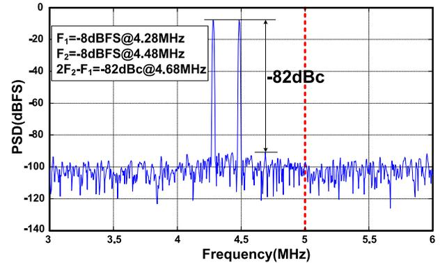
Fig. 15. Measured IMD3 of the  $\Delta\Sigma$  modulator output over a 5MHz bandwidth.
