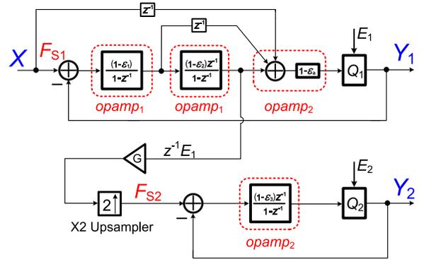
Fig. 6. DT 2-1 MASH with gain errors induced by finite GBW of opamps.
