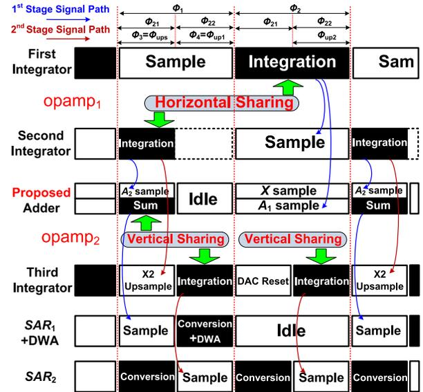
Fig. 3. The timing chart for the proposed DT 2-1 MASH operation.
