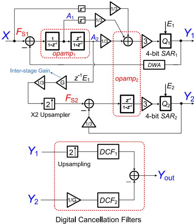
Fig. 2. Block diagram of the proposed DT 2-1 MASH together with the digital cancellation filters.
