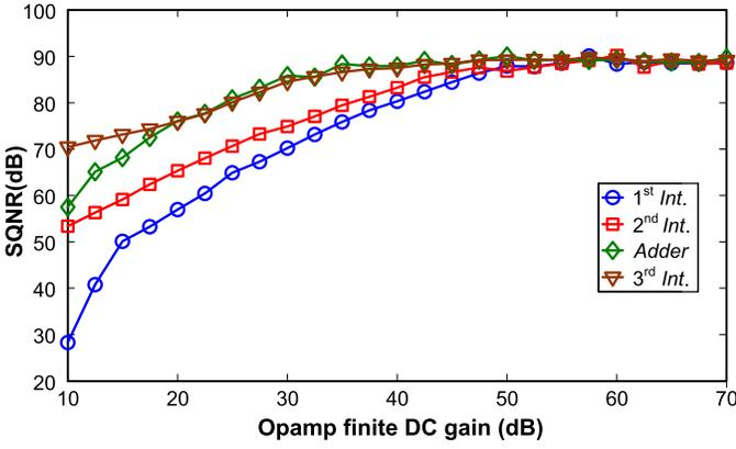
Fig. 4. The SQNR of the modulator versus opamp finite DC gain.
