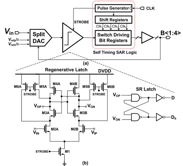
Fig. 11. (a) Block diagram of a 4-bit SAR quantizer with a self-timing scheme. (b) Implementation of the comparator.
