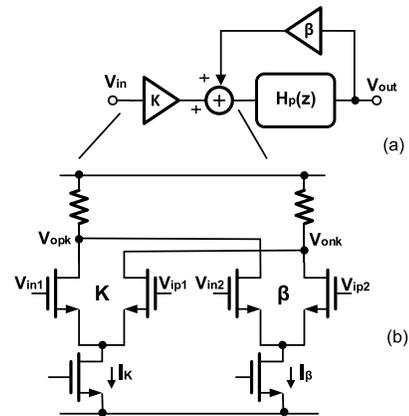
Fig. 2. (a) Compensation technique model. (b) Circuit implementation.
