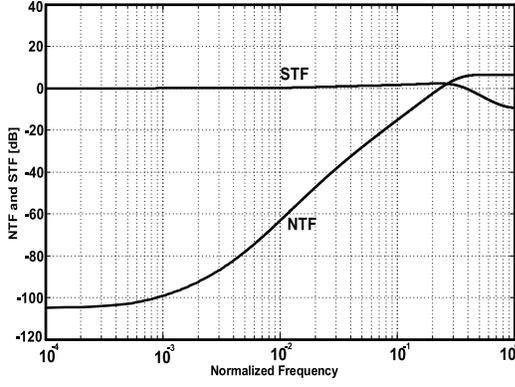
Fig. 6. STF and NTF of the modulator.
