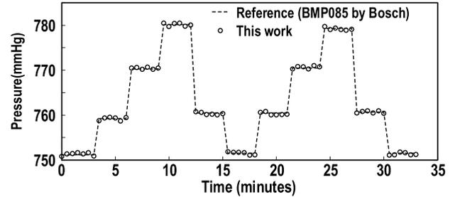
Fig. 15. Dynamic pressure measurement with a reference pressure sensor.
