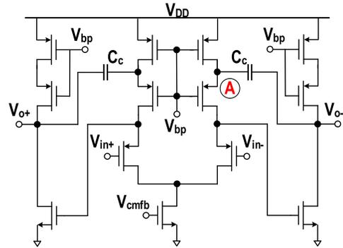
Fig. 9. Schematic of the two-stage amplifier in the integrators.
