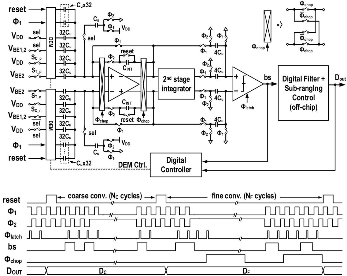
Fig. 8. Detailed schematic of the readout circuit and timing diagram.
