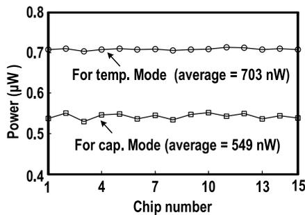
Fig. 11. Measured power consumption of capacitance and temperature sensing modes (15 chips).
