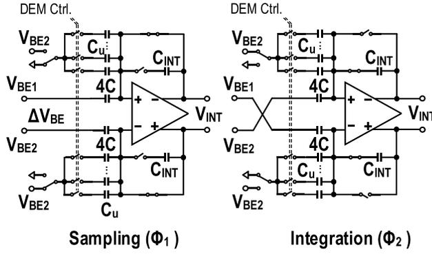
$$\text{Temperature Mode: } V_{\text{INT}} = (4\Delta V_{\text{BE}} - V_{\text{BE2}}) 2C / C_{\text{INT}}$$
