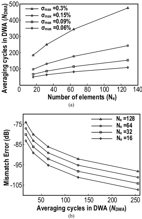
Fig. 2. (a) The DWA averaging cycles  $N_{DWA}$  against  $N_e$  for various  $\sigma_{max}$ , with  $e_{MIS} = -92$ dB. (b)  $e_{MIS}$  versus the DWA averaging cycles for different  $N_e$  with identical  $\sigma_{max}$  of 0.1%.
