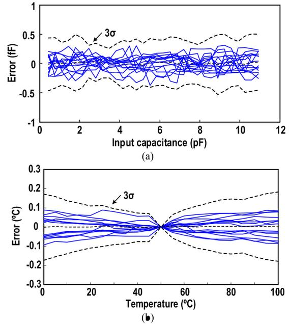
Fig. 12. (a) Measured capacitance error via 15 chips after individual calibration, with bold dashed lines indicating the  $\pm 3\sigma$  bounds. (b) Measured temperature error via 15 chips after one-point calibration at 50 °C, with bold dashed lines indicating the  $\pm 3\sigma$  bounds.
