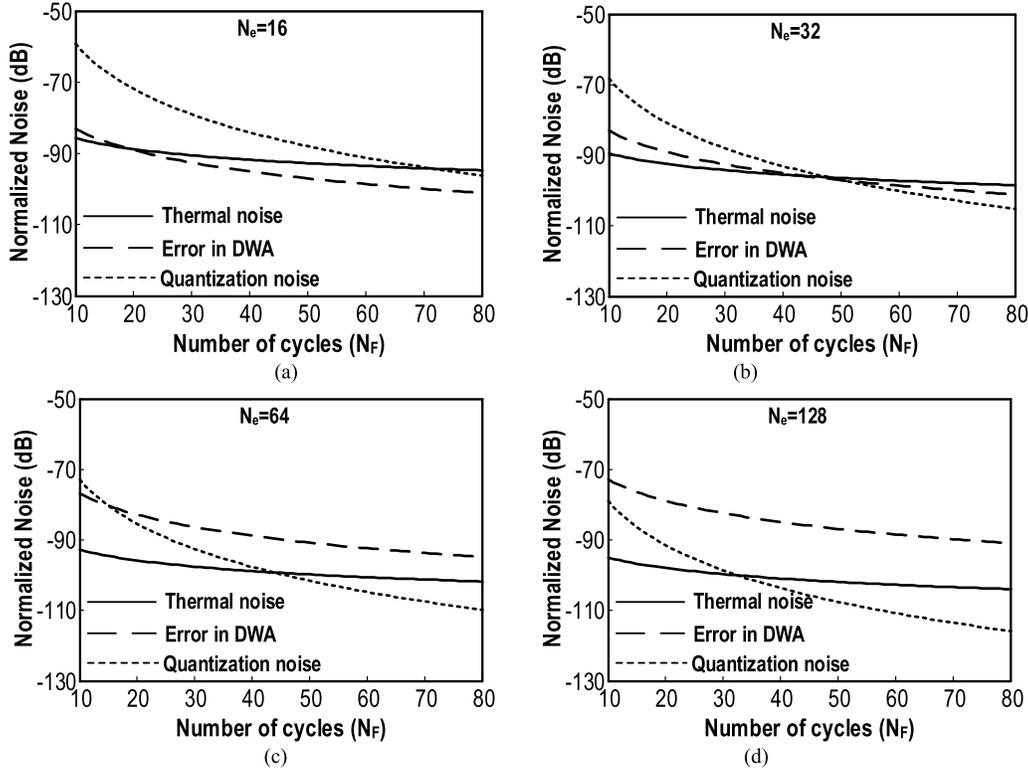
Fig. 4. Noise sources (thermal noise, mismatching error, and quantization noise) in fine conversion for different  $N_e$ .
