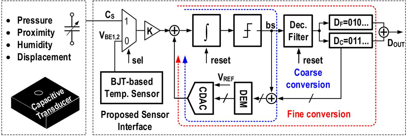
Fig. 1. System overview for capacitive sensor readout with the proposed sensor interface, where CDAC serves as the reference cap  $C_{REF}$ .
