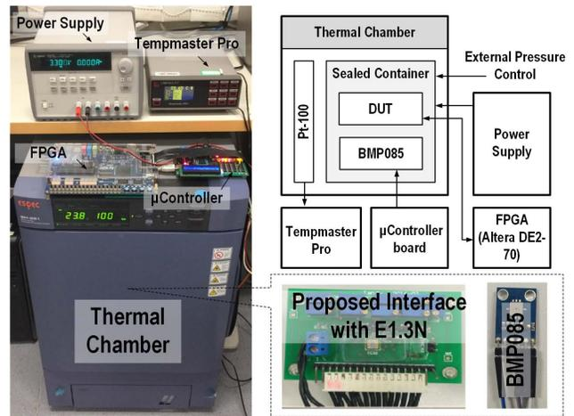
Fig. 13. System measurement setup of the proposed capacitive sensor readout.
