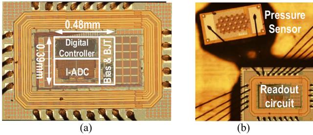
Fig. 10. (a) Die photo of the proposed capacitive sensor readout. (b) Assembly of the MEMS pressure sensor and the readout circuit.
