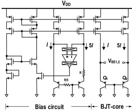
Fig. 5. Schematic of bias circuit and BJT-core for temperature sensing (DEM of current source in BJT-core omitted for clarity).
