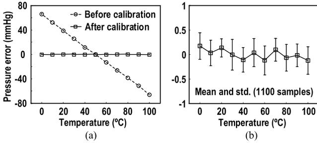
Fig. 14. System level measurement: (a) pressure accuracy before and after temperature compensation; and (b) close-up after calibration.
