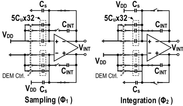
$$\text{Capacitance Mode: } V_{\text{INT}} = 2V_{\text{DD}}(C_{\text{S}} - 5C_{\text{u}}) / C_{\text{INT}}$$
