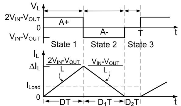
Fig. 3. Idealized  $V_L$  and  $I_L$  waveforms of KY converter in DCM.
