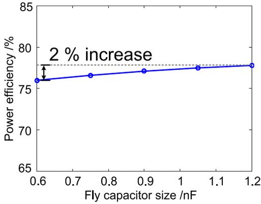
Fig. 6. The efficiency versus flying capacitor  $C_f$  size.
