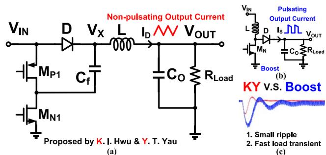
Fig. 1. (a) KY converter. (b) Conventional boost converter. (c) Comparison in terms of ripple and load transient response between the KY and the conventional boost converters.
