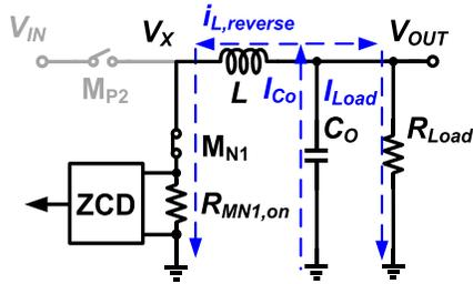
Fig. 10. Conventional ZCD for buck converter.
