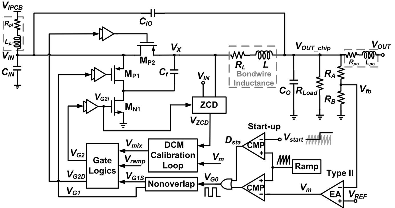
Fig. 7. Block diagram of the proposed fully integrated KY converter under DCM operation (overall system).
