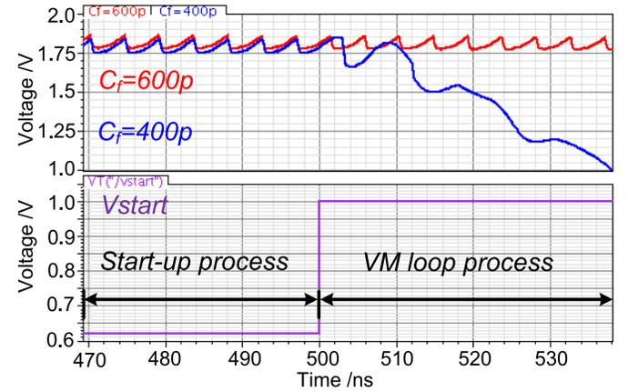
Fig. 5.  $V_{OUT}$  waveform when  $V_{IN} = 1.2$  V and target  $V_{OUT} = 1.8$  V,  $f_s = 220$  MHz and  $R_{Load} = 30 \Omega$ , with  $C_f = 400$  pF and 600 pF.
