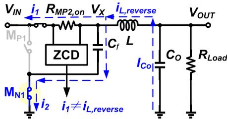
Fig. 11. Problem of conventional ZCD for KY the converter.
