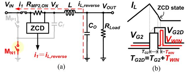
Fig. 12. Proposed ZCD for KY converter: (a) circuit and (b) gate signal.
