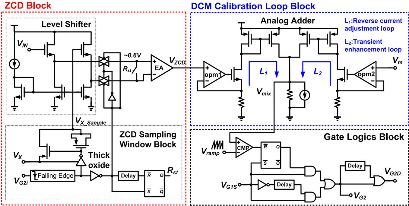
Fig. 13. Proposed ZCD and DCM calibration loop with load transient enhancement circuitry [2] for the KY converter under DCM operation.
