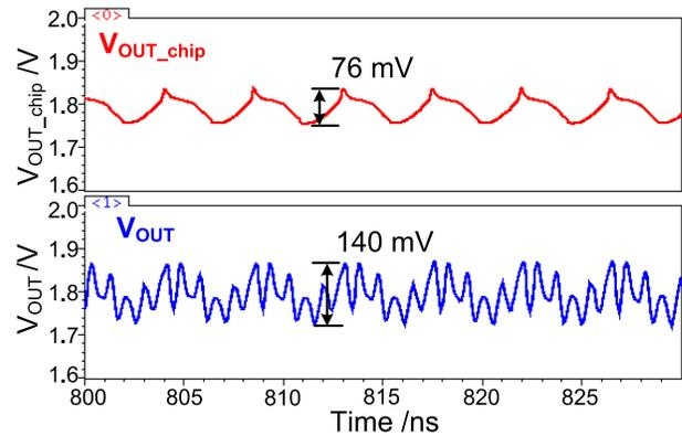
Fig. 19. Simulated on-chip output voltage  $V_{OUT\_chip}$  and off-chip output voltage  $V_{OUT}$  under  $V_{IN} = 1.2$  V,  $V_{OUT} = 1.8$  V,  $I_{Load} = 40$  mA.
