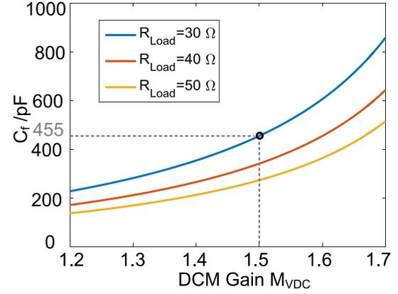
Fig. 4.  $C_f$  versus  $M_{VDC}$  with different  $R_{Load}$  when  $f_s = 220$  MHz.
