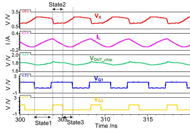
Fig. 20. The simulated  $V_X$ ,  $I_L$ ,  $V_{OUT\_chip}$ ,  $V_{G1}$  and  $V_{G2}$  waveforms of the proposed KY converter.
