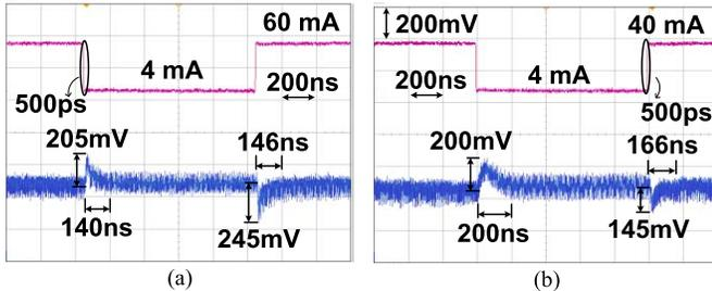
Fig. 16. Load transient response of the proposed KY converter under DCM operation at: (a)  $V_{OUT} = 1.5$  V and (b)  $V_{OUT} = 1.8$  V.
