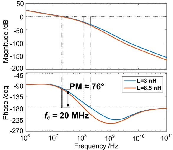
Fig. 9. The loop gain bode diagram of the designed KY converter in:  $L = 3$  nH and  $L = 8.5$  nH.
