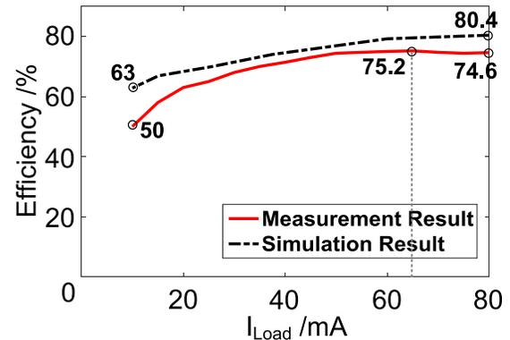
Fig. 17. Simulation and measurement results of power efficiency with DCM control under  $V_{IN} = 1.2$  V and  $V_{OUT} = 1.5$  V.
