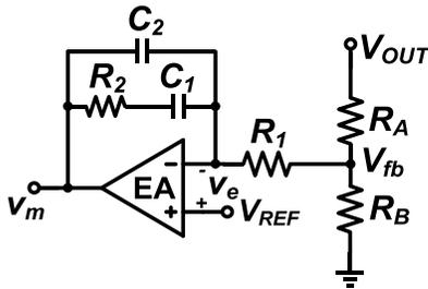
Fig. 8. Integral-single-lead (Type II) compensator.
