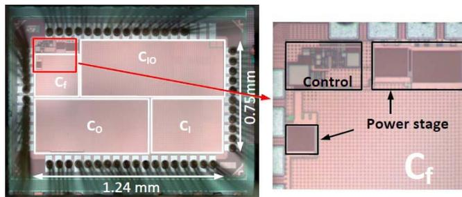
Fig. 14. Chip microphotograph of the proposed KY converter in DCM.
