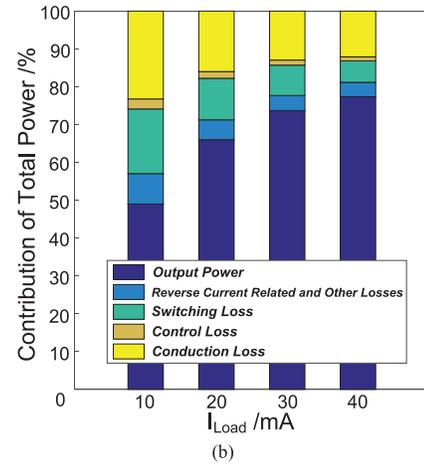
Fig. 15. (a) Measurement power efficiency of the proposed KY converter for  $V_{IN} = 1.2$  V and  $V_{OUT} = 1.5, 1.6, 1.7, 1.8$  V under different load current. (b) Power distribution graph under  $V_{IN} = 1.2$  V,  $V_{OUT} = 1.8$  V and  $I_{Load} = 10 - 40$  mA based on post layout simulation.
