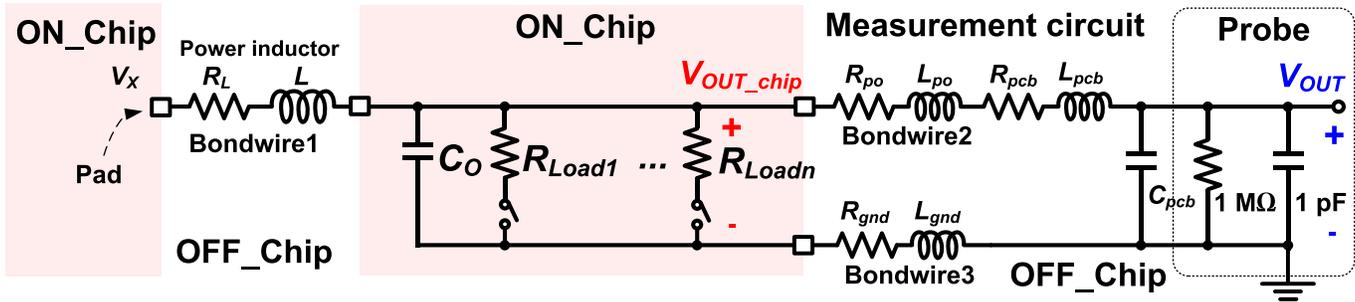
Fig. 18. Equivalent circuit of the KY converter measurement setup.
