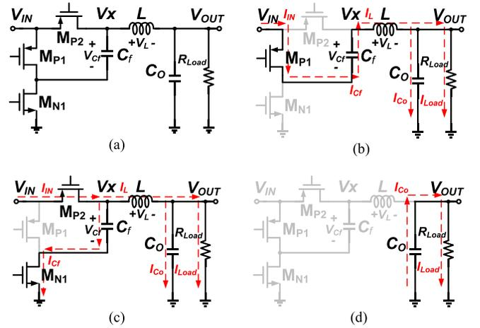
Fig. 2. DCM operation of the KY converter in IC. (a) Overall circuit. (b) State 1: Inductor  $L$  magnetized and  $C_f$  discharged. (c) State 2: Inductor  $L$  demagnetized and  $C_f$  charged. (d) State 3: Output capacitor  $C_O$  discharged.
