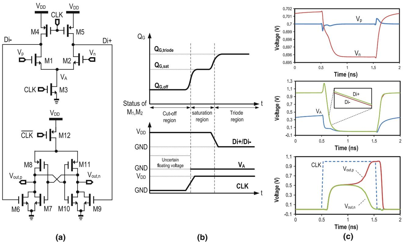
Fig. 2 a A conventional dynamic latched comparator. b The timing diagram shows the states and charge induced on the gate of M<sub>1</sub> (M<sub>2</sub>). c The simulated operation voltages of critical nodes
