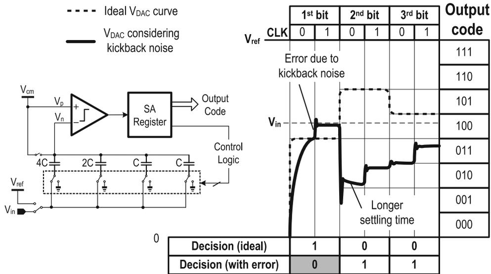
Fig. 1 SAR-type ADC with error code and longer settling time due to kickback noise
