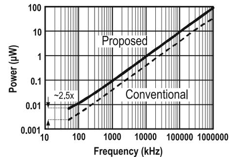
**Fig. 8** Dynamic power versus the CLK frequency of the conventional and proposed comparators
