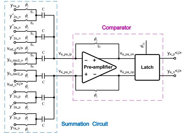
Fig. 10. Schematic diagram of a comparator of the 4-bit quantizer used in the even path together with the passive summation circuit ( $C = 5 \text{ fF}$ ).
