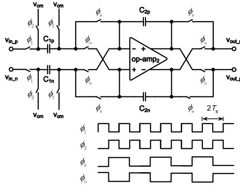
Fig. 5. The conventional circuit implementation of the chopper integrator with delay together with phases timing.
