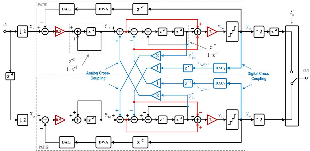
Fig. 4. Improved block diagram of the proposed third-order two-path  $\Sigma\Delta$  modulator with cross-coupling branches.
