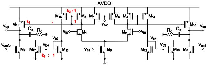
Fig. 9. Schematic diagram of the current-mirror op-amp in the chopper integrator.
