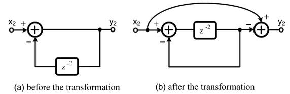
Fig. 3. The transformation from  $1/(1 + z^{-2})$  to  $1 - [z^{-2}/(1 + z^{-2})]$ .
