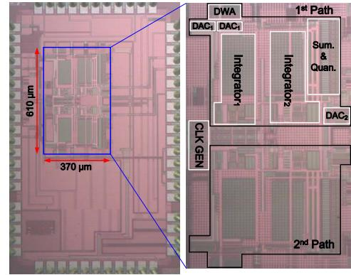
Fig. 11. Chip micrograph.
