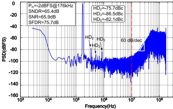
Fig. 12. Measured output spectrum.
