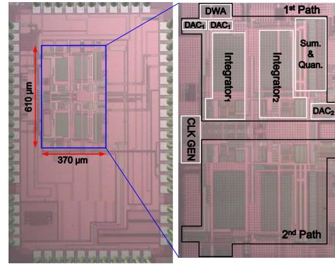
Fig. 11. Chip micrograph.
