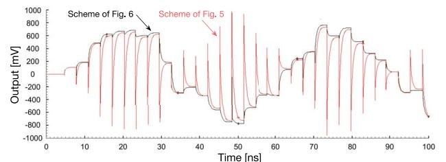
Fig. 7. Simulated output voltages of the chopper integrator, implemented with the schemes of Fig. 5 and Fig. 6.
