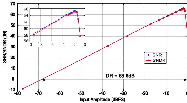
Fig. 13. Measured SNR and SNDR as a function of the input signal amplitude for a 176-kHz input.
