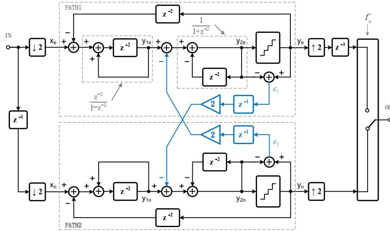
Fig. 1. Block diagram of the proposed third-order  $\Sigma\Delta$  modulator using a two-path architecture with cross-coupling branches ( $z = e^s/f_s$ ,  $z^2 = e^{2s}/f_s$ ).
