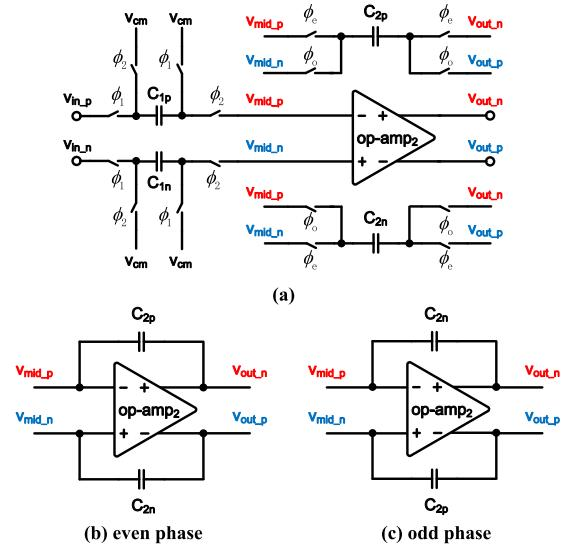
Fig. 6. The improved circuit implementation of the chopper integrator with delay: (a) the scheme, (b) and (c) the simplified circuit in the even and in the odd phase, respectively.
