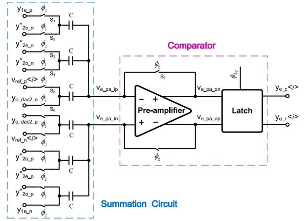
Fig. 10. Schematic diagram of a comparator of the 4-bit quantizer used in the even path together with the passive summation circuit ( $C = 5$  fF).
