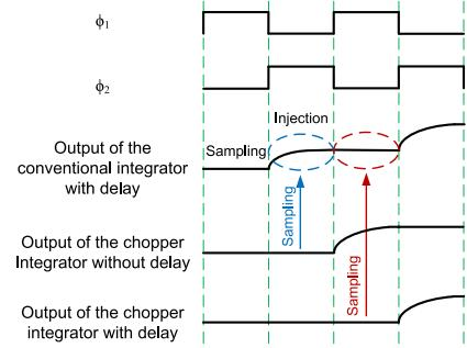
Fig. 2. The problem of the chopper integrator without delay.
