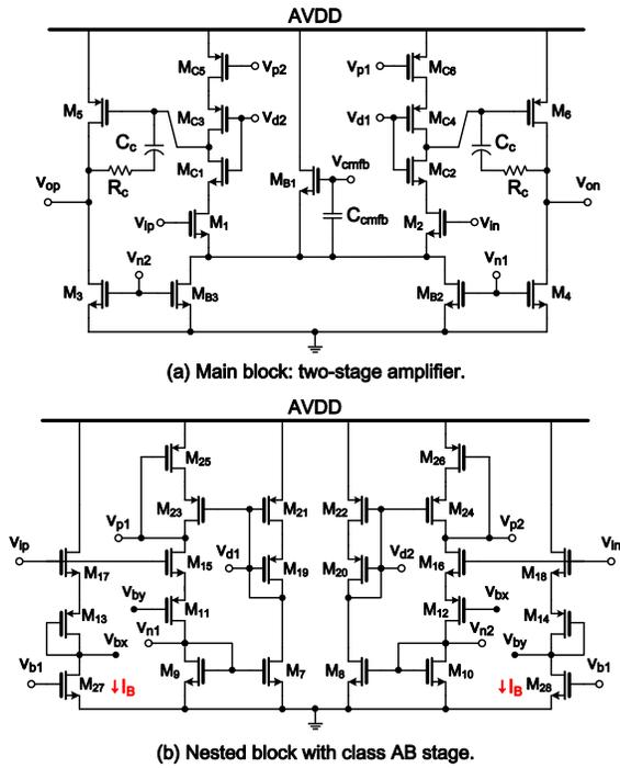
Fig. 8. Schematic diagram of the op-amp used in the conventional integrator: (a) two-stage amplifier and (b) nested block with class AB stage.
