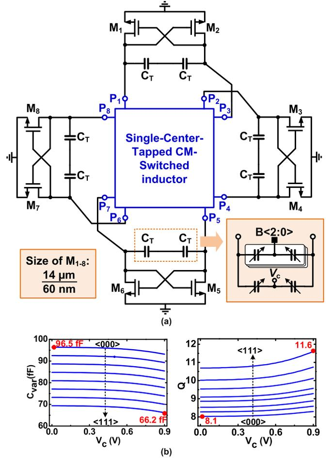
Fig. 9. (a) Schematic of the quad-core-coupled VCO using the proposed SCT switched inductor. (b) Simulated capacitance and  $Q$  of the varactor bank.
