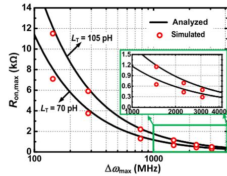
Fig. 12. Simulated and calculated  $R_{ON,\max}$  versus  $\Delta\omega_{\max}$  for Mode-H under the worst case frequency arrangement ( $f_F = 47.6$  GHz).
