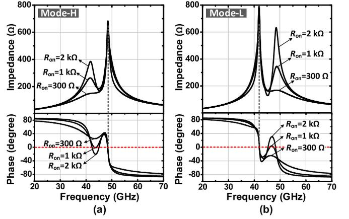
Fig. 10. Simulated amplitude and phase response of the tank impedance for (a) Mode-H and (b) Mode-L. ( $L_0 = 85$  pH,  $L_{CM} = 17$  pH,  $k_2 = 0.15$ , and  $Q_T = 15$ ).
