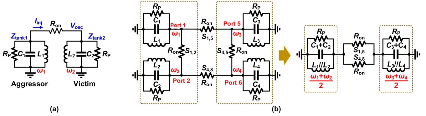
Fig. 11. Equivalent circuits for the frequency synchronization analysis of (a) dual-core coupled VCO and (b) mode-switching quad-core-coupled VCO in Mode-H.
