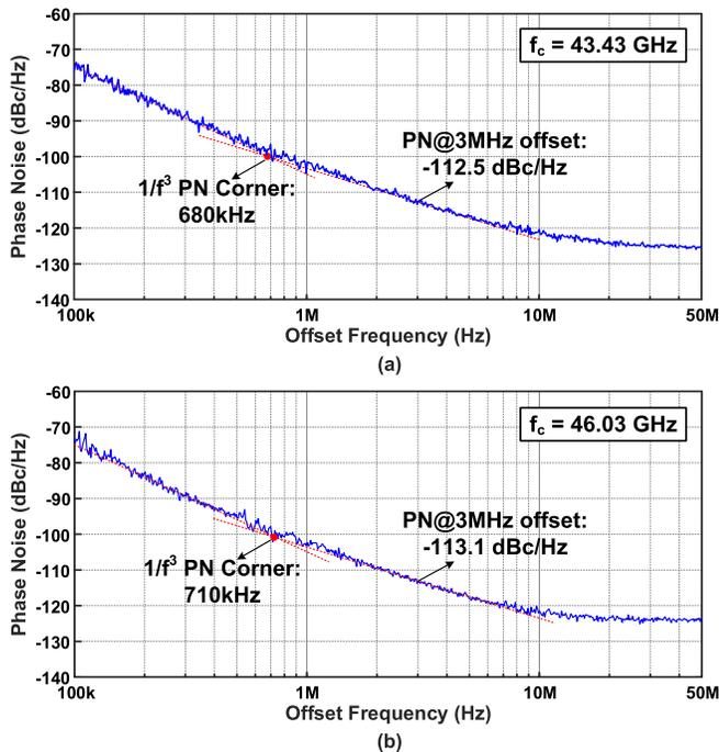
Fig. 17. Measured PN versus offset frequencies at carrier frequencies of (a) 43.43 GHz (Mode-L) and (b) 46.03 GHz (Mode-H).
