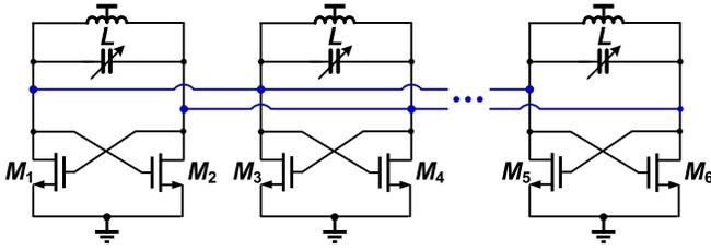
Fig. 1. Multiple VCO cores coupled in parallel allows PN reduction.
