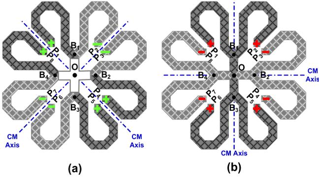
Fig. 6. Port excitations of the quad-core-coupled VCO using the SCT switched inductor in (a) Mode-H and (b) Mode-L.
