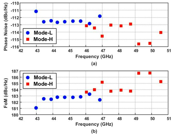
Fig. 18. Measured (a) PN and (b) FoM at 3-MHz offset versus carrier frequencies.
