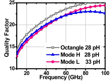
Fig. 7. EM simulated  $Q_s$  of the SCT switched inductor and the conventional single-turn octangle inductor.
