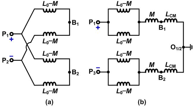
Fig. 4. Equivalent tank inductance of (a) Model-H and (b) Model-L assuming ideal switches.
