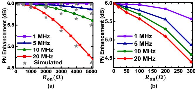
Fig. 13. PN enhancement versus  $R_{ON}$  at different offset frequencies for Mode-H at  $L_0 = 85$  pH,  $C_T = 80$  fF, and  $Q_T = 15$ : (a) without frequency mismatch ( $\omega_1 = \omega_2 = \omega_3 = \omega_4$ ) and (b) with 7% frequency mismatch ( $\omega_1 = \omega_2 < \omega_3 = \omega_4$ ).
