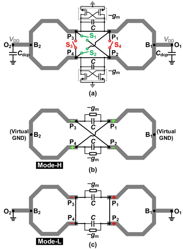
Fig. 2. (a) Proposed switched inductor applied to a dual-core-coupled VCO. (b) Illustration of the tank for Mode-H when the switches  $S_1$  and  $S_2$  are turned on and  $S_3$  and  $S_4$  are turned off. (c) Illustration of the tank for Mode-L when the switches  $S_3$  and  $S_4$  are turned on, and  $S_1$  and  $S_2$  are turned off.
