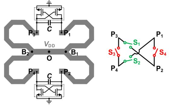
Fig. 5. Dual-core-coupled VCO with an SCT switched inductor.
