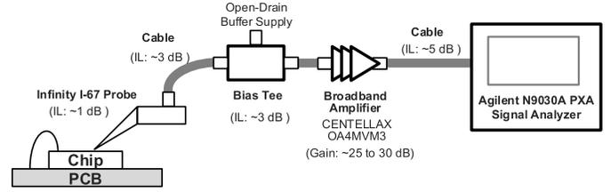
Fig. 15. PN measurement setup.
