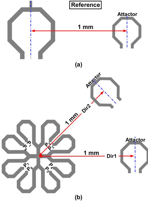
Fig. 8. Floor plan of the EM simulation for injection pulling from other circuits with on-chip inductors. (a) Victim is a conventional octangle inductor as a reference. (b) Victim is the SCT switched inductor.
