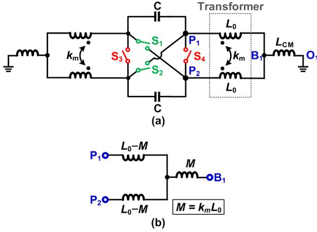
Fig. 3. (a) Tank model of the mode-switching dual-core-coupled VCO. (b) T-model for the transformer.
