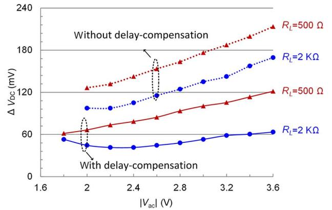
Fig. 20. Measured output voltage ripples.
