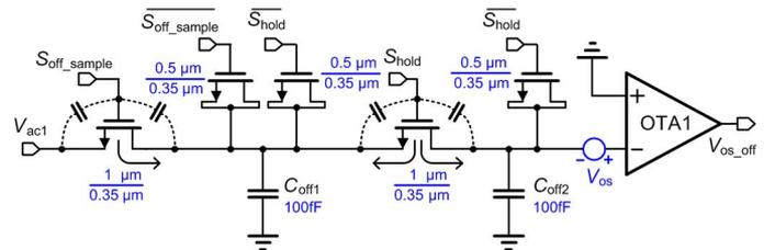
Fig. 13. Detailed schematic of the sampling circuit.
