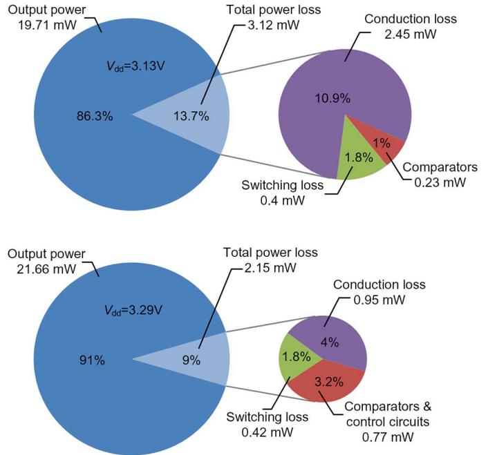
Fig. 12. Power distribution of the active rectifier. (a) Without the proposed technique. (b) With the proposed technique.
