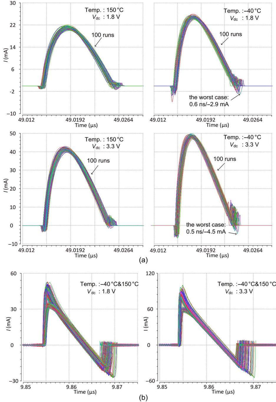
Fig. 14. Monte Carlo simulation waveforms of  $I_{ac1}$ . (a) With delay-compensation. (b) Without delay compensation.
