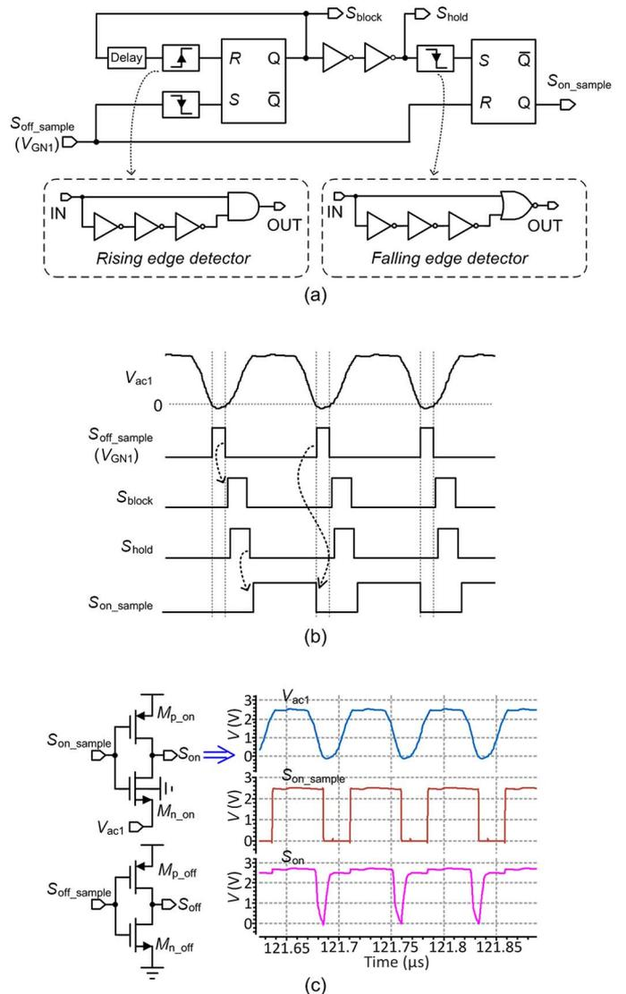
Fig. 9. (a) Control logic. (b) Timing diagram. (c) Simulated waveforms.
