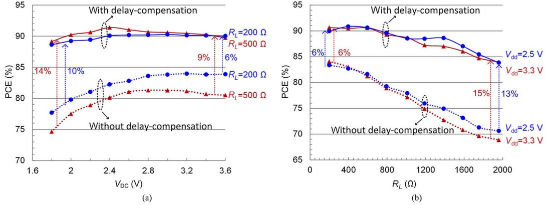
Fig. 21. Measured PCE under (a) different  $V_{DC}$  and (b) different  $R_L$ .TABLE III
