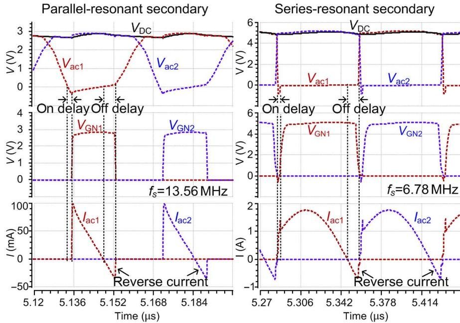
Fig. 4. Waveforms of active rectifiers.
