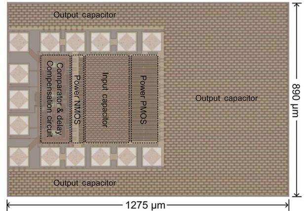
Fig. 17. Chip micrograph of the proposed active rectifier.
