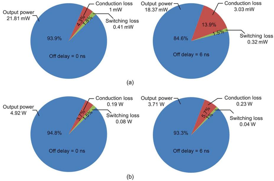
Fig. 6. Power distribution of the active rectifiers with (a) the parallel-resonant secondary; (b) the series-resonant secondary when the off-delays are 0 and 6 ns, respectively.
