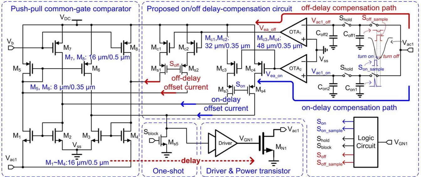
Fig. 7. Schematic of the active diode with the proposed adaptive on/off delay-compensation technique.
