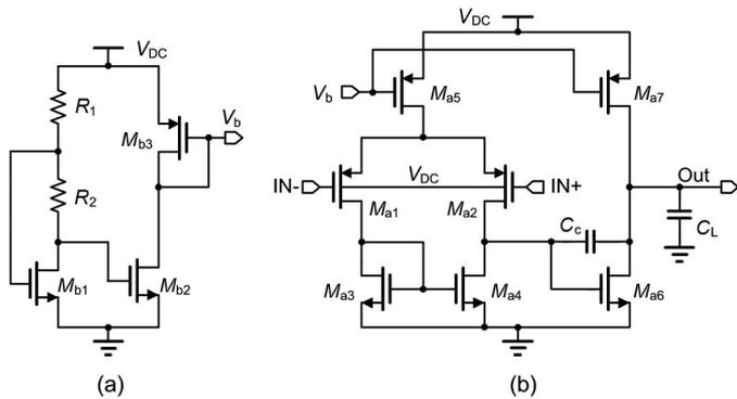
Fig. 11. Schematic of (a) peaking current source; (b) OTA.
