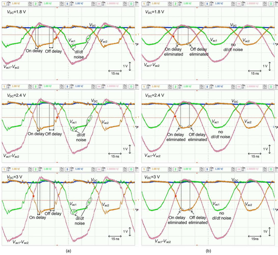
Fig. 18. Measured waveforms of the active rectifier when  $R_L = 500 \Omega$ . (a) Without delay-compensation. (b) With delay-compensation.
