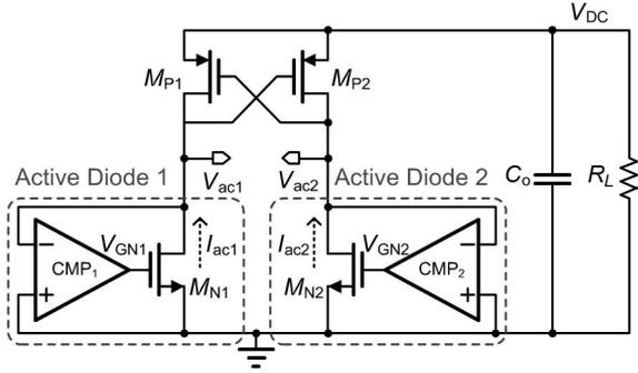
Fig. 2. Schematic of an active rectifier.
