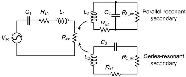
Fig. 3. Simplified equivalent circuit model of the power link.
