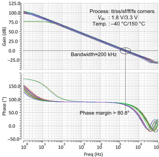
Fig. 16. Bode plots of  $OTA_1$  under different PVT conditions.
