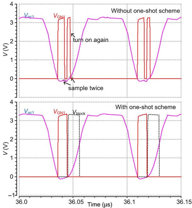
Fig. 10. Simulated waveforms with and without the one-shot scheme.
