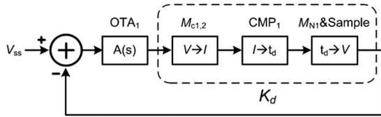
Fig. 15. Small-signal model of the off-delay compensation loop.
