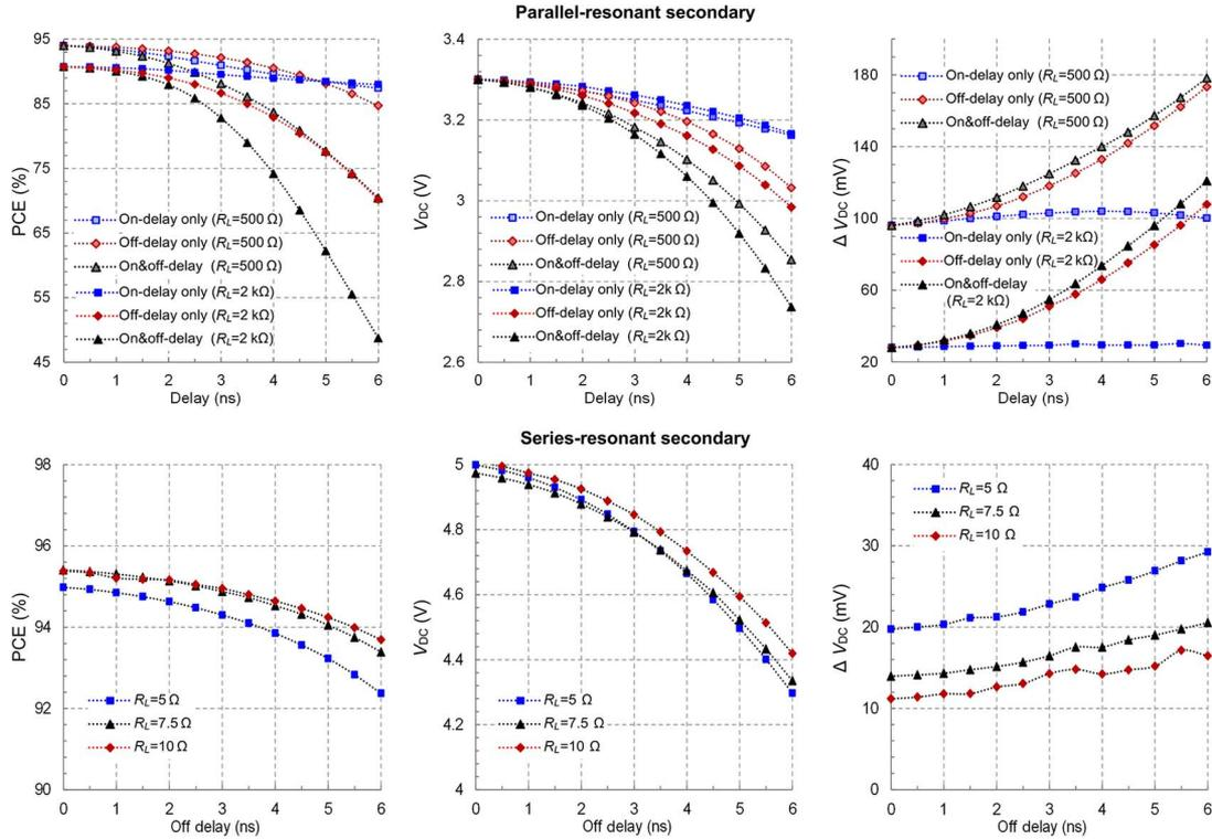
Fig. 5. Effects of on/off delay on the performance of the active rectifiers.
