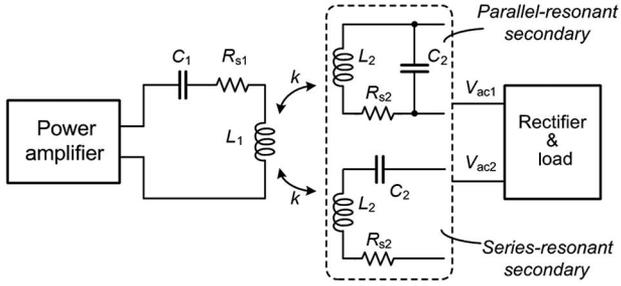
Fig. 1. Power link of an R-WPT system.
