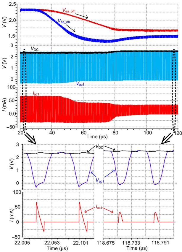
Fig. 8. Simulation results of the proposed technique.
