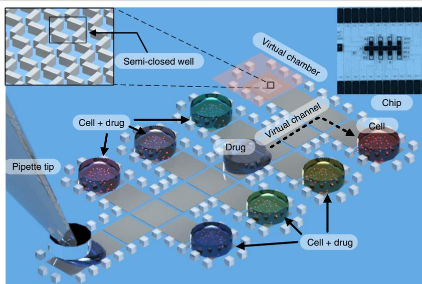
**Fig. 2 Schematic of the DMF chip with virtual channels and virtual chambers for the cell-culture-based drug sensitivity test.** The inset images are the detailed microstructures and the whole picture of the DMF chip
