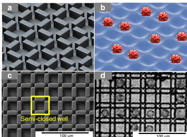
**Fig. 3** The scheme and image results of the microstructure arrays and the corresponding cell trapping results. **a** Microstructures designed on a digital microfluidic chip. **b** The interface formed between the microstructures and promoted single-cell formation. **c** The SEM results of the optimized microstructure arrays, arranged as wall arrays, for trapping single cells. **d** The corresponding results of trapping MDA-MB-231 cells under structures c after 24 h
