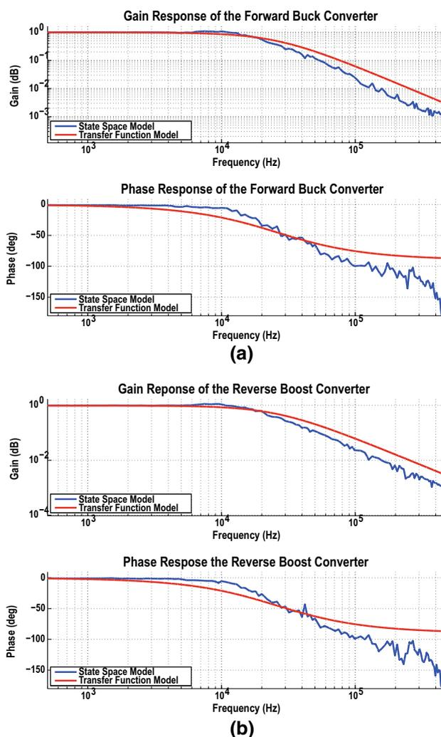
**Fig. 8** Bode plots calculated by state space model and transfer function analysis, for **a** forward buck operation, and **b** reverse boost operation
