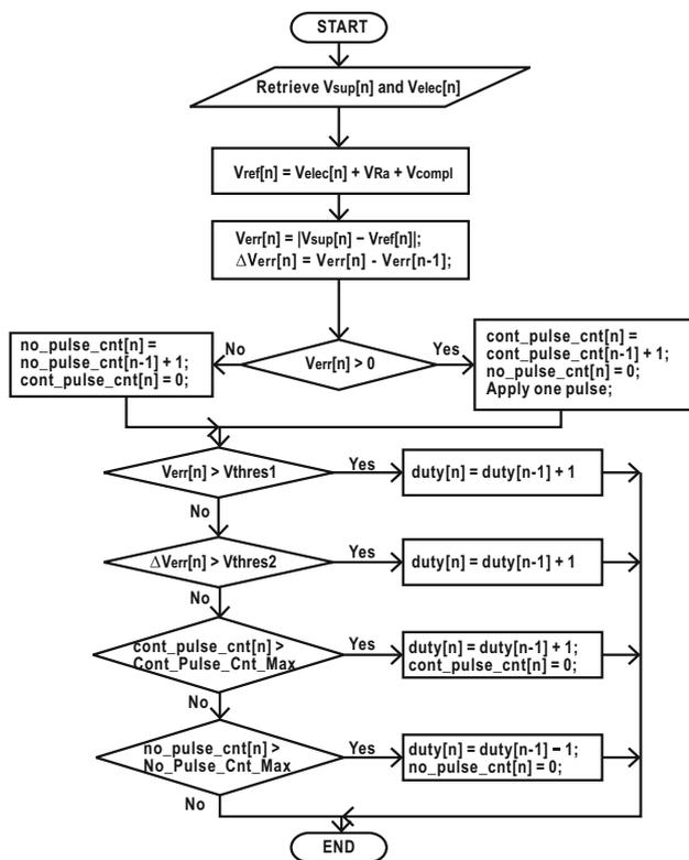
**Fig. 4** Flowchart of the digital pulse-skipping PWM controller with quasi-PID duty update. (Adopted from [8])
