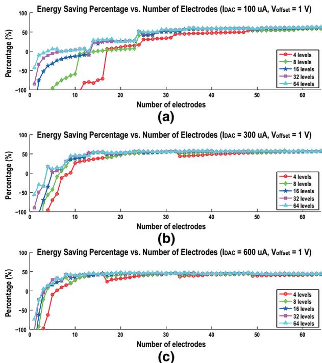
**Fig. 7** Wasted energy saving percentage vs. number of stimulating electrodes for various PT and IESC scaling levels, when **a**  $I_{DAC} = 100 \mu\text{A}$ , **b**  $I_{DAC} = 300 \mu\text{A}$ , and **c**  $I_{DAC} = 600 \mu\text{A}$
