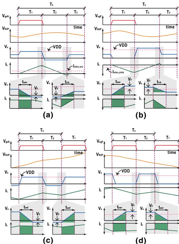
**Fig. 3** Key waveforms during a cycle of the forward-buck conversion phase and the reverse-boost conversion phase. Timing diagram for **a** the DCM forward-buck operation, **b** the DCM reverse-boost operation, **c** the CCM forward-buck operation, and **d** the CCM reverse-boost operation
