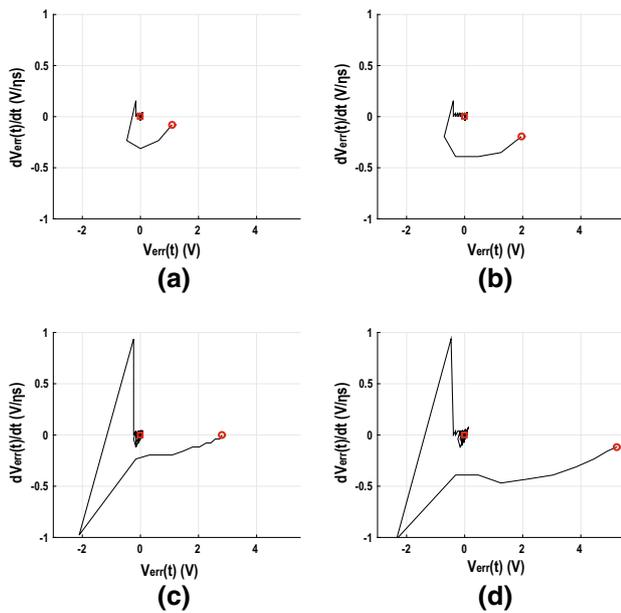
**Fig. 10** Phase portrait plot of the bidirectional SMPS for microstimulator when driving cathodic-first biphasic pulses of **a**  $I_{DAC} = 100 \mu A$  to an electrode during the reverse boost phase, and **b** during the forward buck phase, and when driving **c**  $I_{DAC} = 600 \mu A$  to 64 electrodes during the reverse boost phase, and **d** during the forward buck phase
