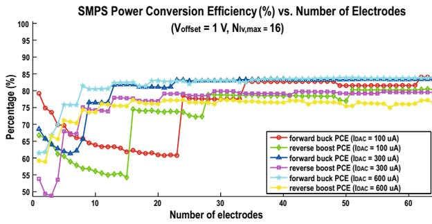
**Fig. 5** Simulated power conversion efficiency of the proposed SMPS calculated during a set of the biphasic stimuli, as  $N_{elec}$  increases from 0 to 64, when  $V_{offset} = 1$  V
