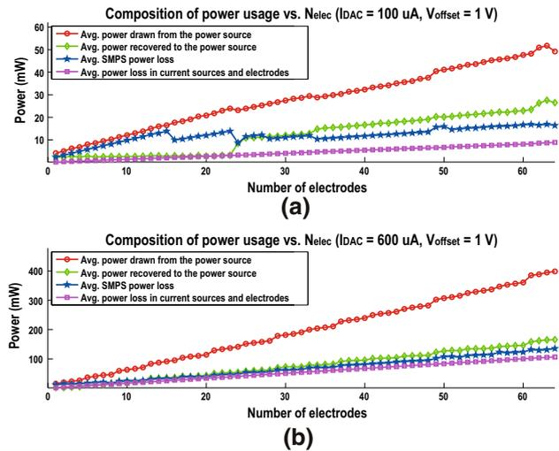
**Fig. 6** Average power compositions pertaining to a set of the biphasic stimuli, as  $N_{elec}$  increases from 0 to 64, when **a**  $I_{DAC} = 100 \mu A$ , and **b**  $I_{DAC} = 600 \mu A$ . The power loss in current sources and electrodes is the average of  $P_{loss,Ra} + P_{loss,CCT}$  during a pair of biphasic stimuli
