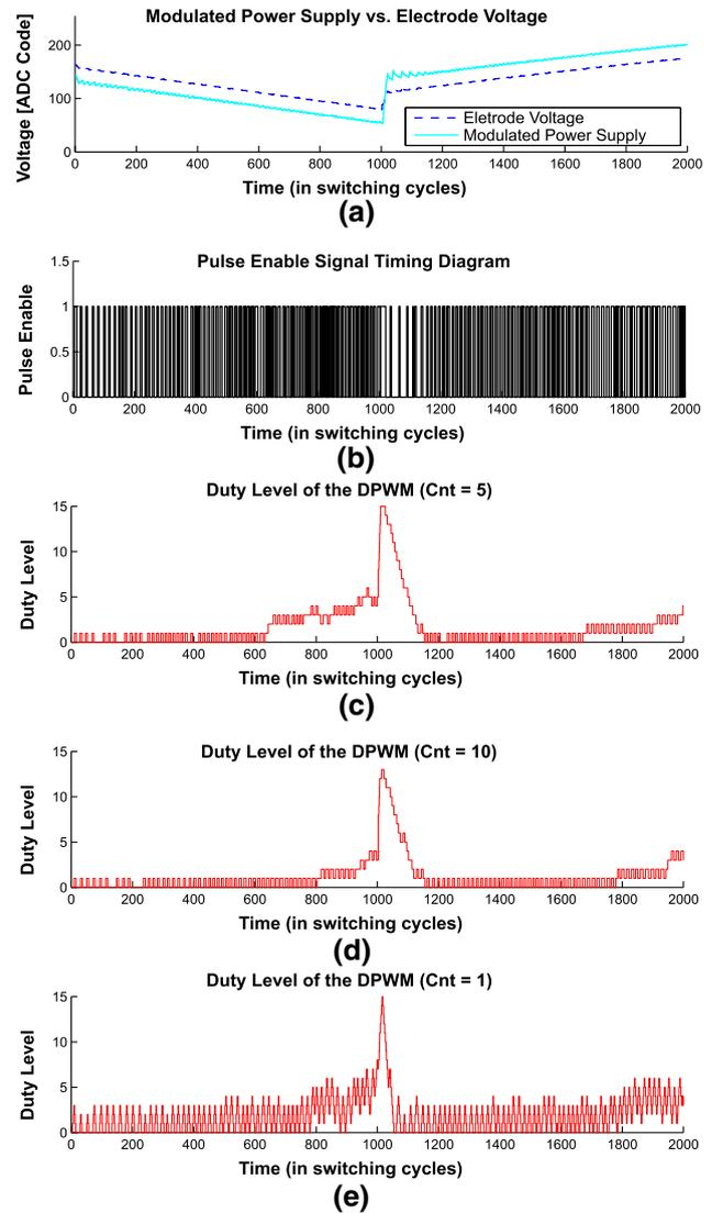
**Fig. 11** Measured duty level dynamics pertaining to various **Cont\_Pulse\_Cnt\_Max** and **No\_Pulse\_Cnt\_Max** values, when  $V_{offset} = 1 V$ ,  $I_{DAC} = 300 \mu A$ , and  $N_{elec} = 16$ . **a**  $V_{elec}$  and  $V_{sup}$  voltage waveforms during a set of biphasic stimulus. **b** Pulse enable signal. **c** Duty level when **Cnt** ( $= \text{Cont\_Pulse\_Cnt\_Max} = \text{No\_Pulse\_Cnt\_Max}$ ) = 5. **d** Duty level when **Cnt** = 1. **e** Duty level when **Cnt** = 10
