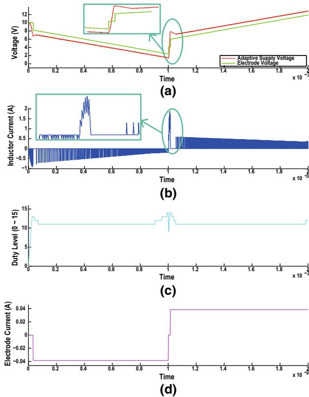
**Fig. 2** Waveforms of the proposed stimulation system during a set of cathodic-first bi-phasic stimulation pulses: waveforms of **a** the voltage at the power supply rail ( $V_{SUP}$ ) and the voltage at the electrode interface ( $V_{elec}$ ). **b** The current flowing through the inductor ( $L_1$ ). **c** The duty cycle command. **d** The total current amplitude flowing through the electrodes array
