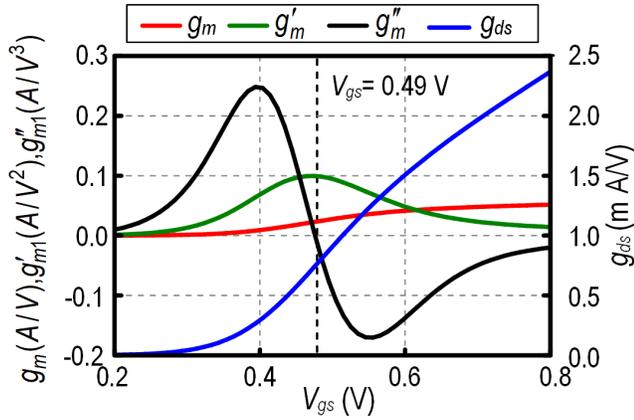
Fig. 2.  $g_m$ ,  $g_{ds}$ ,  $g'_m$ , and  $g''_m$  common-source 80/0.13- $\mu\text{m}$  nMOS transistor. Threshold voltage is about 0.40 V for this device.
