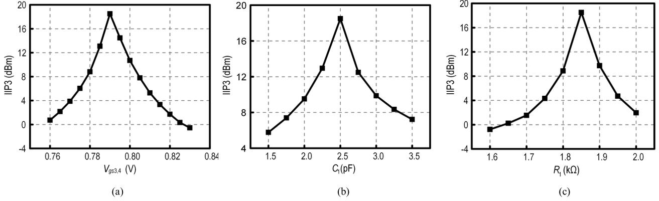
Fig. 12. Simulated plots of (a) IIP3 versus  $V_{gs3,4}$  at constant  $C_1 = 2.5$  pF and  $R_1 = 1.85$  k $\Omega$ , (b) IIP3 versus capacitor  $C_1$  at constant  $V_{gs3,4} = 0.79$  V and  $R_1 = 1.85$  k $\Omega$ , and (c) IIP3 versus resistor  $R_1$  at constant  $V_{gs3,4} = 0.79$  V and  $C_1 = 2.5$  pF.
