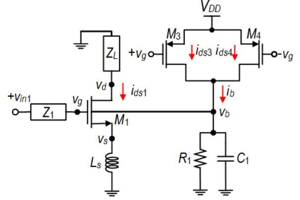
Fig. 9. Thevenin's equivalent half circuit of a combined inductively degenerated common-source transconductance stage and IM2 injection.
