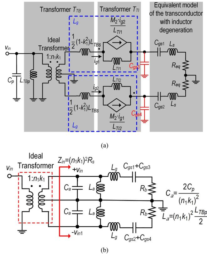
Fig. 5. Schematic showing the proposed differential ISD transconductor with (a) transformer equivalent model of transformer-based balun  $T_{TB1}$  and transformer-based gate inductor  $T_{TI}$  while including input parasitic capacitance. (b) More compact equivalent circuit model of input network for calculating the input impedance by series of parallel-series conversion.
