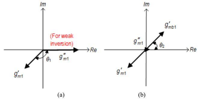
Fig. 11. Vector diagram for the components of  $G_3(\pm\omega_1, \pm\omega_1, \omega_2)$  for (a) conventional ISD transconductor and (b) proposed ISD transconductor.
