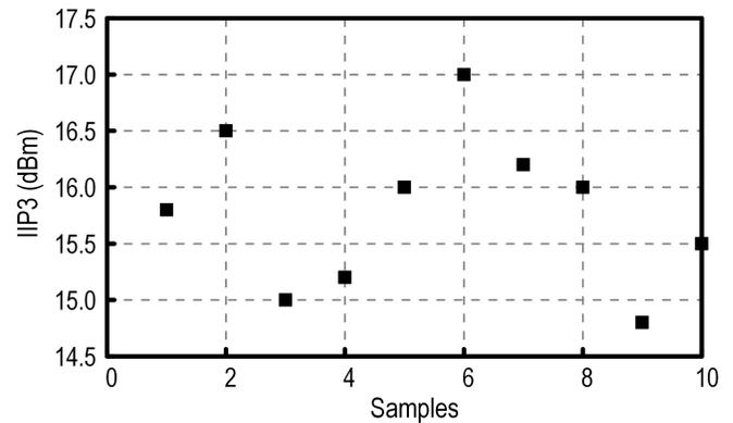
Fig. 18. Measured IIP3 over ten samples.
