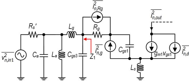
Fig. 8. Noise equivalent half circuit of the input transconductance stage.
