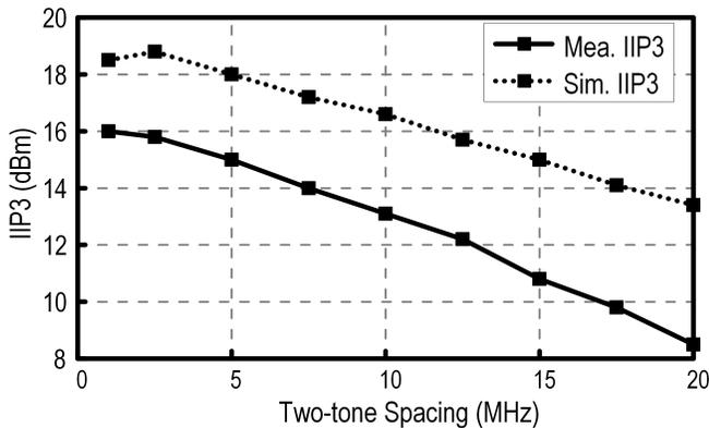
Fig. 17. Measured and simulated IIP3 versus two-tone spacing.
