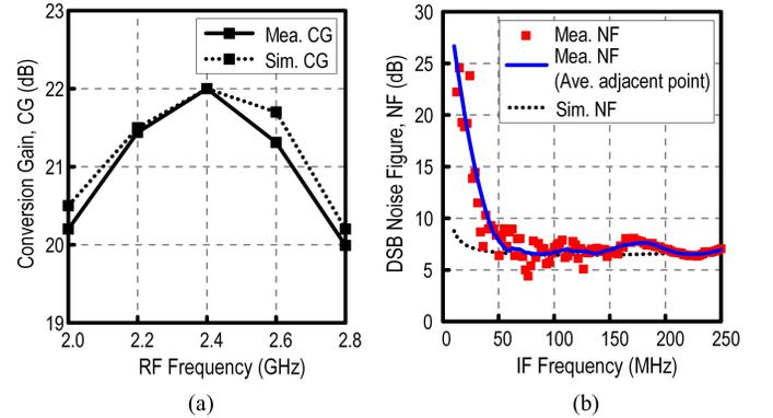
Fig. 15. Measured and simulated (a) CG versus RF frequency and (b) DSB NF versus IF frequency.
