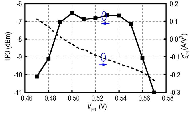
Fig. 10. Simulated IIP3 and  $g''_{m1}$  of the input transistor  $M_{1,2}$  without integrating IM2 circuit relating to its gate-source voltage  $V_{gs1}$ .
