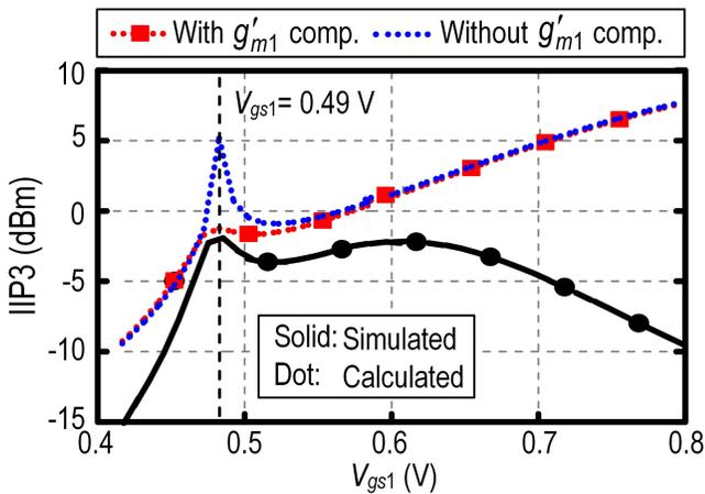
Fig. 3. Simulated and calculated of IIP3 for different values of  $V_{gs1}$ .
