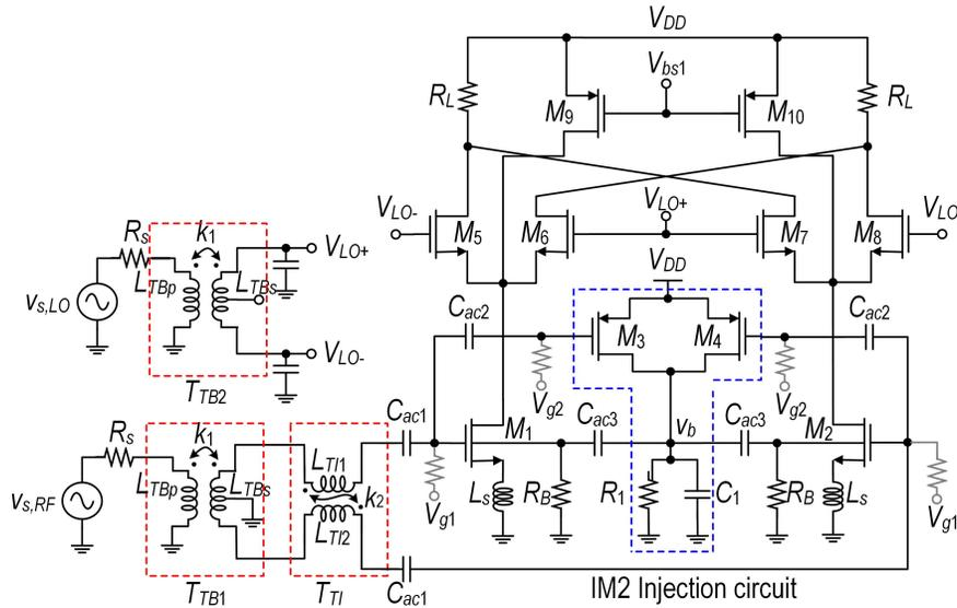
Fig. 4. Circuit schematic of the proposed modified ISD balun-LNA mixer, including an on-chip transformer-based balun and a transformer-based inductor at the input transconductance stage without the output IF buffer and biasing circuits. The three transformers' impedance ratio from the primary to the secondary winding is unity.
