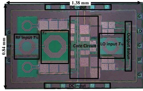
Fig. 13. Microphotograph of the proposed LNA mixer.
