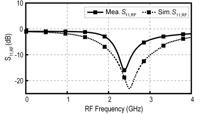
Fig. 14. Measured and simulated of input return loss ( $S_{11}$ ) of the RF port.
