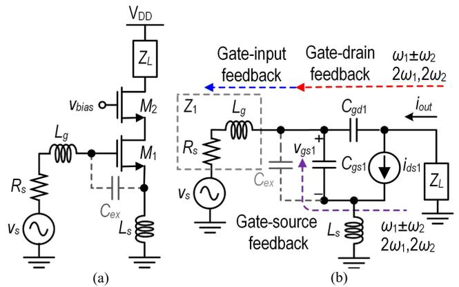
Fig. 1. (a) Schematic and (b) small-signal equivalent circuit of the ISD common-source transconductor with feedback path.
