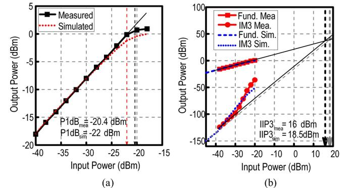
Fig. 16. Measured and simulated (a)  $P_{1dB}$  and (b) two-tone IIP3 results.
