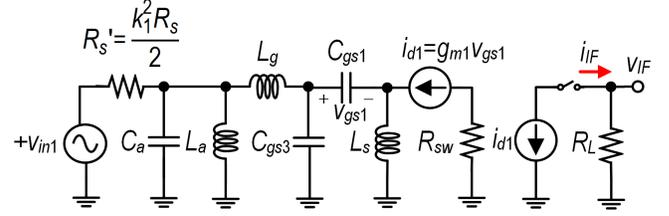
Fig. 6. Half-circuit small-signal representation of the proposed balun-LNA mixer.
