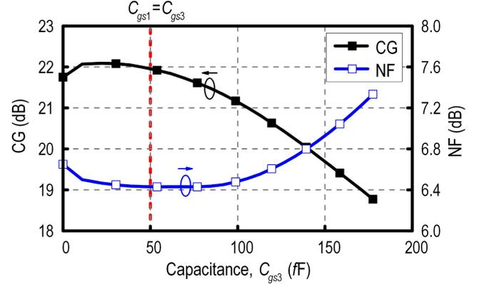
Fig. 7. Simulated CG and NF of the proposed balun-LNA mixer with different transistor size of  $M_{3,4}$ , to demonstrate its effects when  $C_{gs1} \approx 50$  fF.
