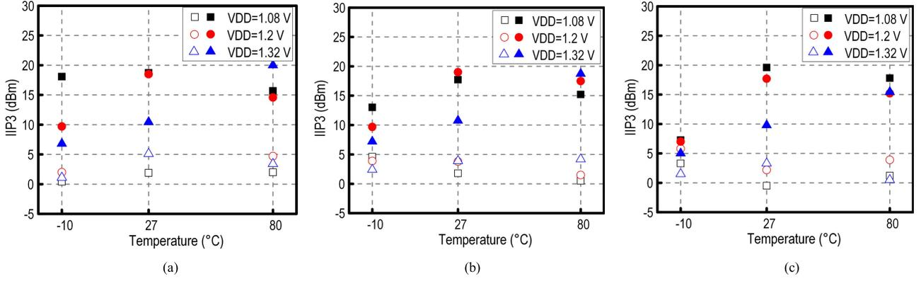
Fig. 19. Simulated IIP3 with PVT variations. (a) Typical corner. (b) Slow–slow corner. (c) Fast–fast corner. The open symbol represents uncalibrated IIP3 and solid symbol represents calibrated IIP3.
