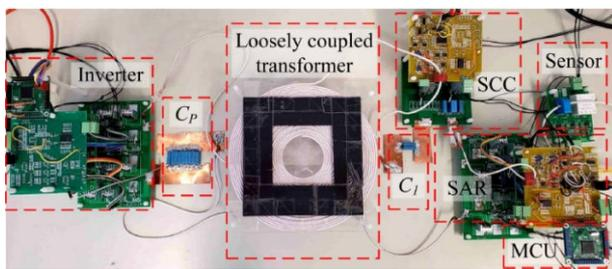
Fig. 2. Experimental Prototype of the proposed CP charging system.
