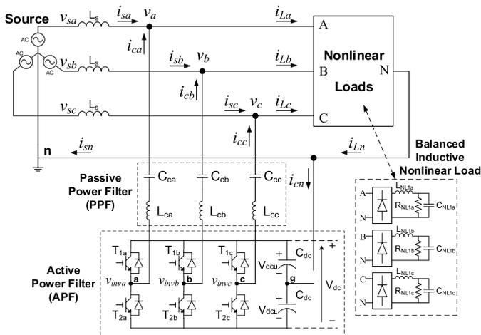
Fig. 1. System configuration of a three-phase four-wire center-split LC-HAPF.
