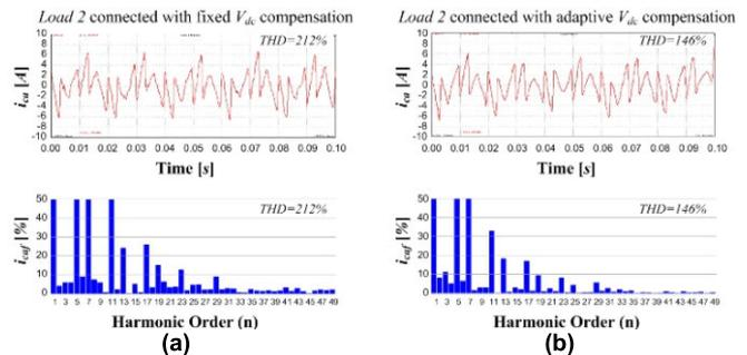
Fig. 2. Experimental  $i_{ca}$  and its frequency spectrum with: (a) fixed  $V_{dc}=60V$  and (b) adaptive  $V_{dc}$  control for Load 2.
