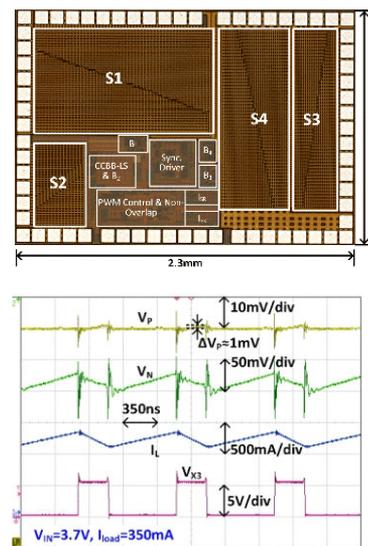
Fig. 2. Chip micrograph, and measured voltage and current waveforms.
