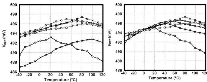
Fig. 2. The measured (a) untrimmed, (b) trimmed  $V_{REF}$  from -40 to 120 °C.
