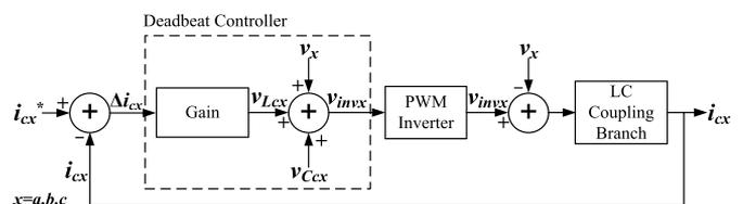
Fig. 2. Control block diagram of deadbeat current controller.
