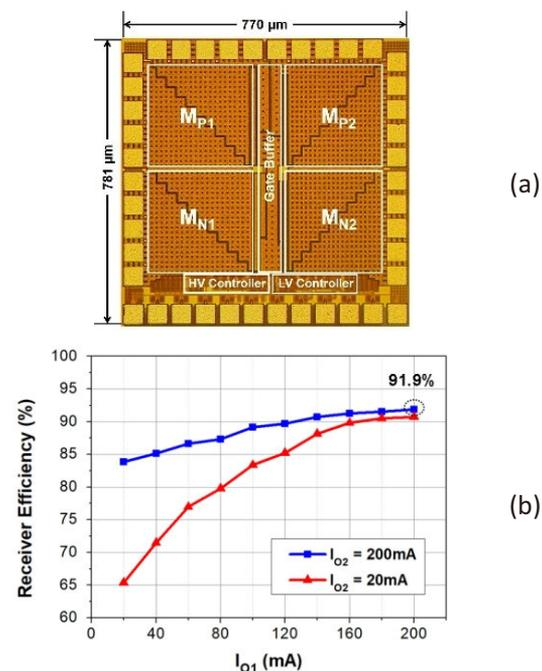
Fig. 2. (a) Chip micrograph, and (b) measured efficiency.
