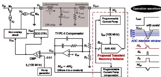
Fig. 1. System block diagram and conceptual waveforms of the proposed buck converter with the SAR assisted transient recovery scheme.
