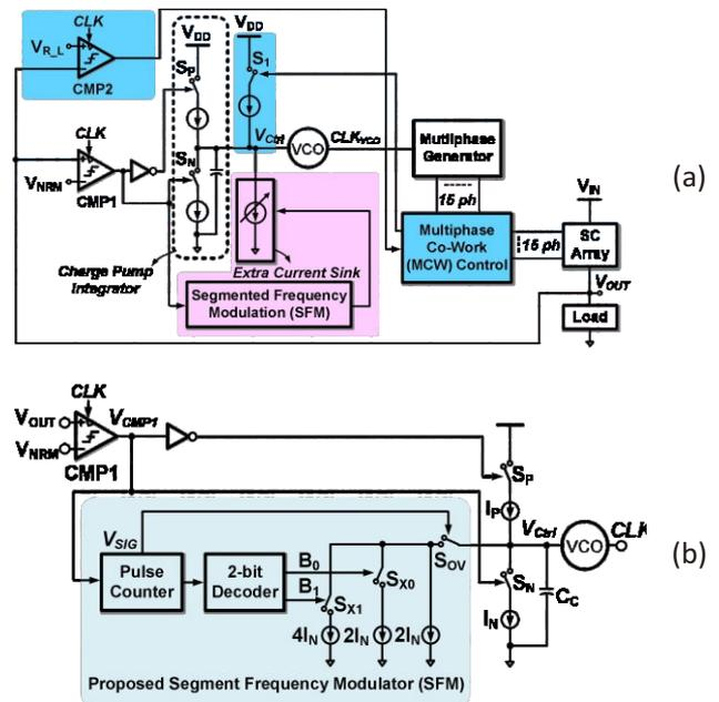
Fig. 1. Block diagram of the proposed Incremental ADC at (a) Linear-Phase and (b) Exponential-Phase.
