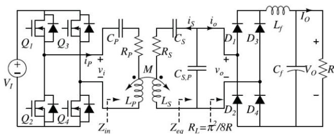
Fig. 1. (a) Schematics and (b) equivalent circuit model of the S/SP IPT converter.
