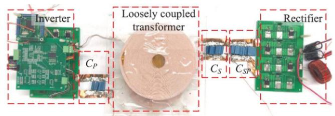
Fig. 2. Experimental Prototype of the S/SP IPT converter.
