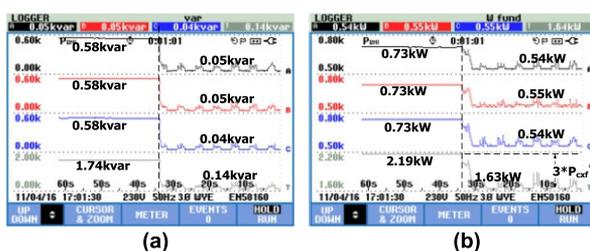
Fig. 3. Dynamic balanced inductive loads compensation by using the HGCI: (a)  $Q_{sxf}$  (reactive power compensation) and (b)  $P_{sxf}$  (active power injection).
