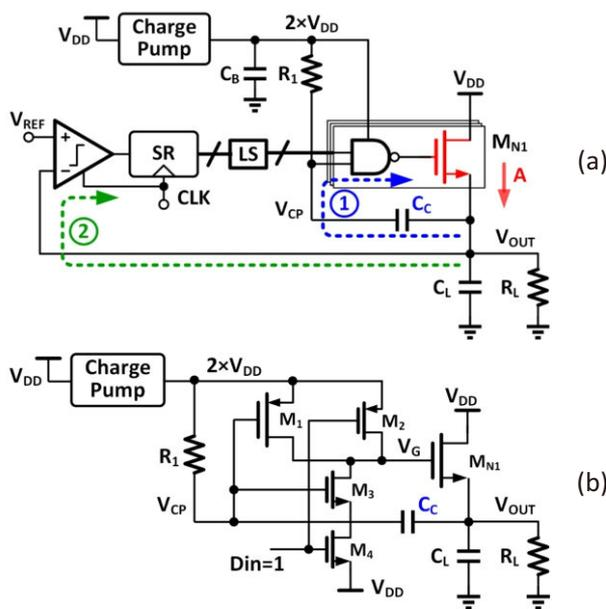
Fig. 1. (a) The proposed NMOS DLDO with NAND-based high-pass analog path, and (b) the Schematic of NAP.
