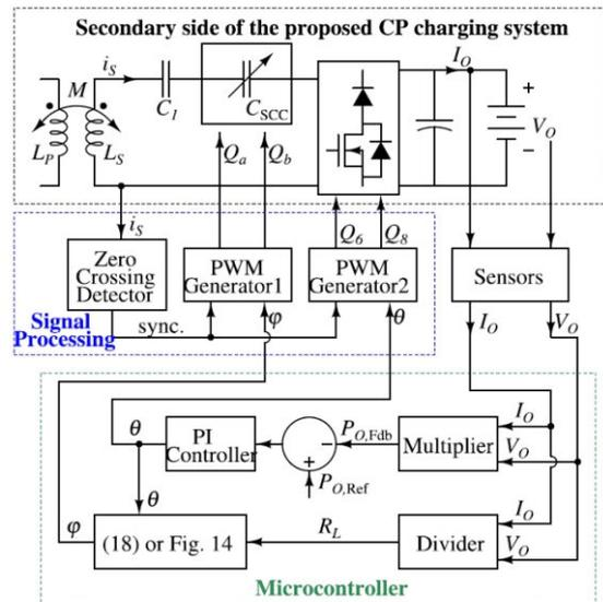
Fig. 3. Secondary load impedance matching control diagram of the proposed CP charging system.
