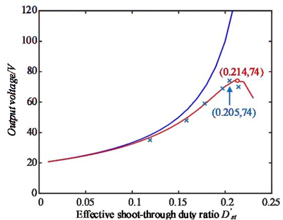
Fig. 3. Comparison of idea lossless, theoretical and experimental results of Trans-Z-source network with  $N_1:N_2=36:12$
