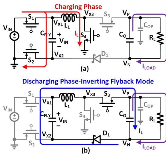
Fig. 1. (a) The charging and (b) the discharging phase of the proposed SIBO converter.
