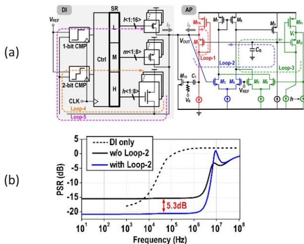
Fig. 1. (a) Schematic of the proposed LDO, and (b) PSR improvement from the replica loop.
