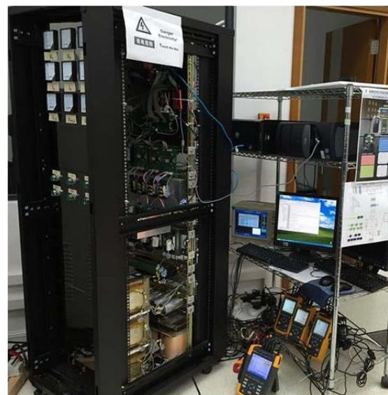
Fig. 2. Experimental setup of the 110V-10A HGCI experimental prototype.
