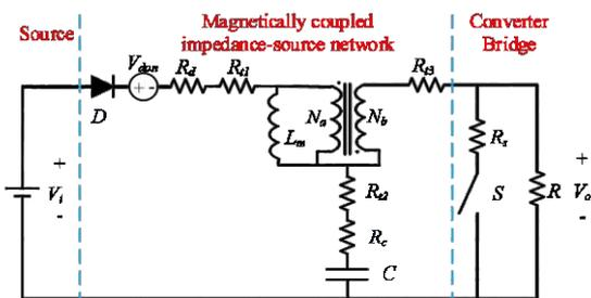
Fig. 1. Equivalent circuit model of magnetically coupled impedance-source converter under parasitic resistances condition
