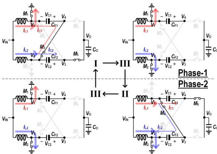
Fig. 1. Proposed convertor working principle.
