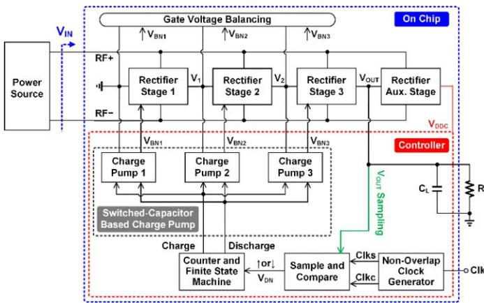
Fig. 1. System overview of the proposed rectifier with active bias tuning.
