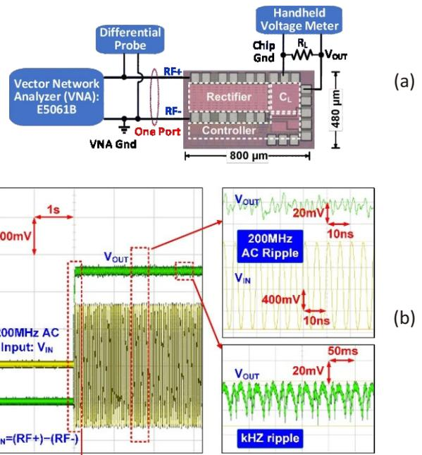
Fig. 2. Chip micrograph, and measured input and output voltage waveforms.
