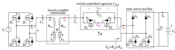
Fig. 1. Schematics of the proposed wireless CP charging system.
