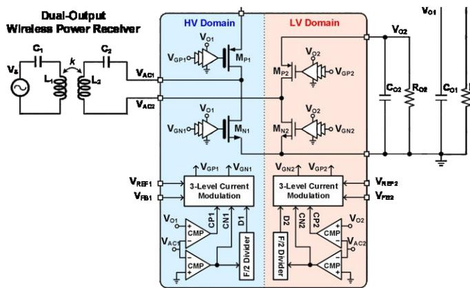
Fig. 1. A wireless power receiver with the proposed dual-output rectifier.
