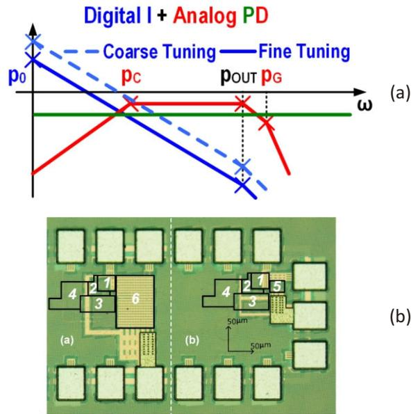
Fig. 2. The frequency responses of the loops, and the die photo of the two proposed design.
