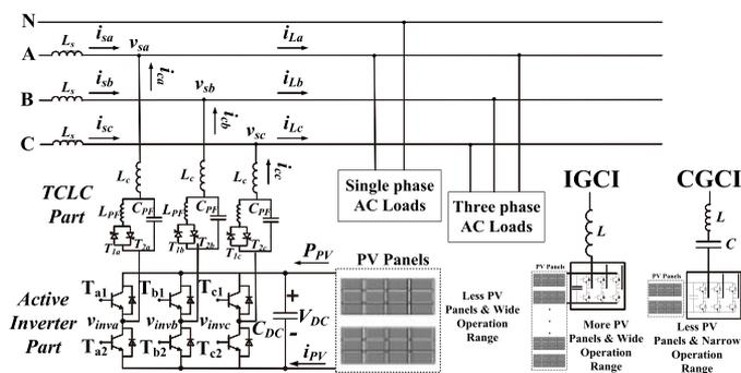
Fig. 1. The structure of the IGCI, CGCI and the proposed HGCI for PV active power injection with power quality conditioning.
