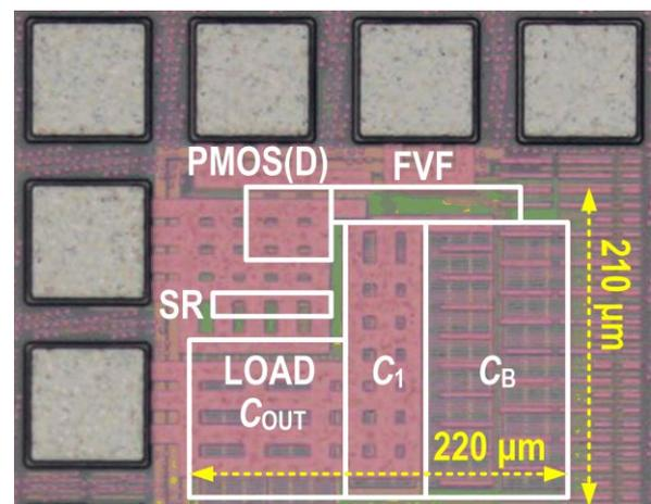
Fig. 2. Chip microphotograph.
