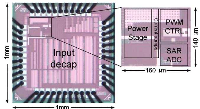
Fig. 2. Chip micrograph.
