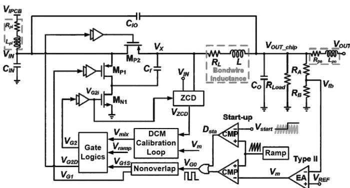
Fig. 1. System block diagram of the proposed fully integrated KY converter under DCM operation.
