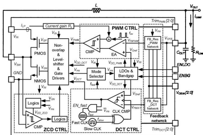
Fig. 1. System block diagram of the proposed DCT/PWM buck converter.
