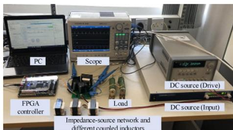
Fig. 2. Experimental prototype of the magnetically coupled impedance-source converter
