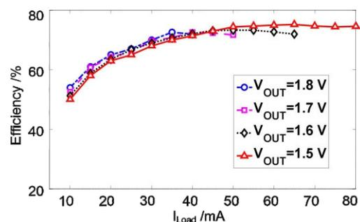
Fig. 3. Measurement power efficiency of the proposed KY converter for  $V_{IN} = 1.2$  V and  $V_{OUT} = 1.5, 1.6, 1.7, 1.8$  V under different load current.
