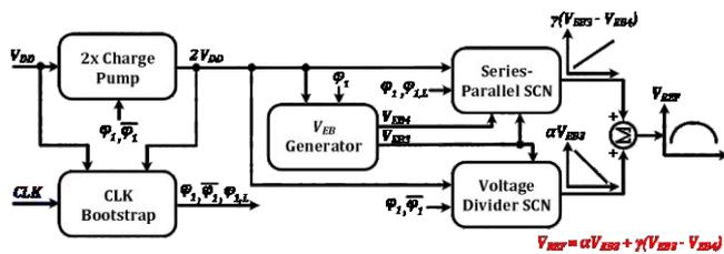
Fig. 1. Architecture of proposed BGR circuit
