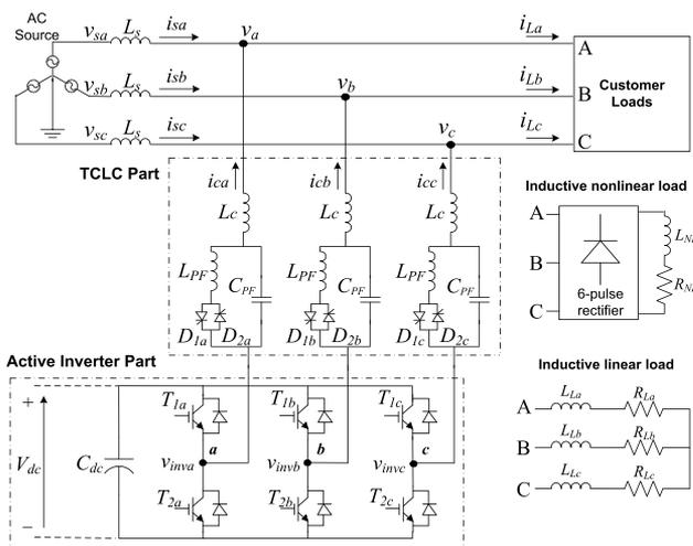
Fig. 1. Circuit configuration of a three-phase three-wire TCLC-HAPF
