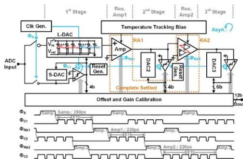
Fig. 1. Overall ADC Architecture and timing.
