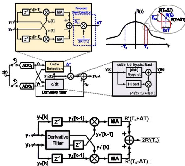
Fig. 1. Proposed fully digital timing mismatch topology based on digital-mixing.
