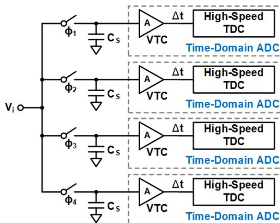
Fig. 1. Overall ADC Architecture and timing
