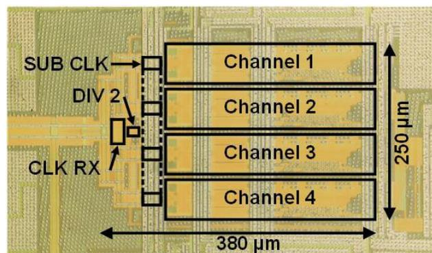
Fig. 2. Chip micrograph.
