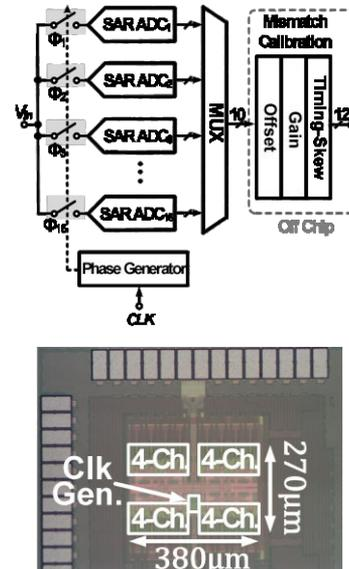
Fig. 2. Block diagram and chip micrograph of 16-way TI ADC.
