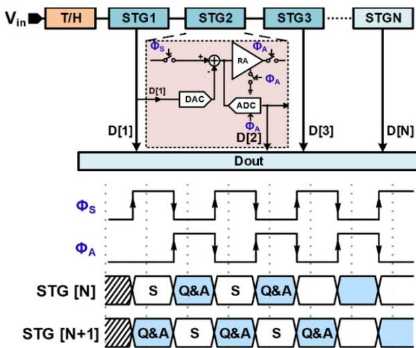
Fig. 1. Overall ADC Architecture and timing.
