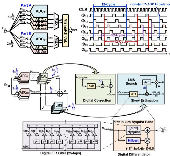
Fig. 1. The architecture and timing skew mismatch calibration of a 3/4-way split TI ADC
