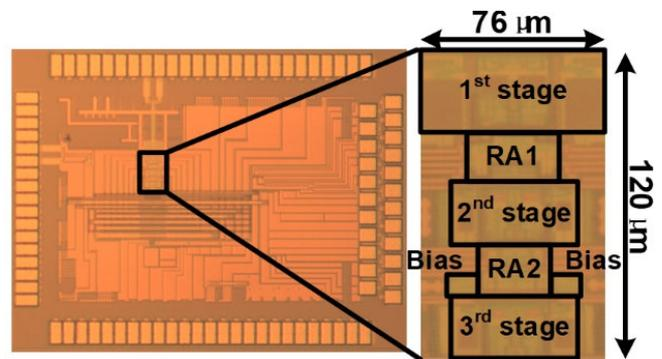
Fig. 2. Chip micrograph.
