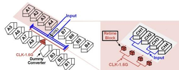
Fig. 2. Block diagram and chip micrograph of 7/8-way split TI ADC.
