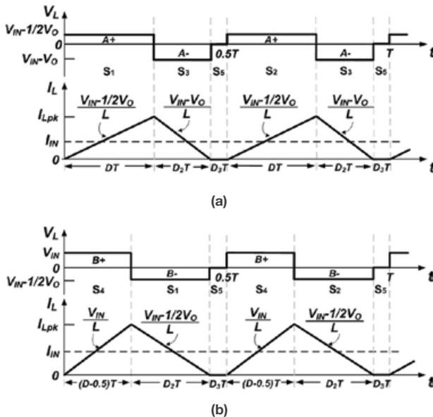
Fig. 2. 3LB converter idealized  $V_L$  and  $I_L$  waveforms for DCM: (a) when  $0 < D < 0.5$  and (b) when  $0.5 < D < 1$ .
