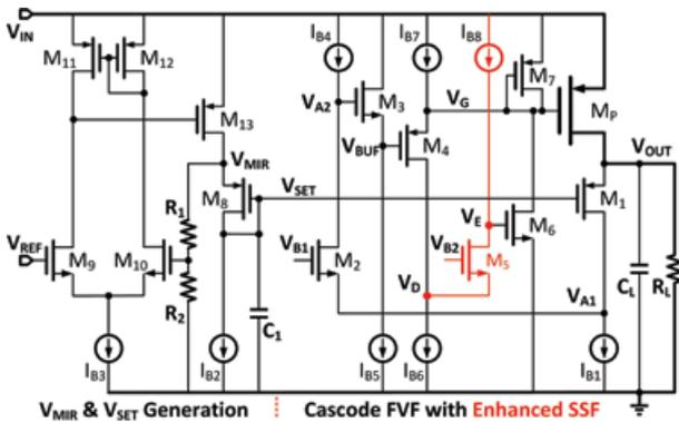
Fig. 1. Schematic of the proposed LDO with enhanced super source follower.
