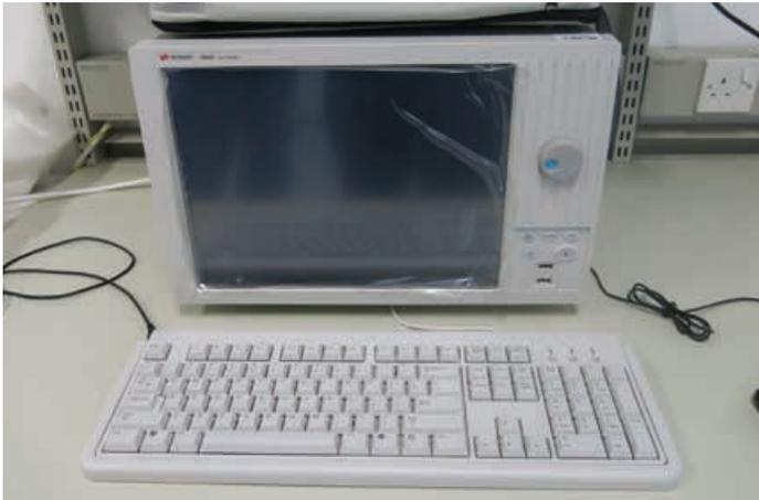
Keysight 16802A 68 channel, 4 GHz timing, 250 MHz state Logic Analyzer
