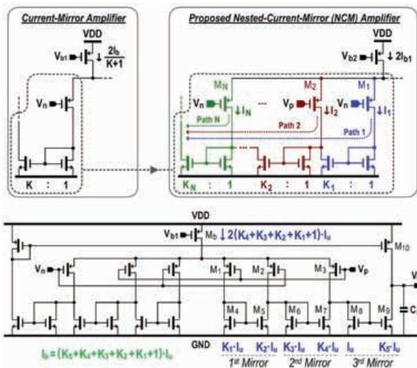
Fig. 1. Development of the NCM amplifier (top) and schematic of the 3-step NCM amplifier (bottom).
