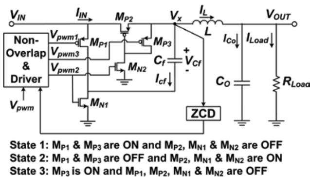
Fig. 1. Proposed KY converter IC topology for DCM.
