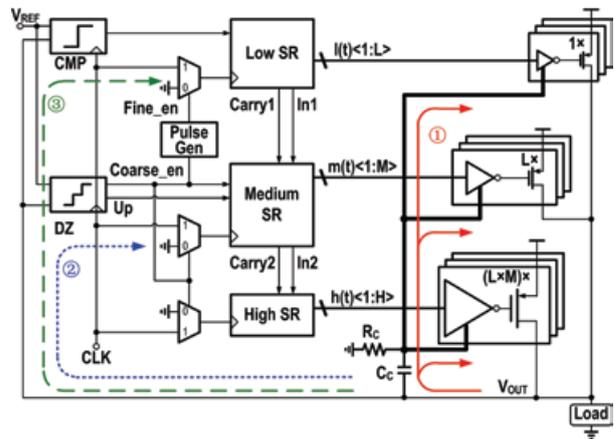
Fig. 2. Overall architecture of the proposed AA-DLDO, with the AA, coarse tuning, and fine tuning loops.
