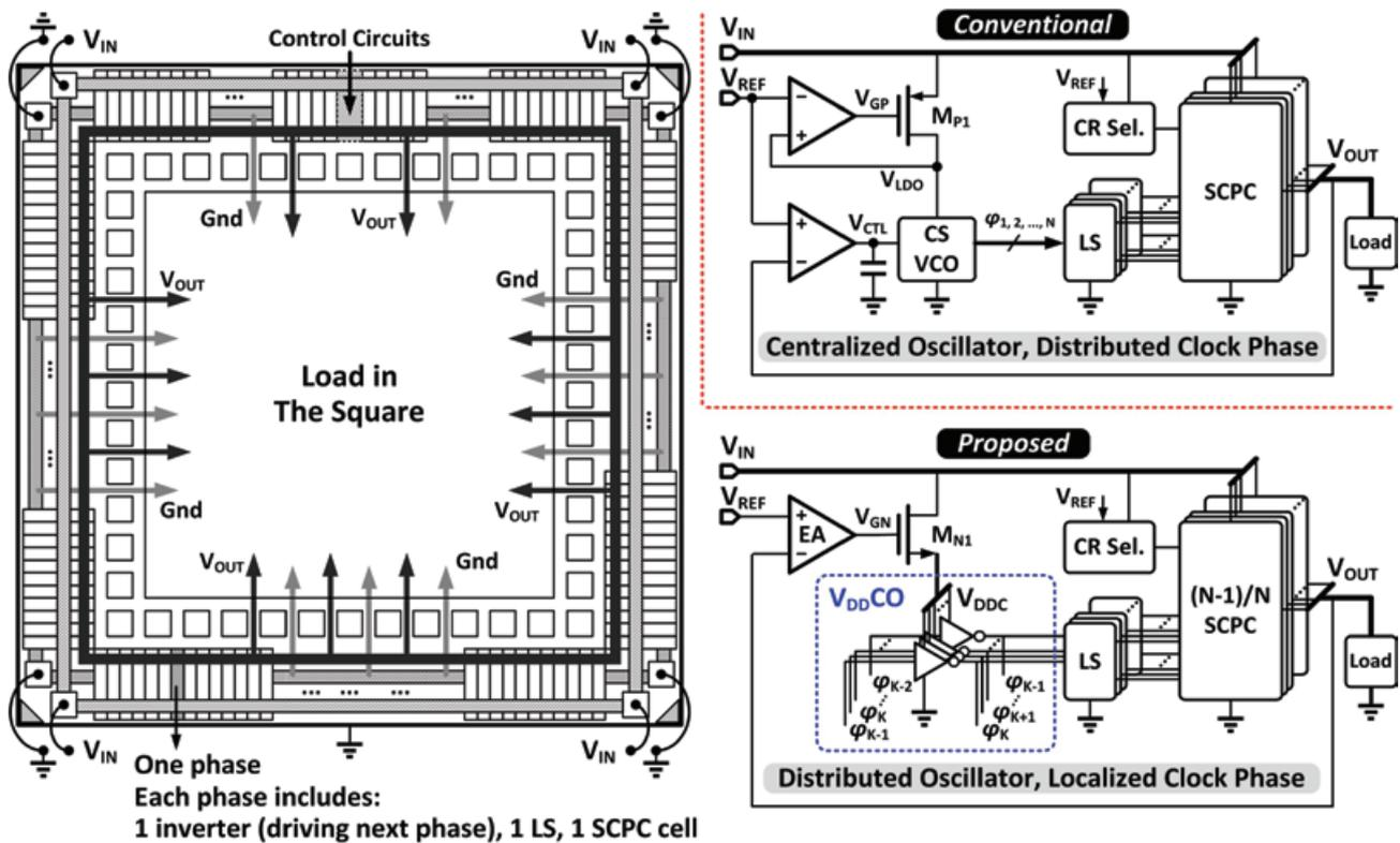
Fig. 1. Conceptual layout of the 100+ phases converter-ring for microprocessors; and the proposed system architecture with the  $V_{DD}CO$  and the (N-1)/N SCPC.
