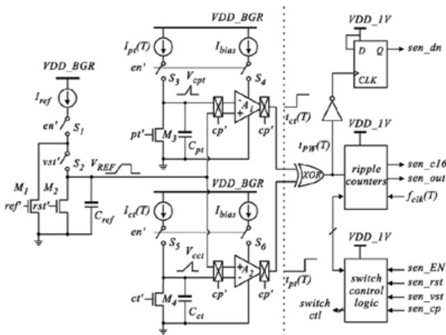
Fig. 1. Implementation of the proposed temperature sensor core.
