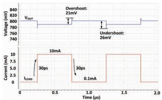
Fig. 2. Simulated load transient response of the LDO with 1.2 V input voltage and 1.0 V output voltage with voltage positioning.
