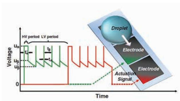
Fig. 1. Profiles of the electrode-driving signal, Natural Discharge after Pulse (NDAP), for a droplet moving across two electrodes. The high-voltage  $u_\alpha$  (HV) period lasts a period of  $t'$ . The low-voltage (LV) period includes multi-cycles of natural discharges ( $t_\beta$ ) and DC pulse ( $t_\alpha$ ).  $u_\beta$  is the instantly decreased voltage when disconnecting an electrode.  $u'$  is the lowest voltage to maintain the movement of a droplet.
