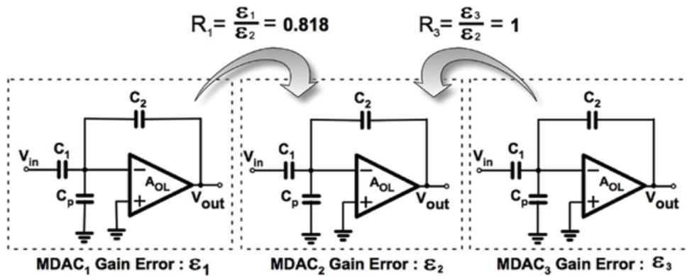
Fig. 1. Gain error ratios tracking between each MDAC.
