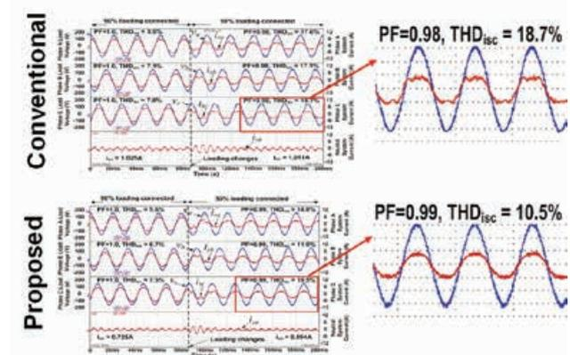
Fig. 2. Experimental compensation performance during loading changes by using conventional digital controller and proposed mixed signal controller.
