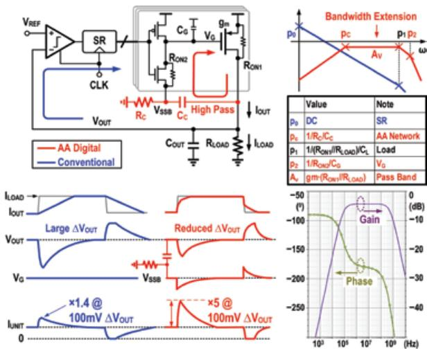
Fig. 1. AA-DLDO scheme and the poles of the AA loop; the transient waveforms of the AA and conventional schemes; and, the Bode plot of the AA loop.
