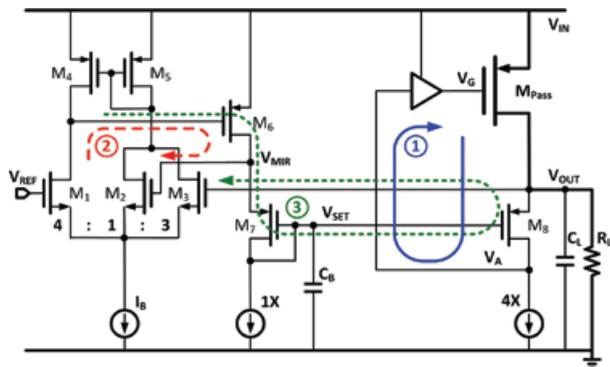
Fig. 1. Schematic of the proposed fully integrated tri-loop LDO.
