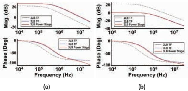
Fig. 4. Boost converter and 3LB converter open-loop bode plot for DCM: (a) When  $D=0.3$  and (b) When  $D=0.7$ .
