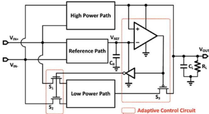
Fig. 1. System architecture of the dual-path rectifier.
