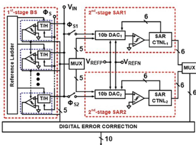
Fig. 1. ADC architecture.
