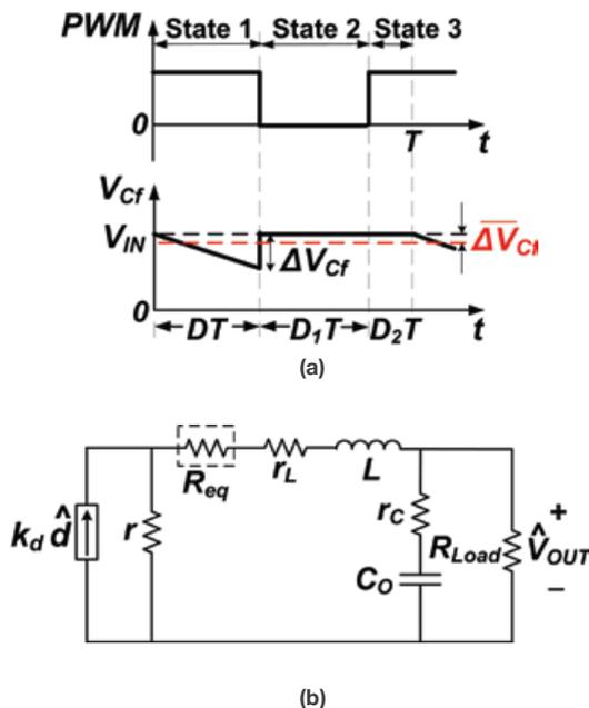
Fig. 3. Small signal model of KY converter for DCM: (a) Flying capacitor voltage  $V_{cf}$  deviation phenomenon and (b) Small signal model with  $V_{cf}$  deviation.
