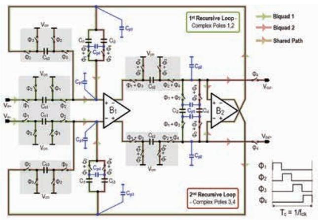
Fig. 1. 1x-recycling SC-buffer Biquad that is equivalent to a 4<sup>th</sup>-order Butterworth LPF.
