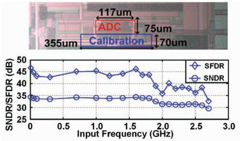
Fig. 1. The ADC architecture, the Chip Photograph and Dynamic Performance.
