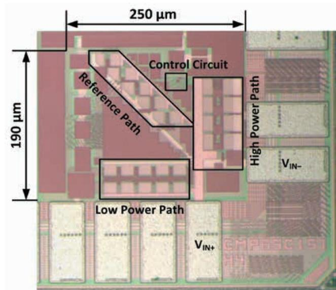
Fig. 2. Chip micrograph of the proposed dual-path rectifier.
