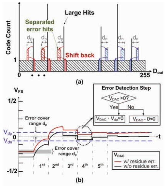
Fig. 2. (a) Code histogram of an 8b example with reference error. (b) Signal behavior of the DAC's output.
