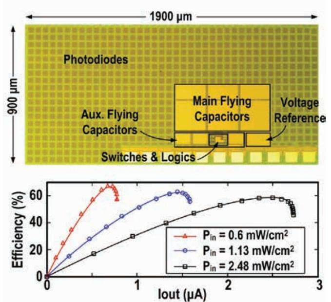
Fig. 2. Chip micrograph (top) and measured efficiency under different incident power levels (bottom).
