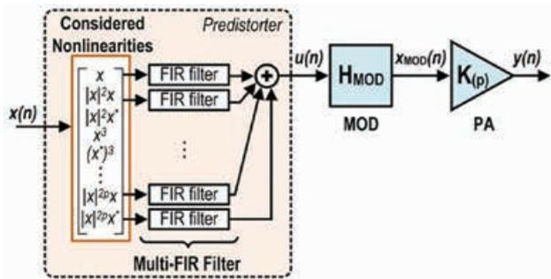
Fig. 1. Block schematic of the DPD addressing both CIM, I/Q imbalance, and RF nonlinearities.
