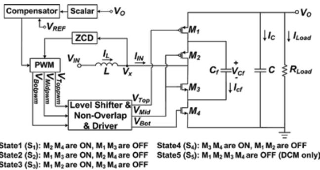
Fig. 1. Proposed 3LB converter IC topology for DCM.
