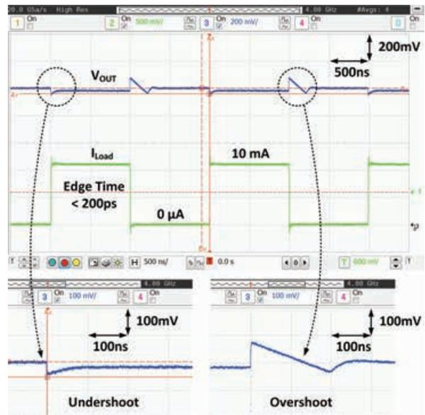
Fig. 2. Measured transient response with  $V_{IN} = 1.2$  V,  $V_{OUT} = 1.0$  V, and on-chip loading change from 0  $\mu$ A to 10 mA within edge times of 200 ps.
