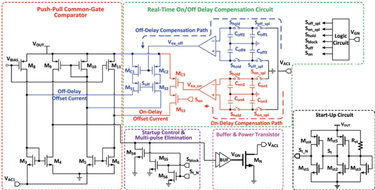
Fig. 1. Schematic of the active diode with the proposed adaptive on/off delay-compensation technique.
