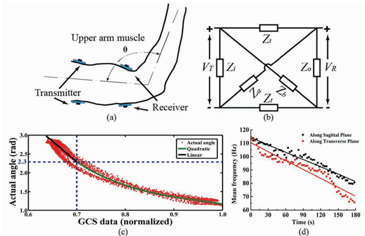
Fig. 1. (a) Schematic of the galvanic couple system on upper arm muscles; (b) Equivalent circuit model of upper arm; (c) Analysis of the curve fitting between GCS data and EJA; (d) Muscle fatigue during forearm movement (for 2 kg load).
