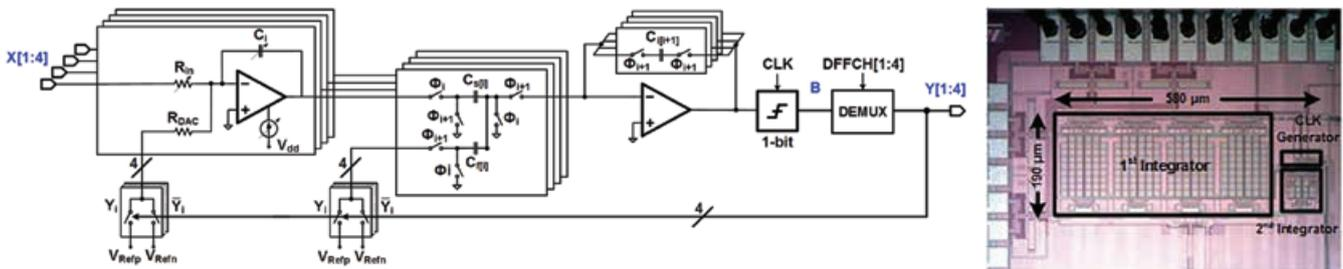
Fig. 1. The Multi-Channel Front-End Architecture and Chip Photograph.
