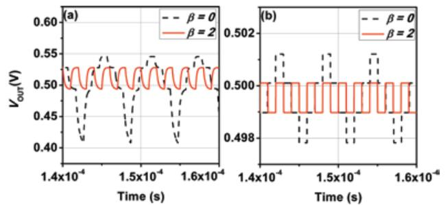
Fig. 2. Simulated results of the proposed D-LDO in  $\beta = 0$  and 2 cases, with (a) 0.5- and (b) 20-mA load currents, at  $F_s = 1$  MHz and  $V_{REF} = 0.5$  V.
