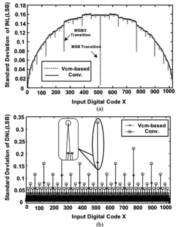
Fig. 2. Behavioral simulation comparing the DNL and INL of conventional and  $V_{cm}$ -based 10-b SAR ADCs.
