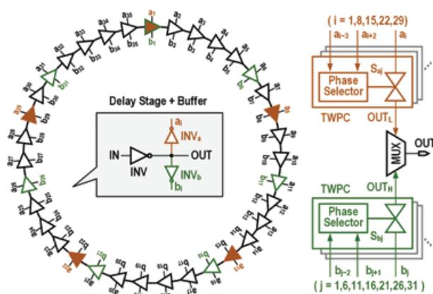
Fig. 1. Schematic of the proposed 35-stage dual-mode TI-RVCO.
