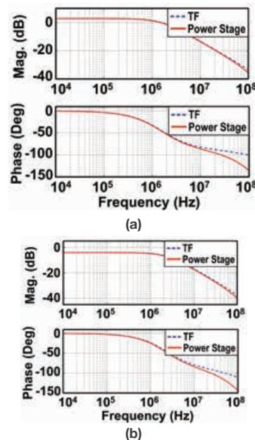
Fig. 4. KY converter open-loop bode plot for DCM: (a) When  $D=0.3$  and (b) When  $D=0.5$ .
