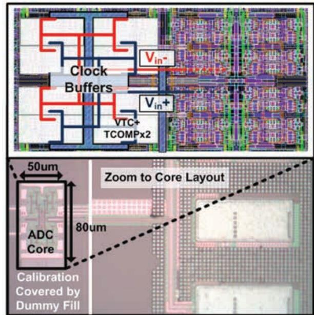
Fig. 2. Chip microphotograph and layout view.
