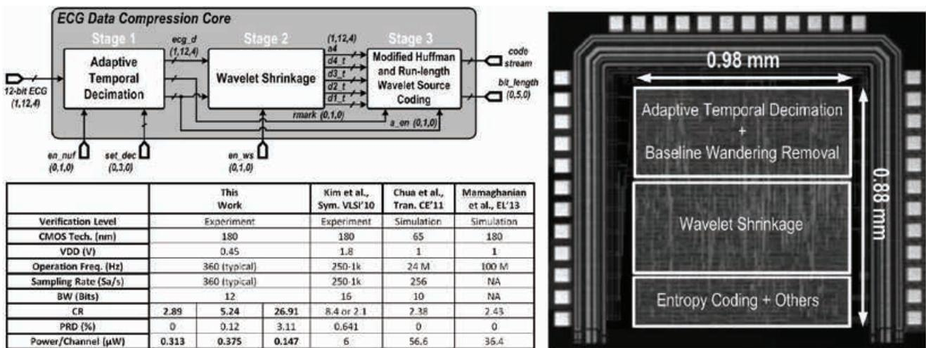
Fig. 1. Proposed ECG compression processor architecture (top left). Chip photograph (right). Performance comparison with state-of-the-art (bottom left).
