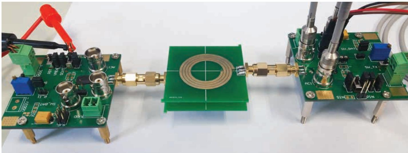
Measurement setup of a reconfigurable bidirectional wireless power transceiver system.
