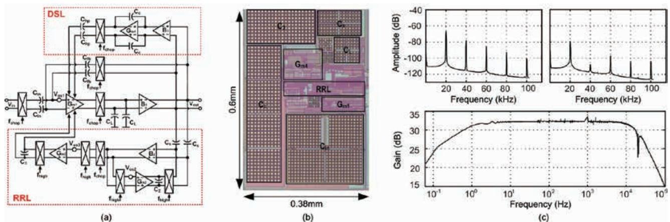
Fig. 1. (a) The proposed chopper-stabilized CCIA topology. (b) Chip photograph. (c) Measured output spectrum and transient waveform of the CCIA with  $f_{chop}=20$  kHz and  $f_{high}=20$  kHz (top left),  $f_{chop}=20$  kHz and  $f_{high}=80$  kHz (top right), and measured frequency response of the complete CCIA (bottom).
