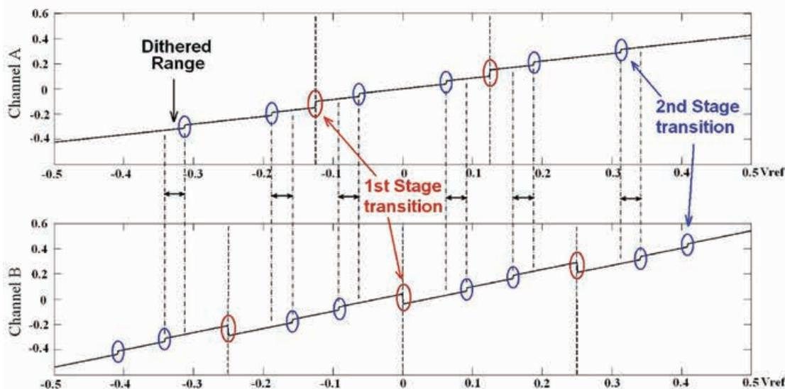
Fig. 1. Proposed Dithered ADC Transfer Characteristics.
