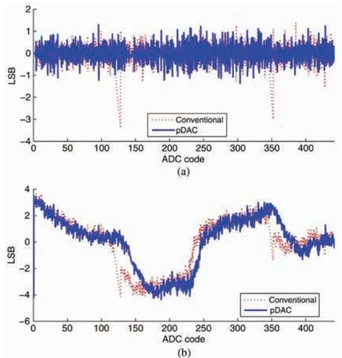
Fig. 2. (a) DNL and (b) INL of the 9 b SAR ADC.
