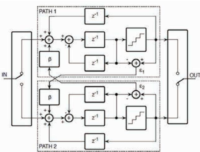
Fig. 1. A 2nd order band-pass polyphase sigma-delta ADC.
