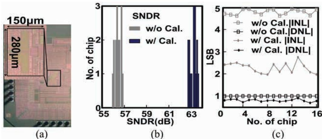
Fig. 2. (a) Chip photograph of SAR ADC. (b) Measured SNDR of total 16 chips. (c) Measured DNL and INL of total 16 chips.
