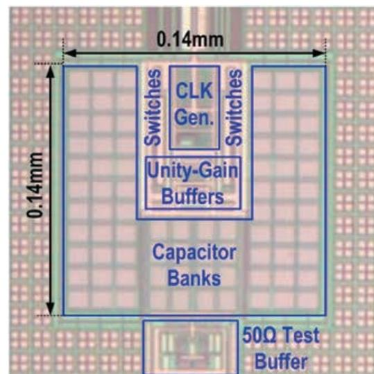
Fig. 2. Chip micrograph.
