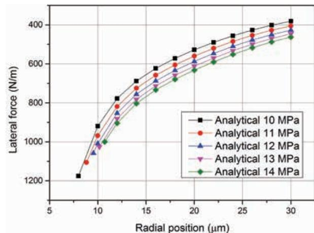
Fig. 2. Modeling results of the lateral force for the large deflection membranes in collapse mode.
