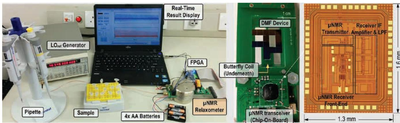
Experimental setup of a nuclear magnetic resonance (NMR)-digital microfluidic system.
