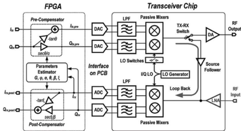
Fig. 1. CMOS TRX chip co-designed with an FPGA implementing the proposed calibration algorithm.
