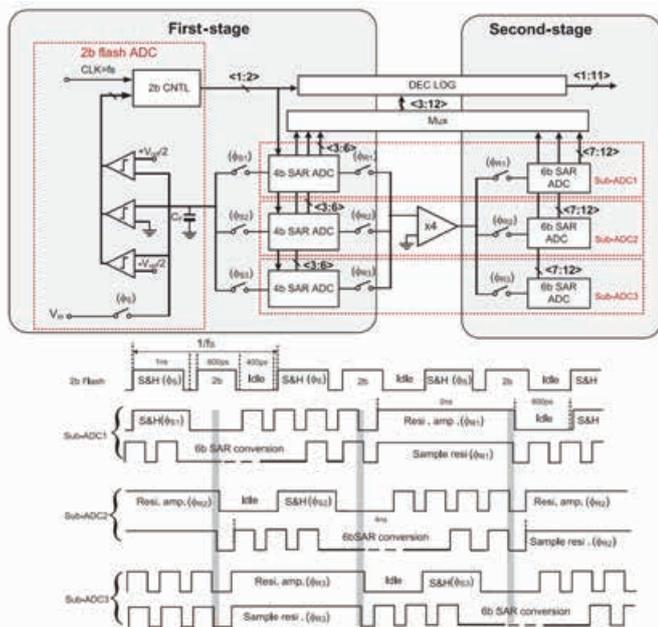
Fig. 1. Overall ADC architecture and its timing diagram.
