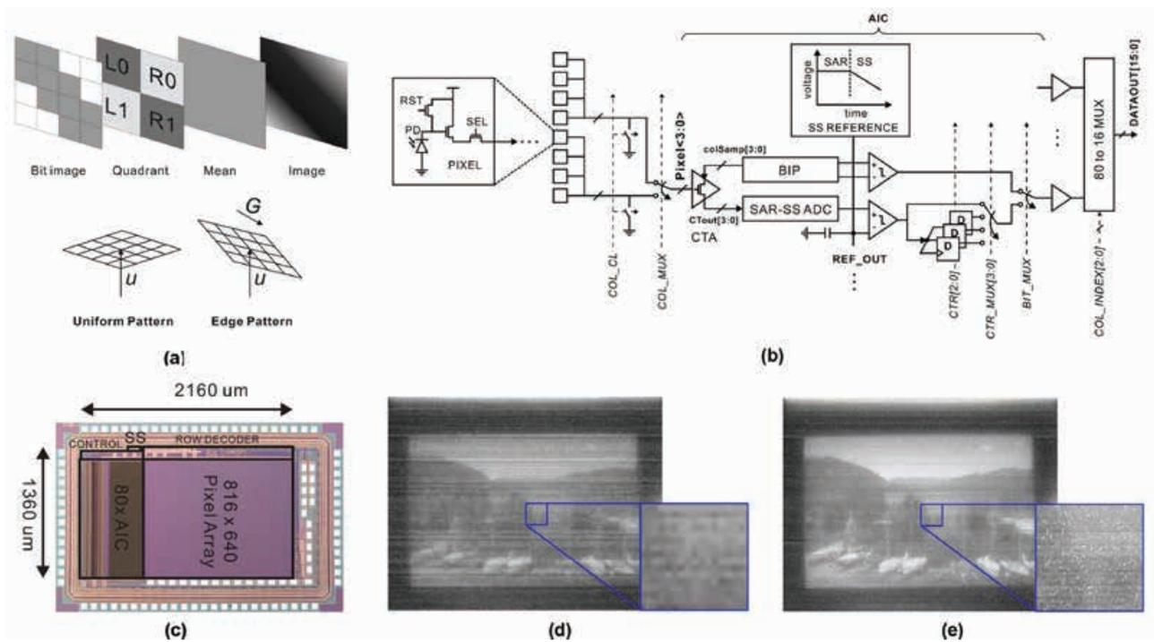
Fig. 1. (a) Components used in the image compression algorithm. (b) Column circuit: from pixel to AIC. (c) Chip micrograph. (d) Image captured from the chip prototype in compression mode. (e) Image captured in raw mode.
