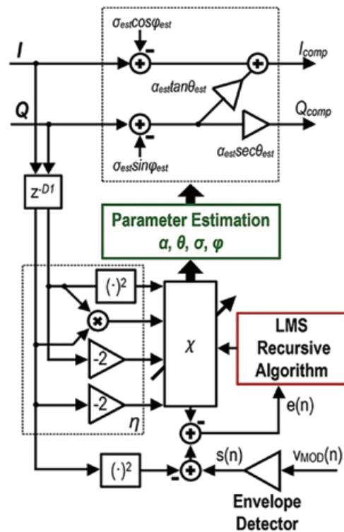
Fig. 2. Block diagram of the digital I/Q-LOFT calibration.
