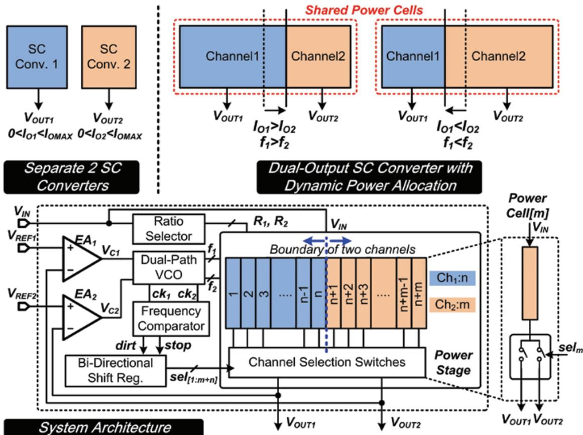
Fig. 1. Strategy of dynamic power-cell allocation and system architecture of proposed dual-output SC converter.
