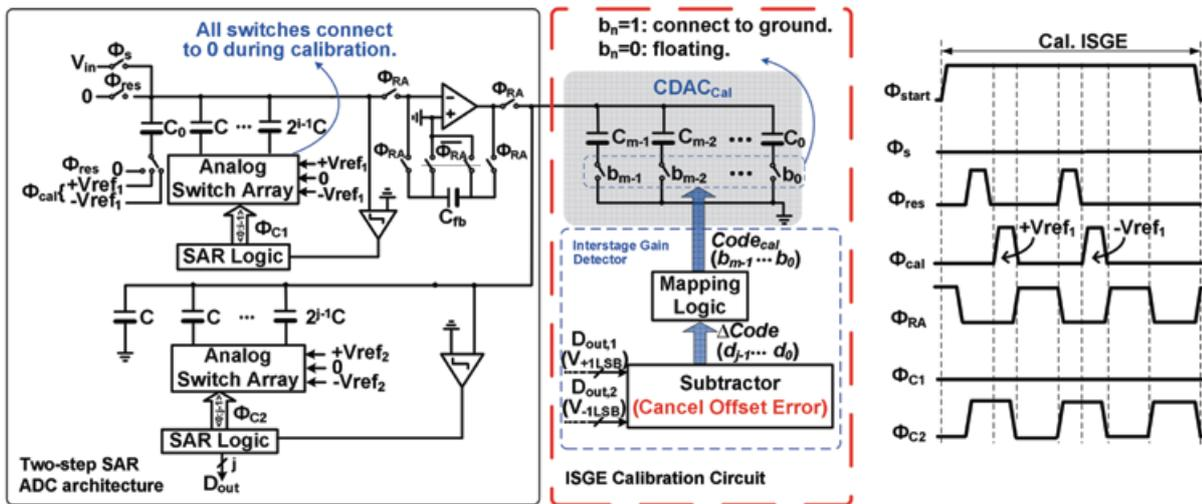
Fig. 1. Two-step SAR ADC with the ISGE calibration and timing diagram.
