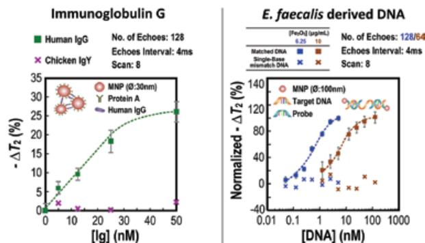
Fig. 2. Experimental results from the detection of Human IgG and synthesized DNA from *E. faecalis*.
