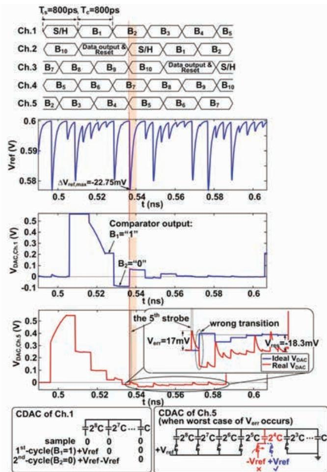
Fig. 1. The worst case of reference ripples in the TI-SAR ADC.
