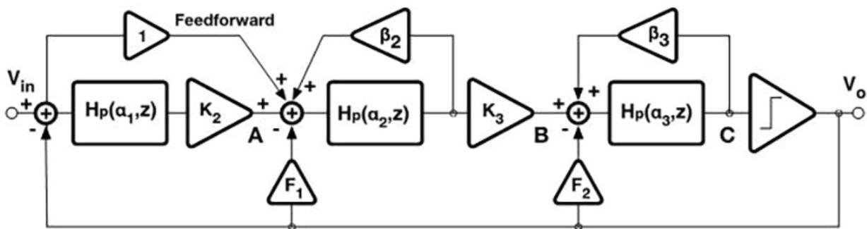
Fig. 1. ADC architecture.
