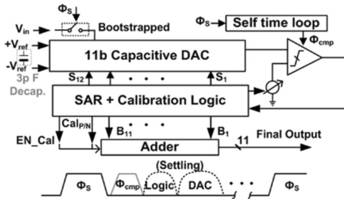
Fig. 1. ADC Architecture (actual implementation is in differential).
