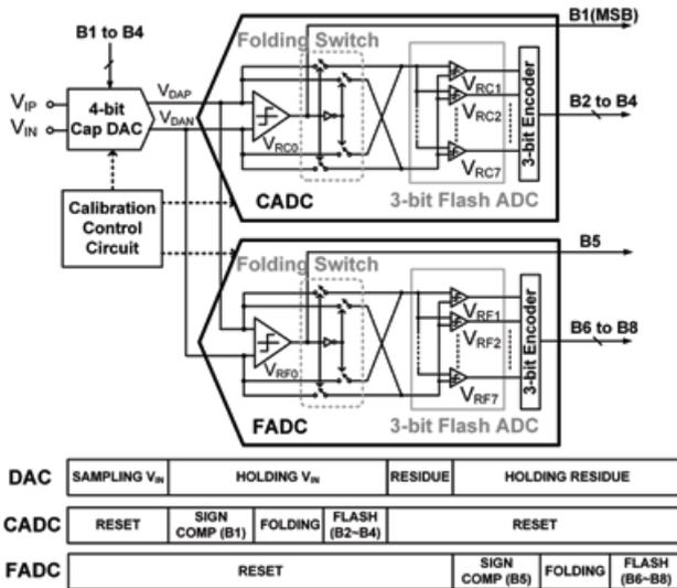
Fig. 1. Proposed ADC circuit diagram.
