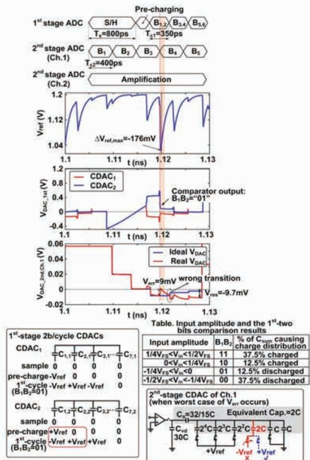
Fig. 2. The worst case of reference ripples in the PI PS ADC.
