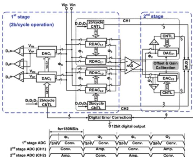
Fig. 1. PI Pipelined-SAR ADC architecture and timing diagram.
