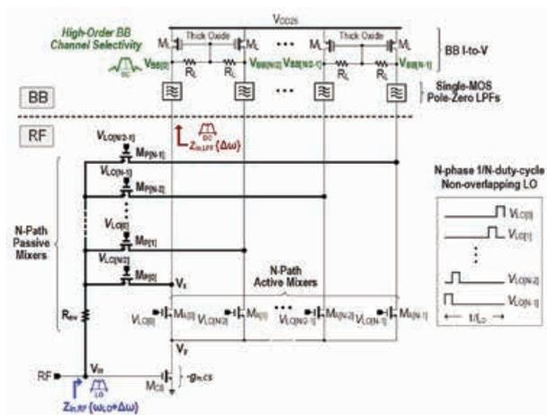
Fig. 1. Proposed RF-to-BB-current-reuse wideband receiver with the N-path filtering technique.
