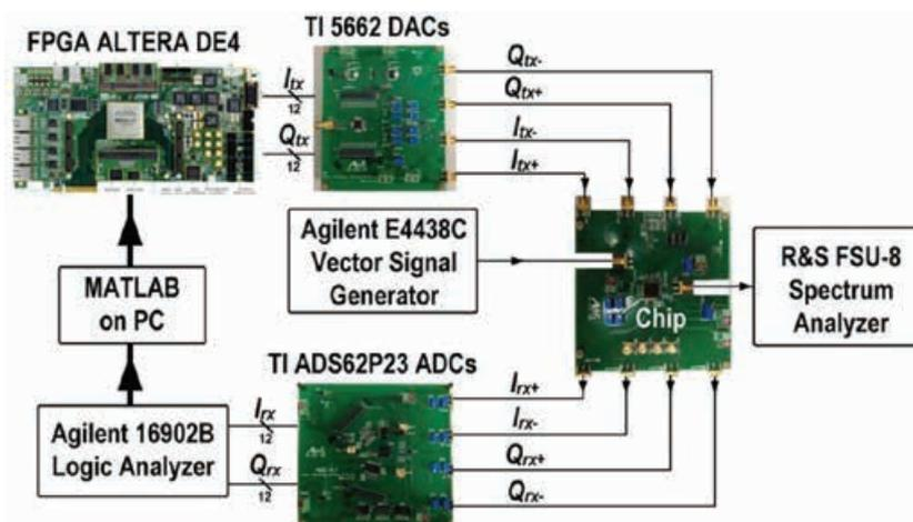
Fig. 2. Measurement setup.
