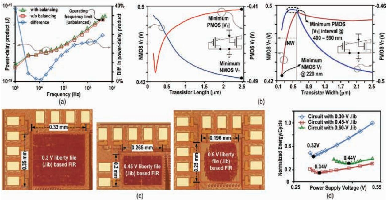
Fig. 1. (a) PDP of an inverter (FO4 loading) with balanced (P/N ratio = 5/1) and unbalanced (P/N ratio = 2/1) PU/PD network vs. operating frequency at 0.3 V. (b) NMOS/PMOS  $V_t$  vs. transistor length (RSC) (left) and transistor width (INW) (right) at  $V_{DD} = 0.3$  V. (c) Die micrographs. (d) Normalized energy/cycle at different supplies.
