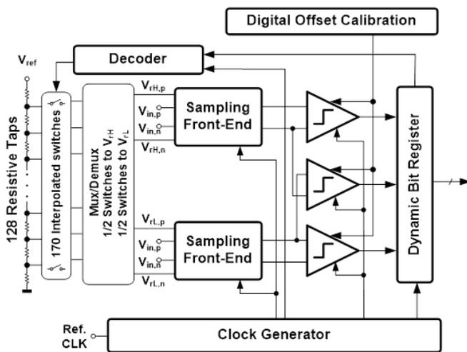
Fig. 1. ADC architecture.
