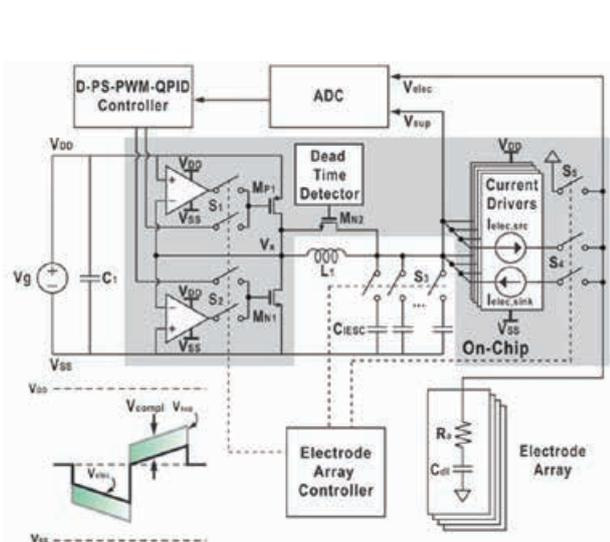
Fig. 1. Block diagram and of the proposed power-supply modulated micro-stimulator system and its output waveform during a biphasic stimulation cycle.
