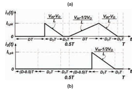
Fig. 3. Output side small signal model of the 3LB converter for DCM: (a) Output side of the 3LB converter DCM small signal model and (b) Output side current waveforms,  $i_1(t)$ :  $0 < D < 0.5$ ,  $i_2(t)$ :  $0.5 < D < 1$ .
