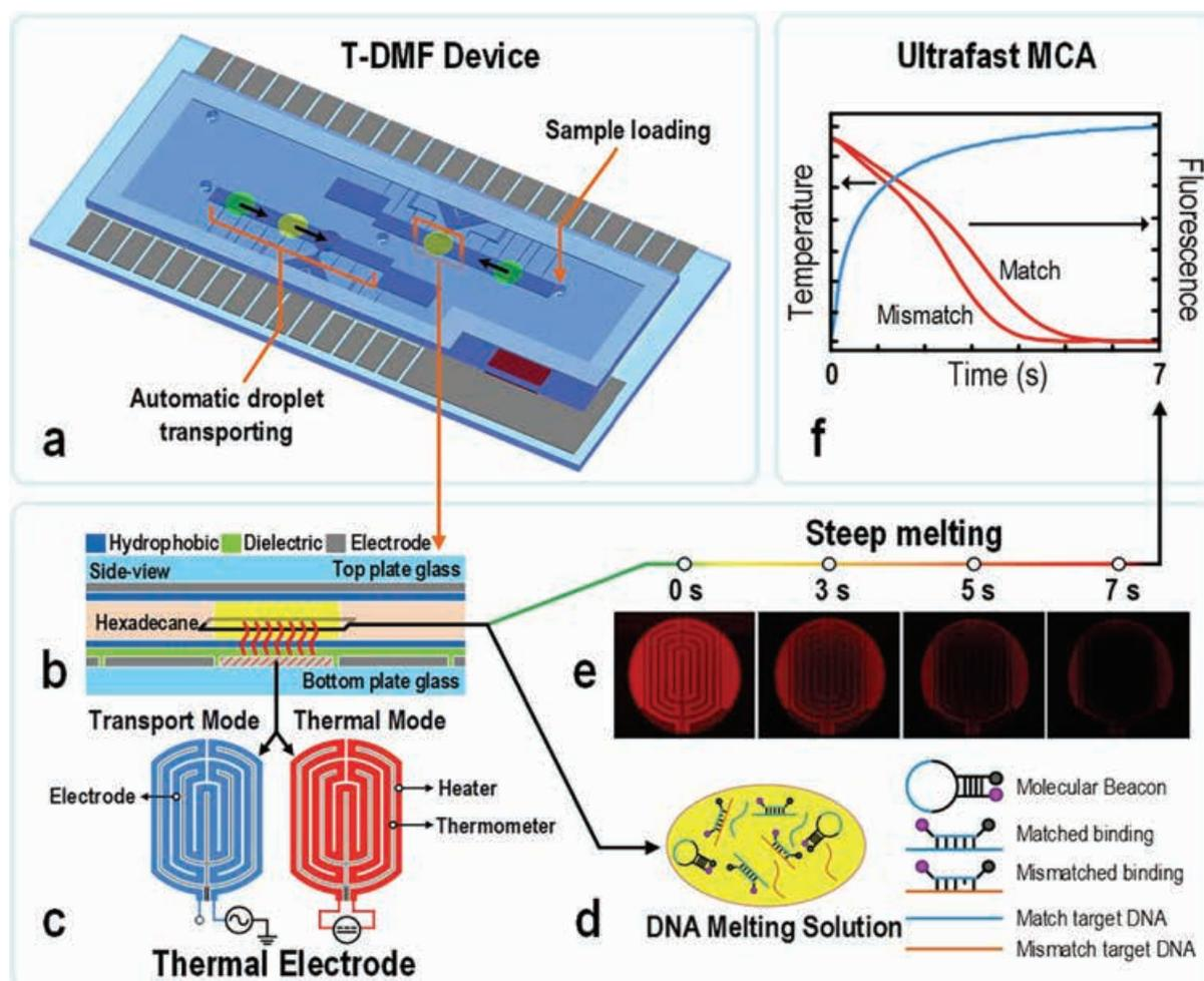
Fig. 1. Thermal digital microfluidic (T-DMF) device for ultrafast DNA melting curve analysis (MCA).
