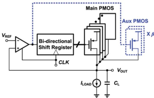
Fig. 1. Implementation of the modified D-LDO with LCO reduction.
