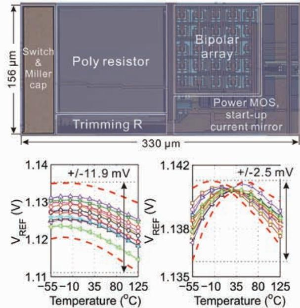
Fig. 2. Chip micrograph (top). Inaccuracy of  $V_{REF}$  from 12 samples without trimming (bottom left) and after batch trimming  $R_{c1}$  at 25  $^{\circ}\text{C}$  (bottom right).
