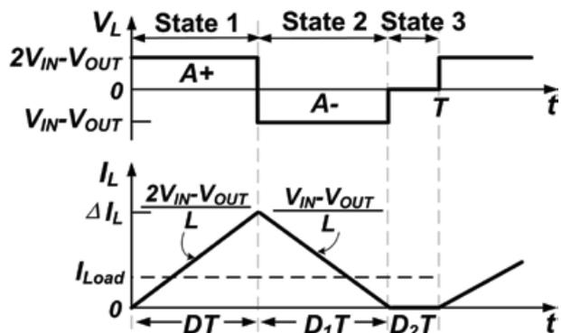
Fig. 2. KY converter idealized  $V_L$  and  $I_L$  waveforms for DCM.
