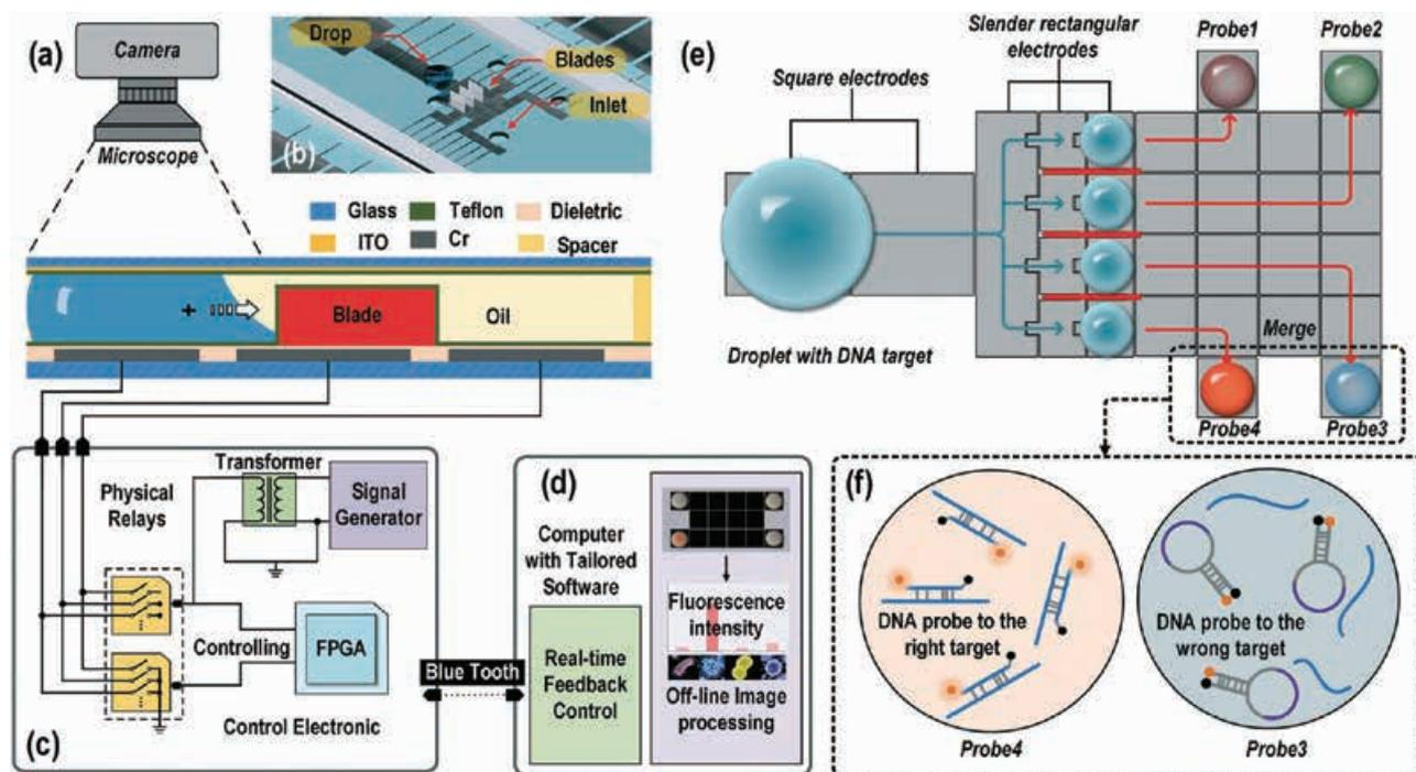
Fig. 1. Thermal digital microfluidic (T-DMF) device for ultrafast DNA melting curve analysis (MCA).
