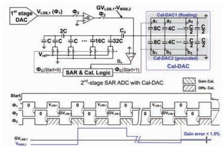
Fig. 2. Circuit implementation of the BSGC technique and its control timing diagram (Only Channel 1 shown).
