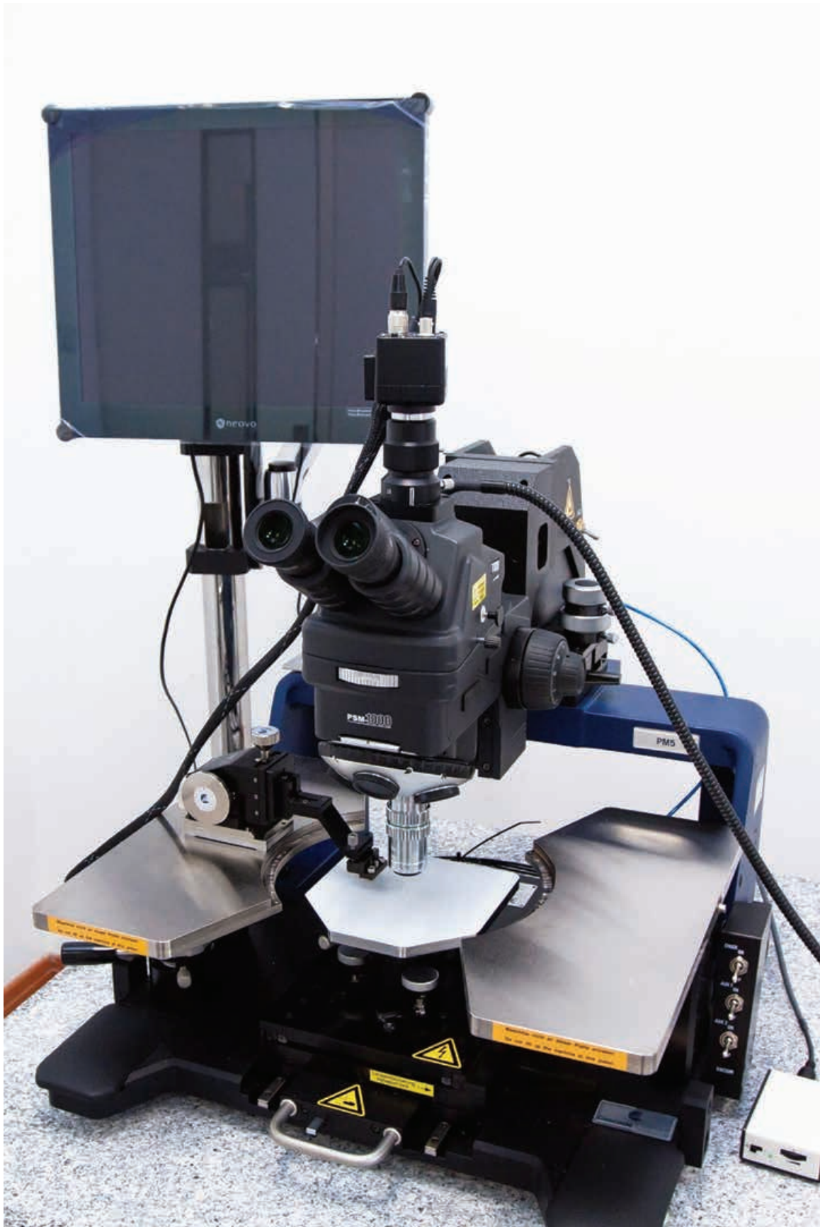
Cascade PM5 Manual Analytical Probe Station/Base Machine and with SGS and SGSGS probes up to 65GHz
