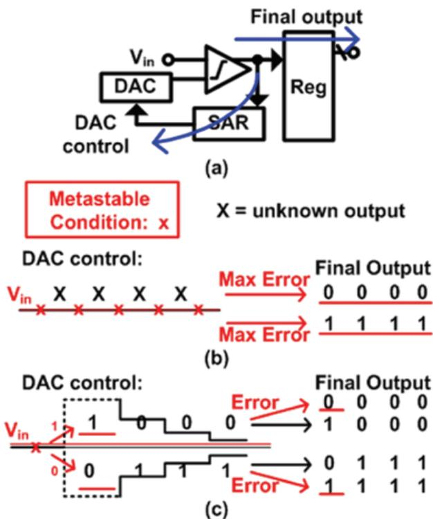
Fig. 1. (a) Conventional SAR block diagram (b,c) metastable error characteristics in the SAR ADC.
