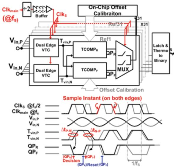
Fig. 1. Proposed ADC architecture and timing diagrams.
