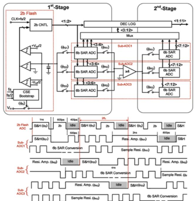
Fig. 2. Main channel ADC architecture and its timing diagram.
