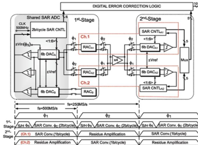
Fig. 1. Overall ADC architecture and its timing diagram.
