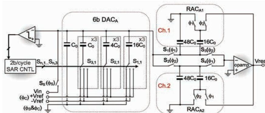
Fig. 2. 1st-stage 6b SAR ADC w/ Opamp-shared TI-Residue Amplification.
