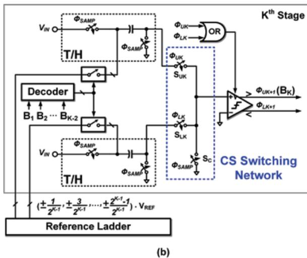
Fig. 1. Scheme of Kth stage of the proposed binary-search ADC.
