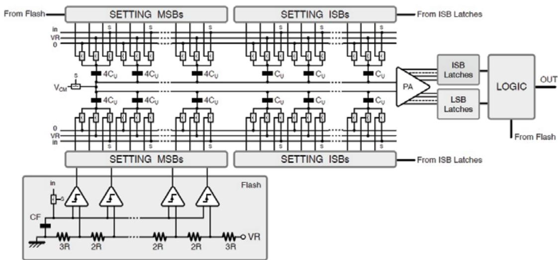
Fig. 1. ADC architecture
