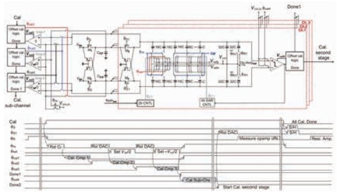
Fig. 2. Detailed circuit implementation of the first stage and offset calibrations for two stages together with its control timing diagram.
