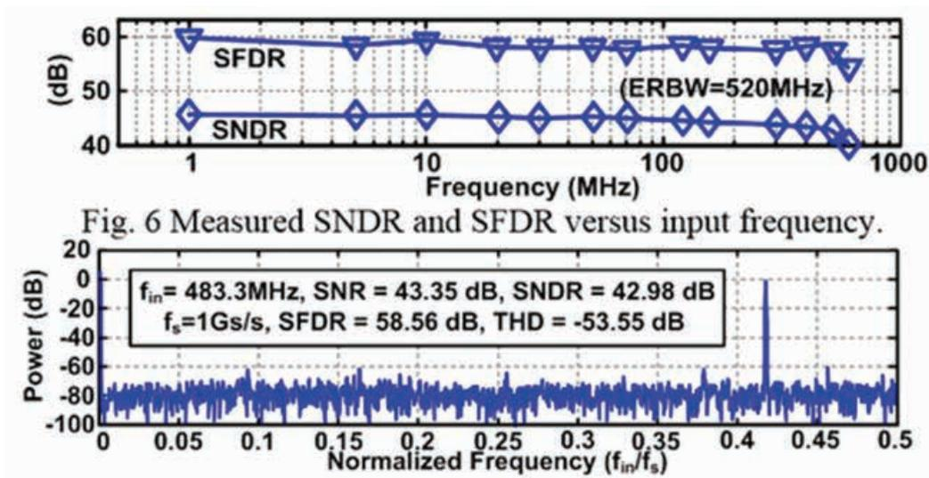
Fig. 2. Spectrum at 1GS/s and Nyquist input (decimated 125x).
