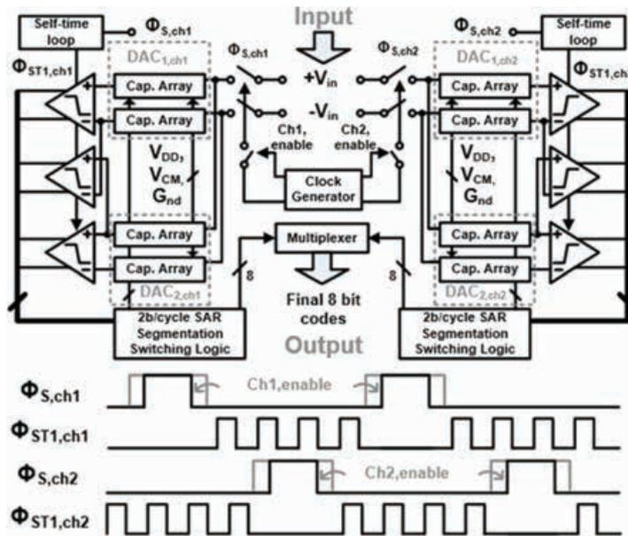
Fig. 1. Overall ADC architecture and its timing diagram.
