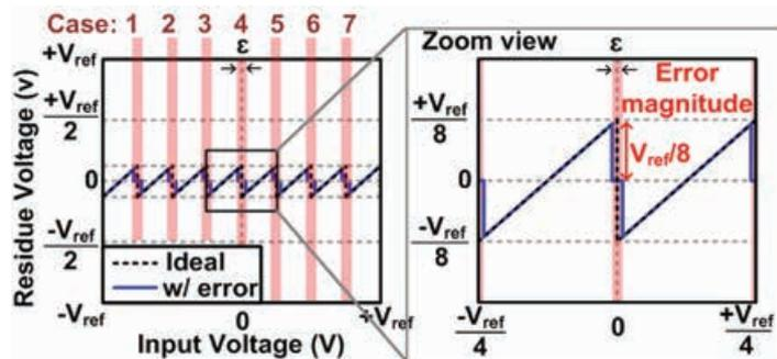
Fig. 2. Ideal and error (dot line) residue transfer curves of 6 bits 3b/cycle SAR with non-differential controls of the DACs in the red regions.
