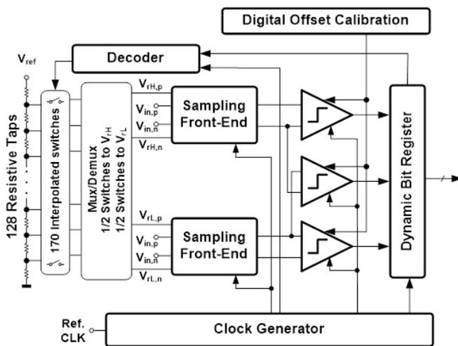
Fig. 1. ADC architecture.
