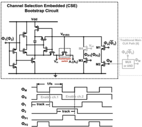
Fig. 1. Proposed Channel-Selection-Embedded bootstrap circuit and its control timing diagram.
