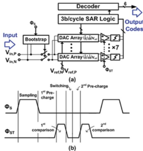
Fig. 1. The ADC (a) architecture and (b) timing diagram with time allocation.
