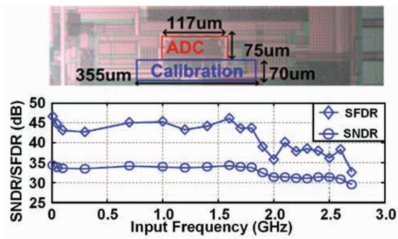
Fig. 1. The ADC architecture, the Chip Photograph and Dynamic Performance.
