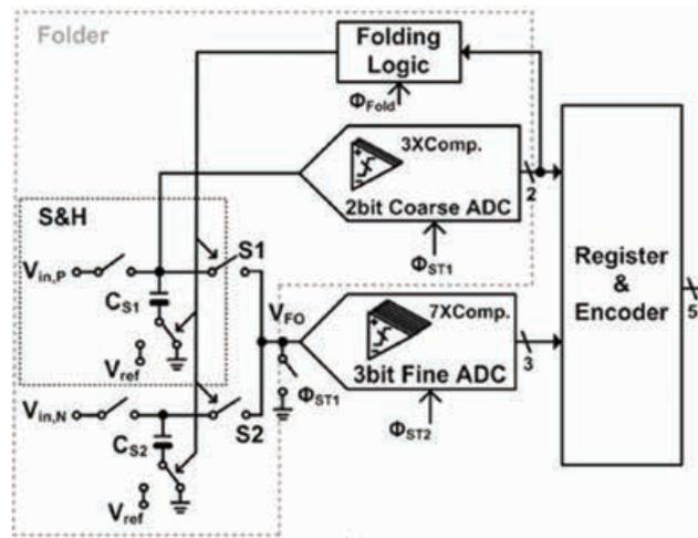
Fig. 1. ADC Architecture (actual implementation is in differential).
