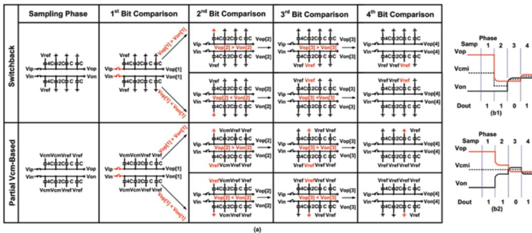
Fig. 2. (a) 4-b example of switchback and partial  $V_{cm}$ -based switching procedures. (b1) Comparator input common mode variation for switchback switching. (b2) Comparator input common mode variation for the proposed switching.
