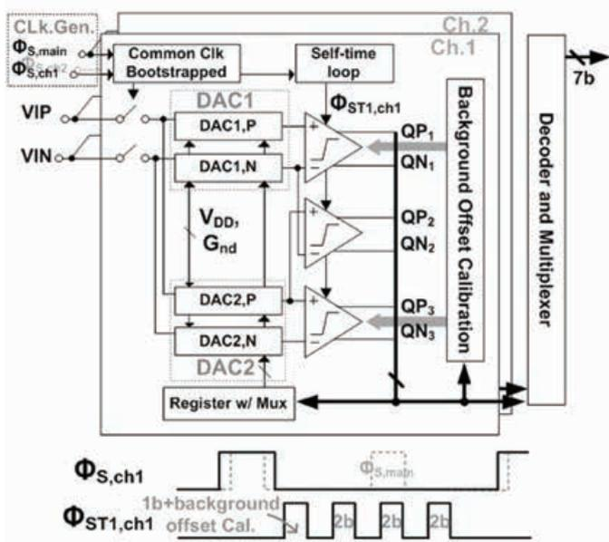
Fig. 1. Overall 2x interleaved 1-then-2bit/cycle SAR ADC architecture.
