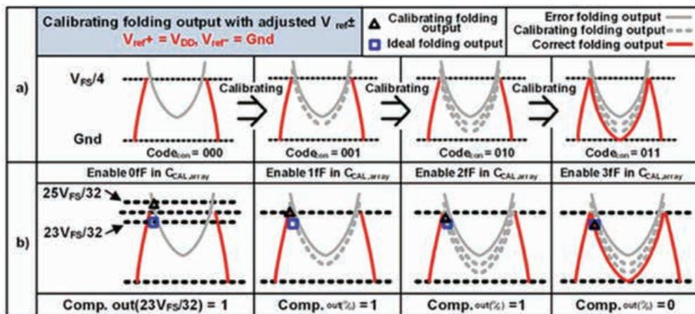
Fig. 2. Folding-reference calibration scheme and its signals behavior.
